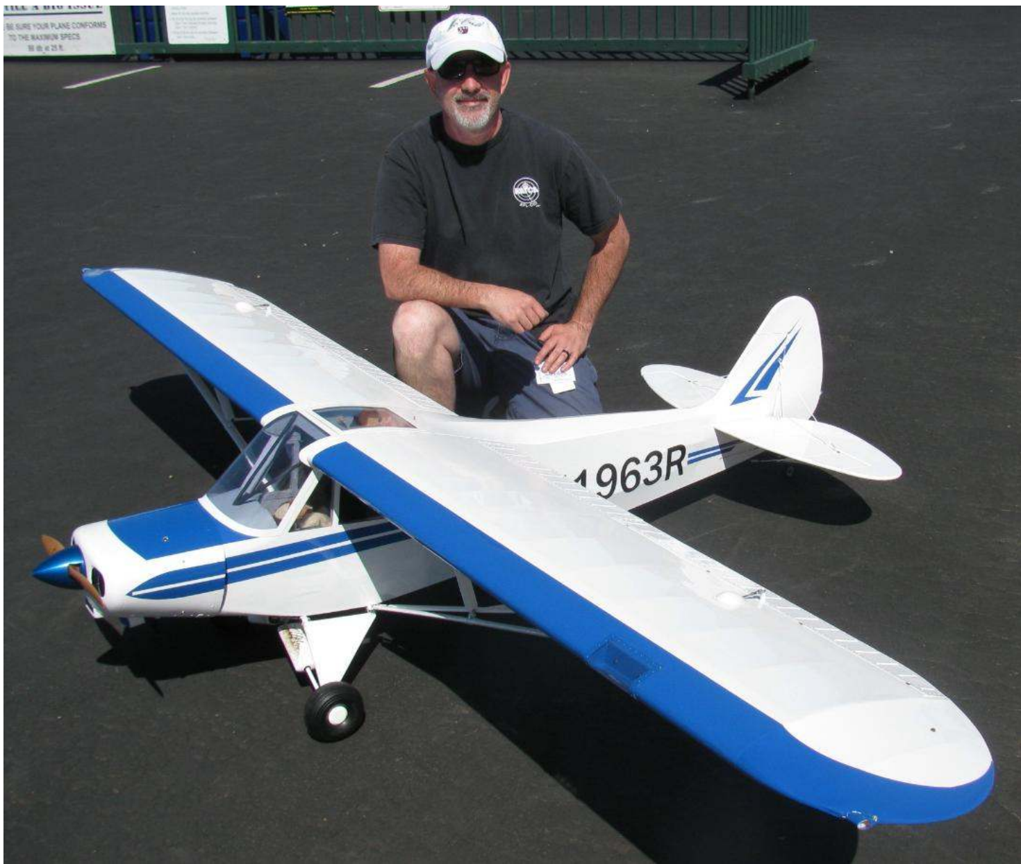
Jared Gregg flies his new Cub from Hangar 9. The wingspan is 108 in. It is powered by an Evolution 33cc gas engine running a 17 x 8 prop. It weighs 16 lbs.
