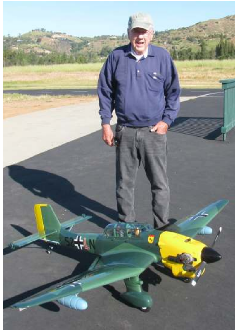
Bill DeMore has maidenied his new German Stuka warbird ARF from Phoenix Models. The wingspan is 74 in. It is powered by an OS-120-AX glow engine with a Bisson Pitts muffler.
