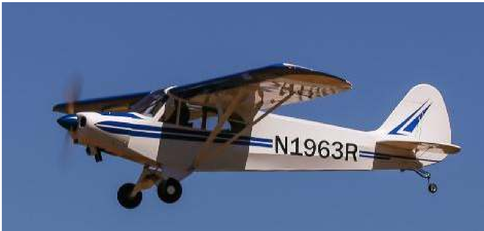
Jared Gregg flies his new Cub from Hangar 9. The wingspan is 108 in. It is powered by an Evolution 33cc gas engine running a 17 x 8 prop. It weighs 16 lbs.
