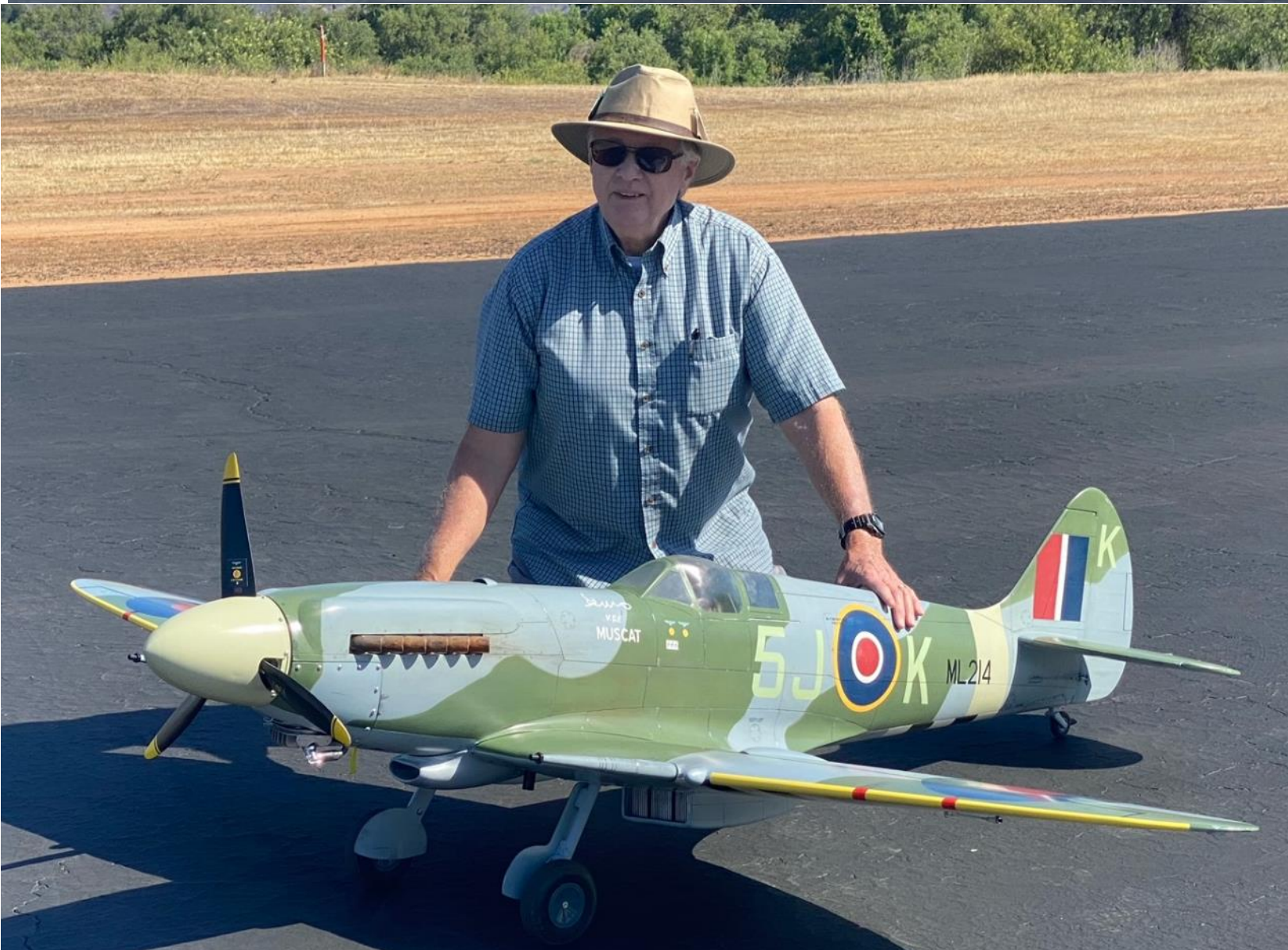
YELLOW Aircraft Spitfire with 55cc DLE with canister exhaust- Painted and weathered with Callie Graphics. As always, John Cutler did an outstanding job. (Chris Thompson photos)
