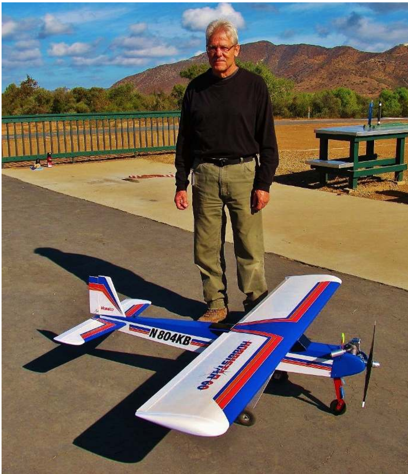
Larry Stainbrook is flying this Hobby Star 60 from Hobbico. It has a wingspan of 72 in. It is powered by a Saito 91 four-stroke glow engine running @ 14 x 6 prop. It weighs 7 lbs. 4 oz. The nose gear has a spring installed for softer landing of tri-gear. The fuselage has been cut just behind the wing so it can be unbolted and separated for transporting.
