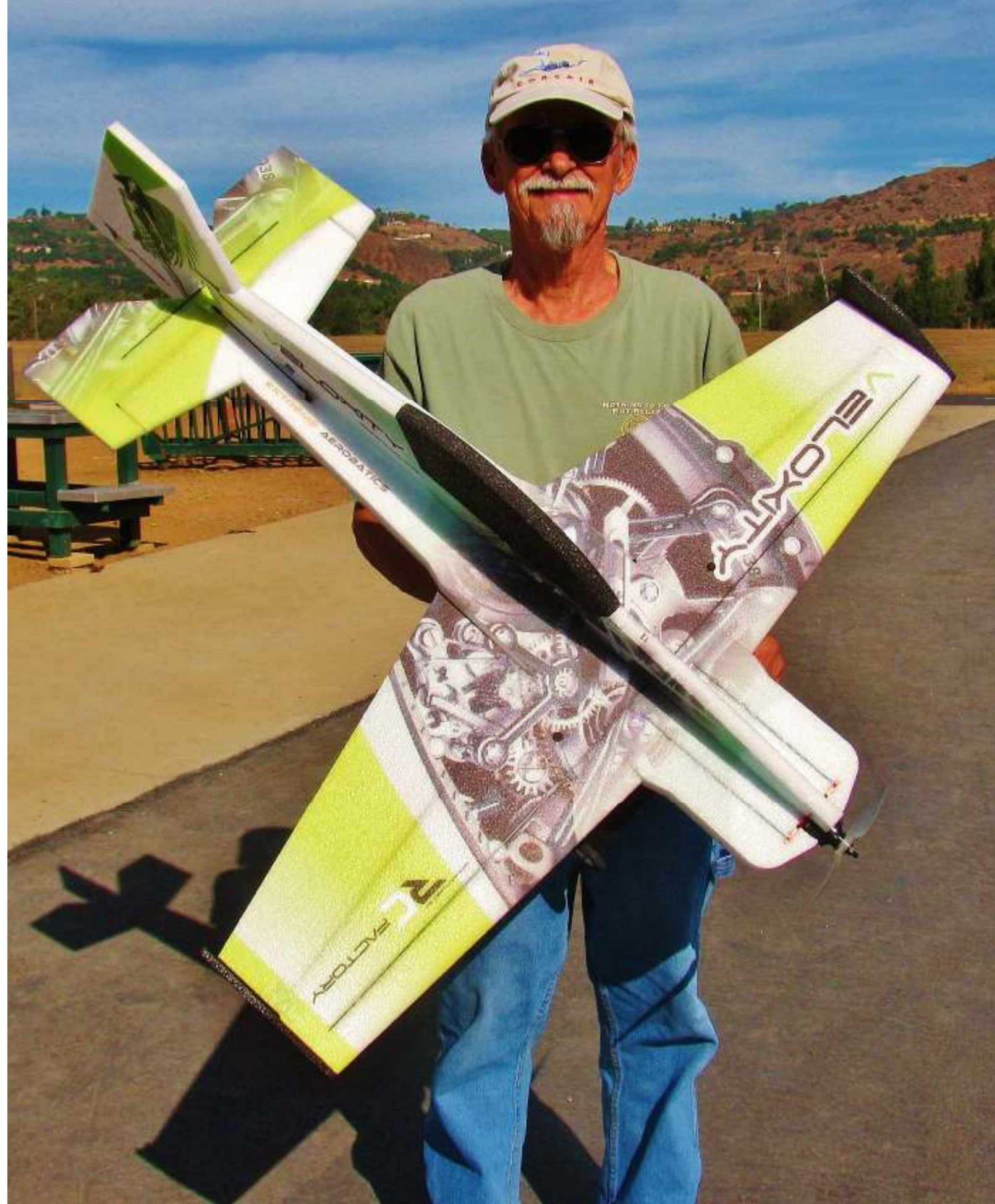
Larry Hufford had a maiden flight with his new Velocity electric ARF from Twisted Hobbies. The wingspan is 44 in. It has a 2814 --100 electric motor, 45 amp ESC, and a 3S battery 2200 mAh.
