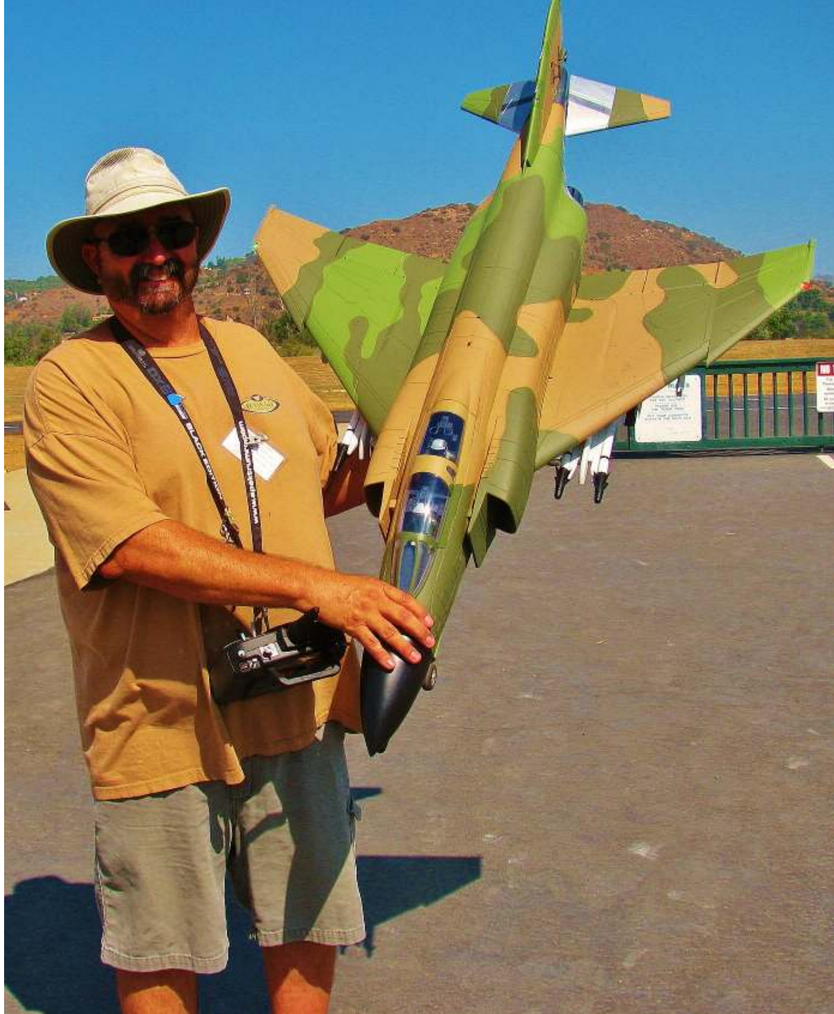
Chris Thompson is flying this F-4 Phantom Jet ARF with electric ducted fan. It has tri-electric retracts and LED lights.
