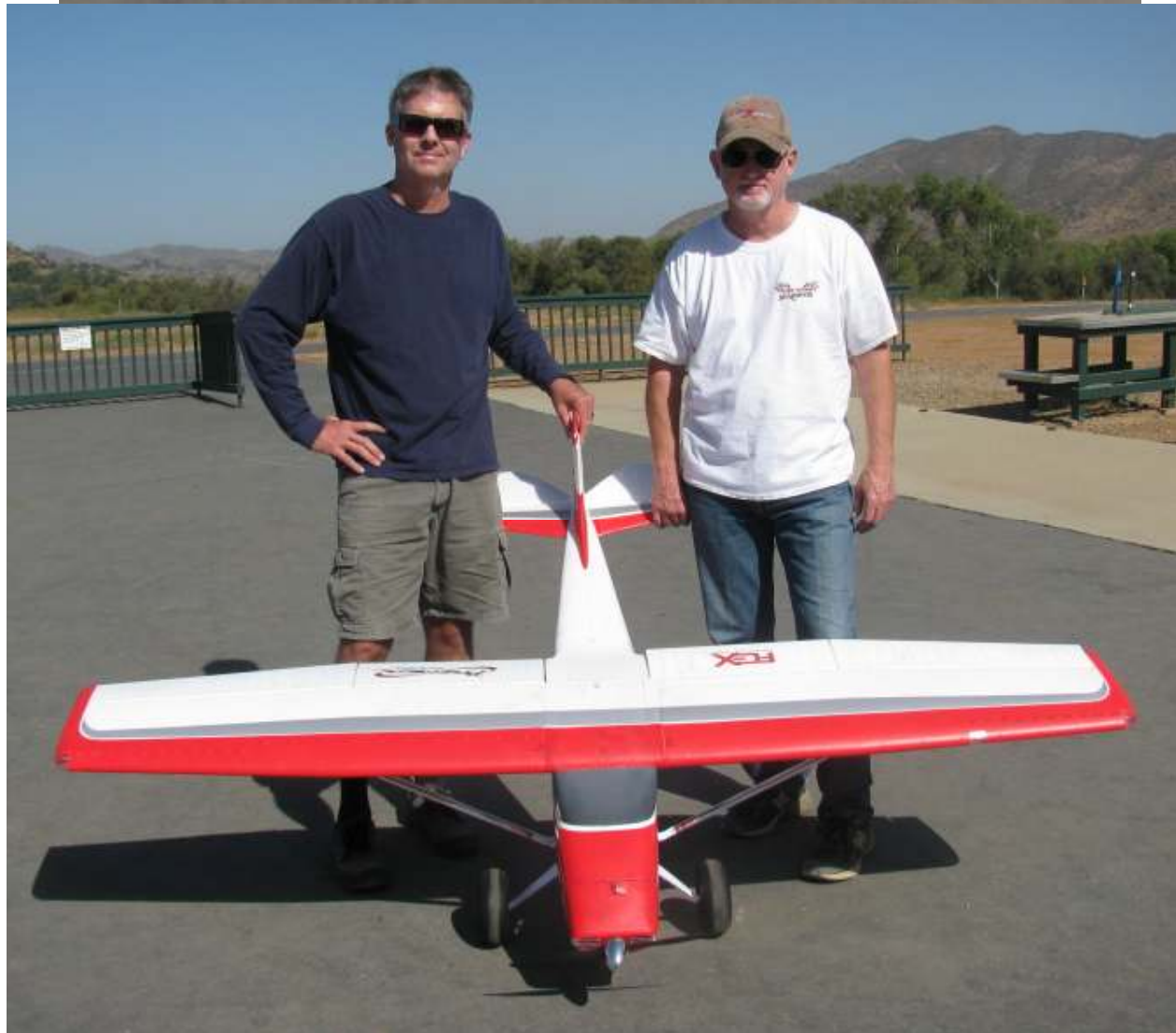
Here are co-partners James D'Eliseo and Dave Litaker with their new Cessna 170 Super STOL from Flex Innovations. This Night Version has factory installed array of LED lights that fully illuminate plane and the floats they also use with it. Tundra landing gear is being used here and a glider towing mechanism is also installed. The wingspan is 84 in. It is 3D capable and has a Potenza electric motor and servos with a 16 x 6 prop. It has full flaps / ailerons with flaps / and crow (all 3 options). It has HobbyWing 80A ESC and 6S 5000 mAh battery.
