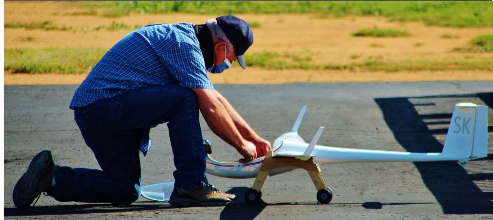
Steve's sailplane sits on a dolly which serves as the take-off gear which separates. The plane has its own power so can take off by itself if Steve wants. Or he can hand launch it.
