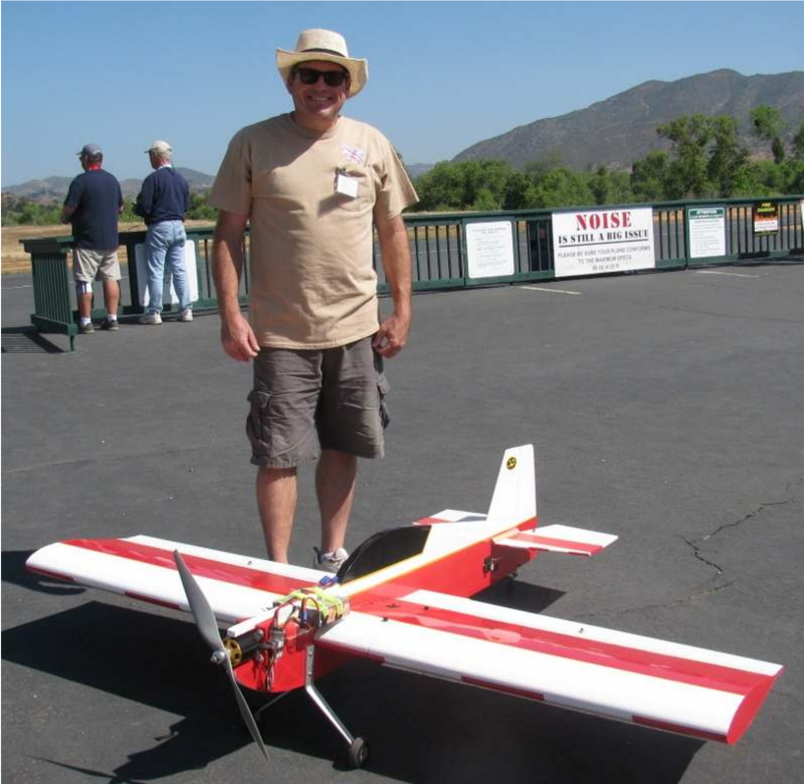
Here is our "Heli" Board Member, Chris Wilson flying an Aeroworks Profile plane with an 80 in. wing-span. This plane is not new and was given to him by a friend, so it was not his maiden flight. It has a Scorpion electric motor and two 6S batteries 3700 mAh.
