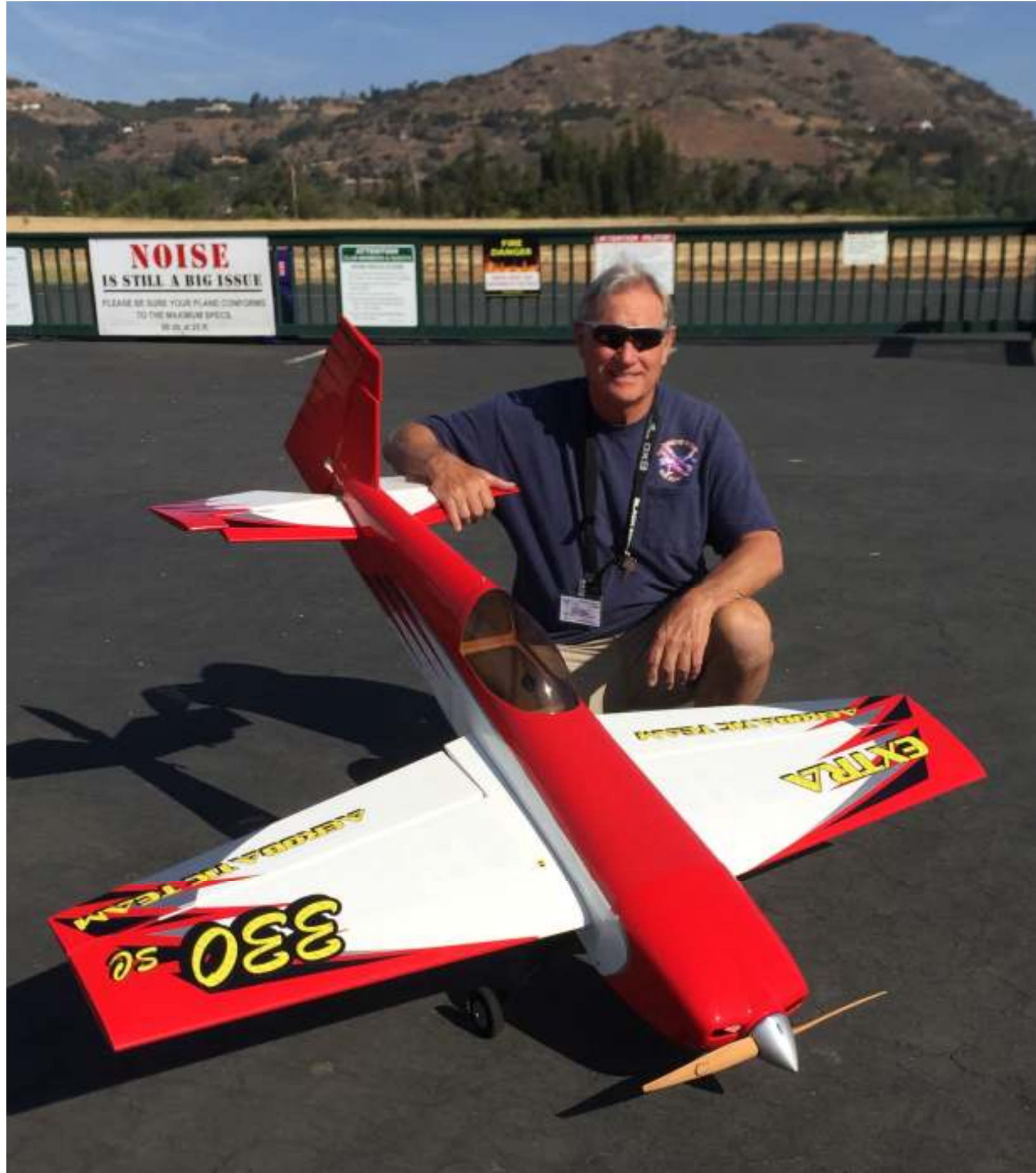
(Photo by Chris Thompson) of Mike Elrod making his maiden flight with this new Extra 330 from Hangar 9. The wingspan is 66 in. 56 It has a Hacker A50 electric motor, Talon 90 ESC, and 6S battery 5000 mAh.
