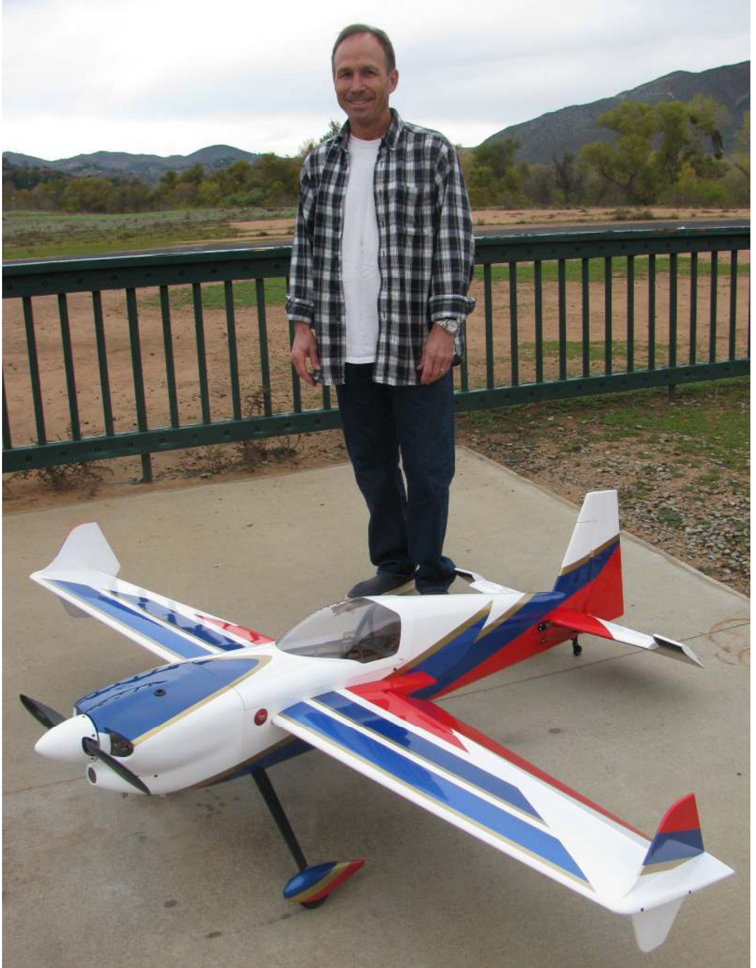
Ernie Leep has a new Edge from 3D Hobby Shop that was just maiden successfully. The wingspan is 75 in. and it weighs 10 lbs. 12 oz. with fuel. It is powered by a DA-35 gas engine running a 20 x 10 Falcon prop. It has HiTec 7955 servos.
