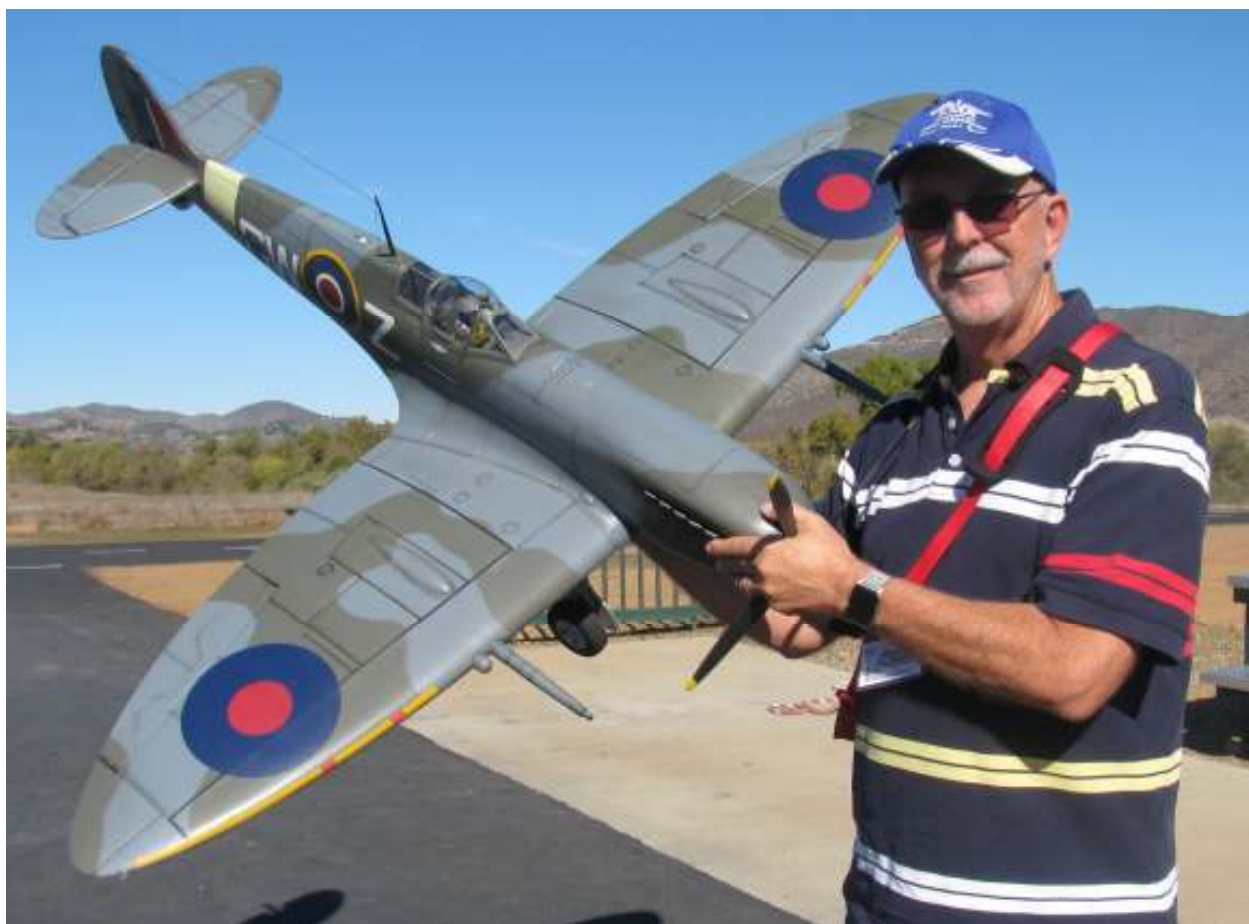
Steve Gebler is flying this new FlightLine Spitfire Mark IXC from Motion RC. A custom airbrush painting job was done by Chris Thompson for a realistic warbird look. The wingspan is 63 in. It has an electric motor 390 kv running a 4-blade prop, 80 amp speed controller, and 6S battery 4000 mAh. It has electric retracts and full lights.
