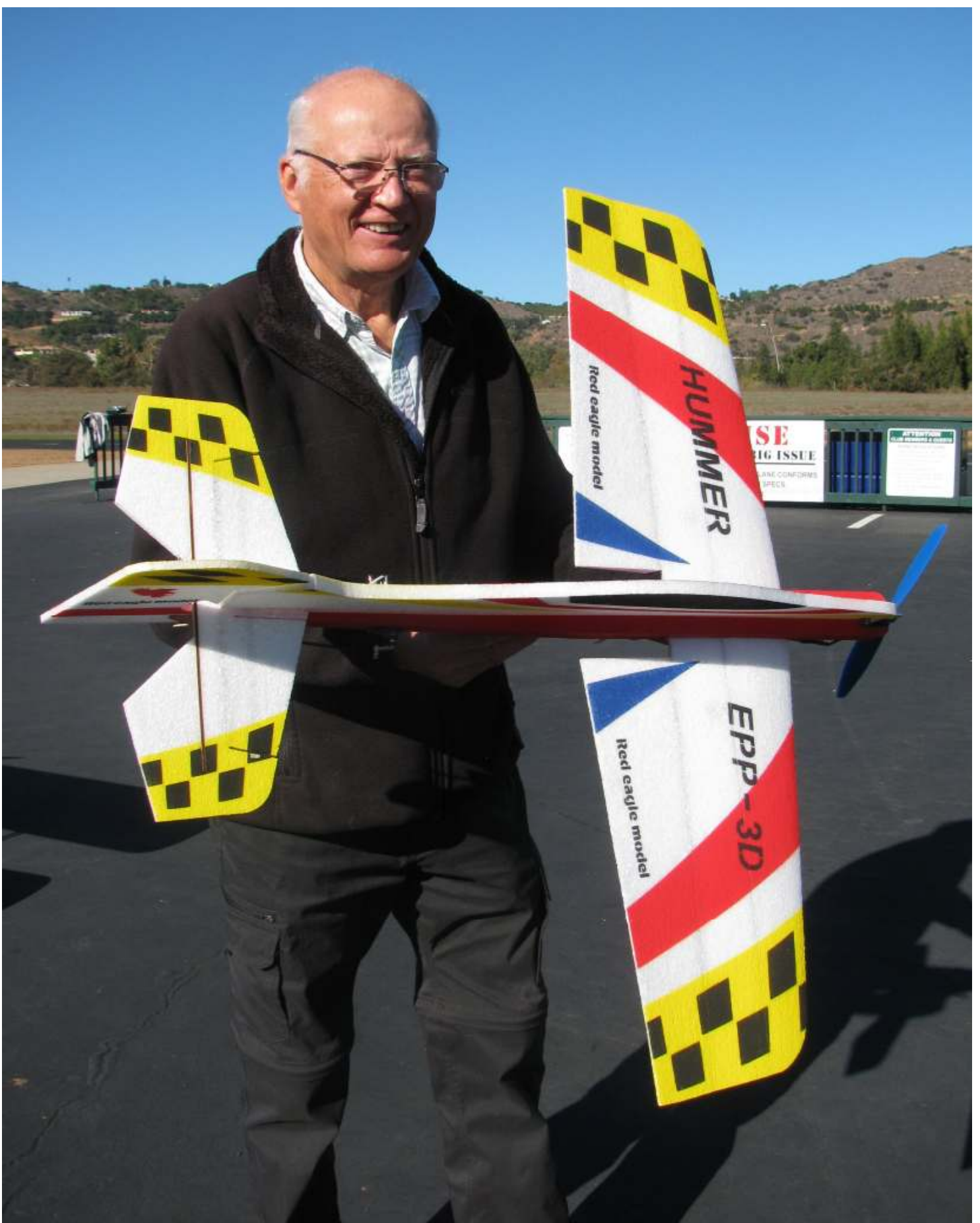
Graham Lloyd, 15 yr. flying member is back again from Great Britain. This is his new electric Hummer from Hobby King. It has a 40 amp ESC with a 1.8 battery. He bought it under $30.00 and the servos are low cost @ $2.00.
