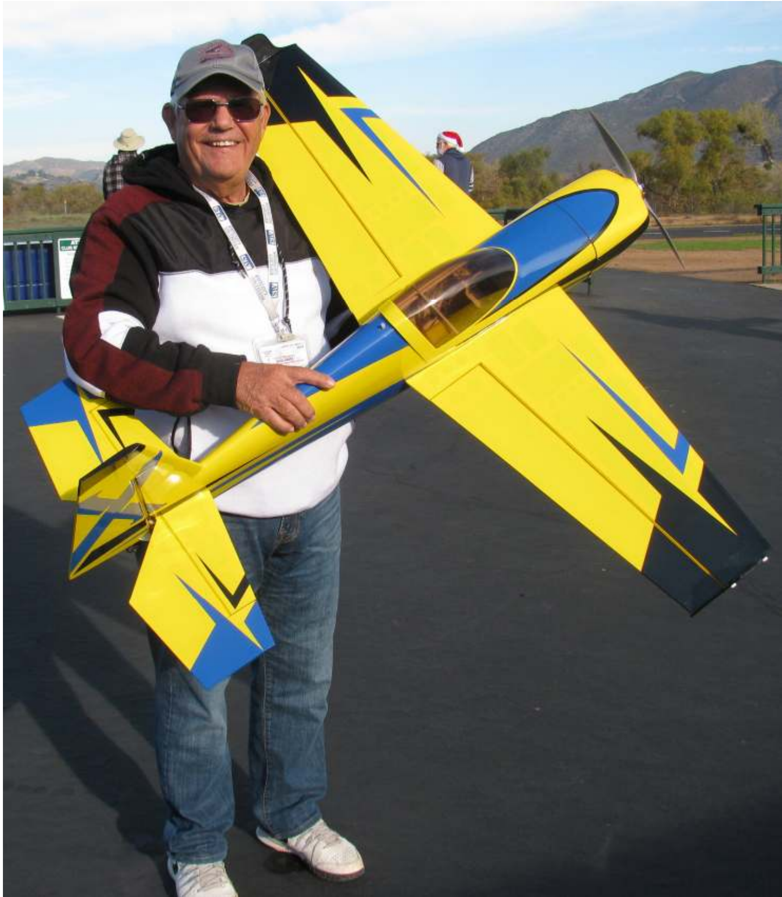
This is Don Davis flying his Slick 580 from Extreme Flight. The wingspan is 52 in. It has a T3910 electric motor with an Air Boss 80 amp ESC.
