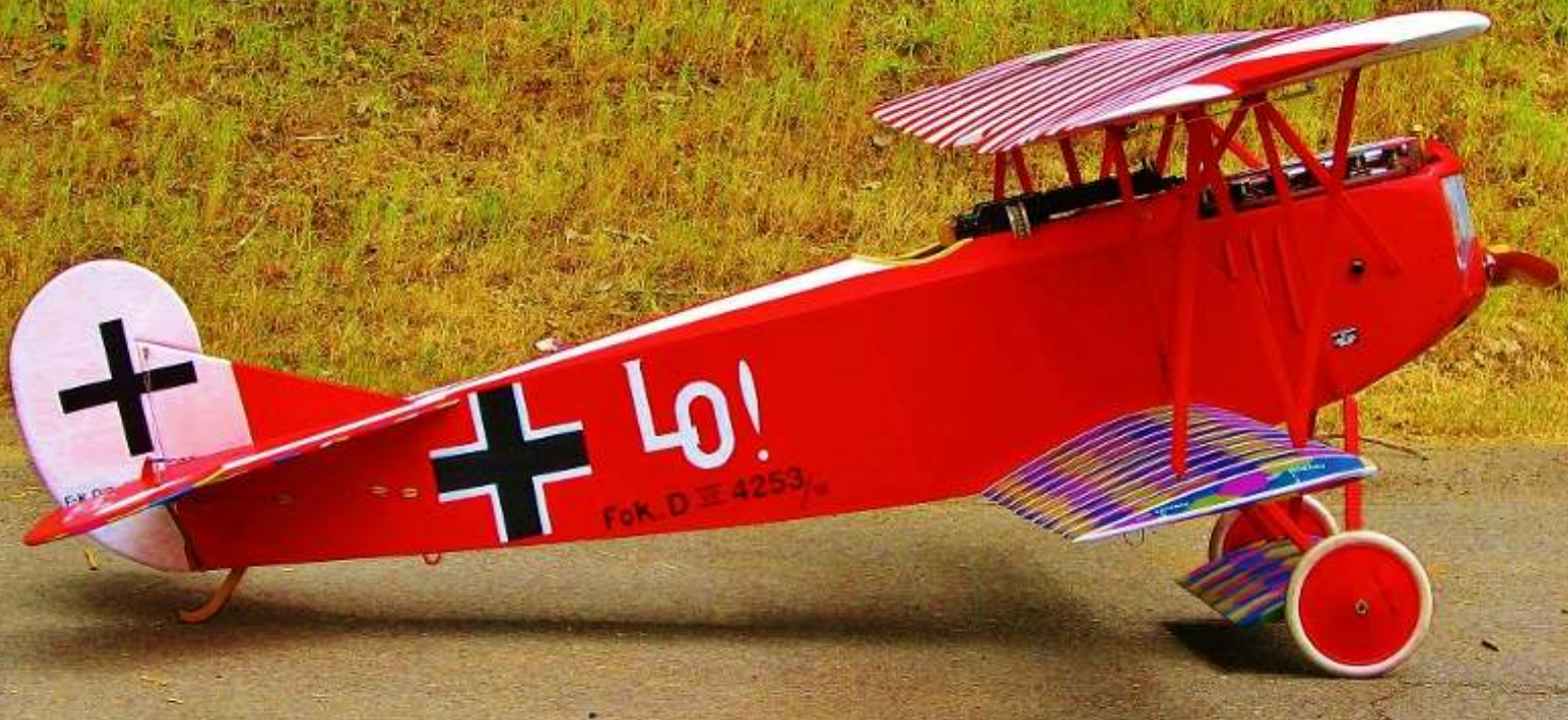
Your editor made this Balsa USA Fokker D-VII in the Von Richthofen Flying Circus colors. The Baron wanted you to see him coming. 'LO' are the first two letters of his girlfriend's name, Lola. This plane even has an engraved data plate, exposed engine, machine guns, complete cockpit, and a Fugli Imvac 34 cc 4 stroke gas engine.
