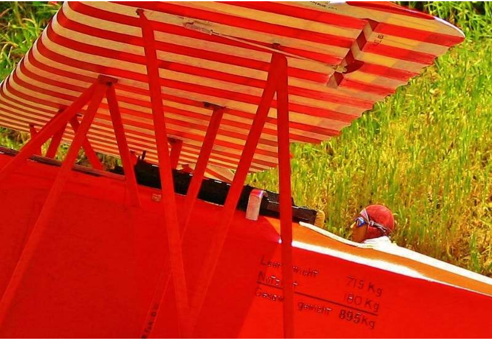
Your editor made this Balsa USA Fokker D-VII in the Von Richthofen Flying Circus colors. The Baron wanted you to see him coming. 'LO' are the first two letters of his girlfriend's name, Lola. This plane even has an engraved data plate, exposed engine, machine guns, complete cockpit, and a Fugli Imvac 34 cc 4 stroke gas engine.
