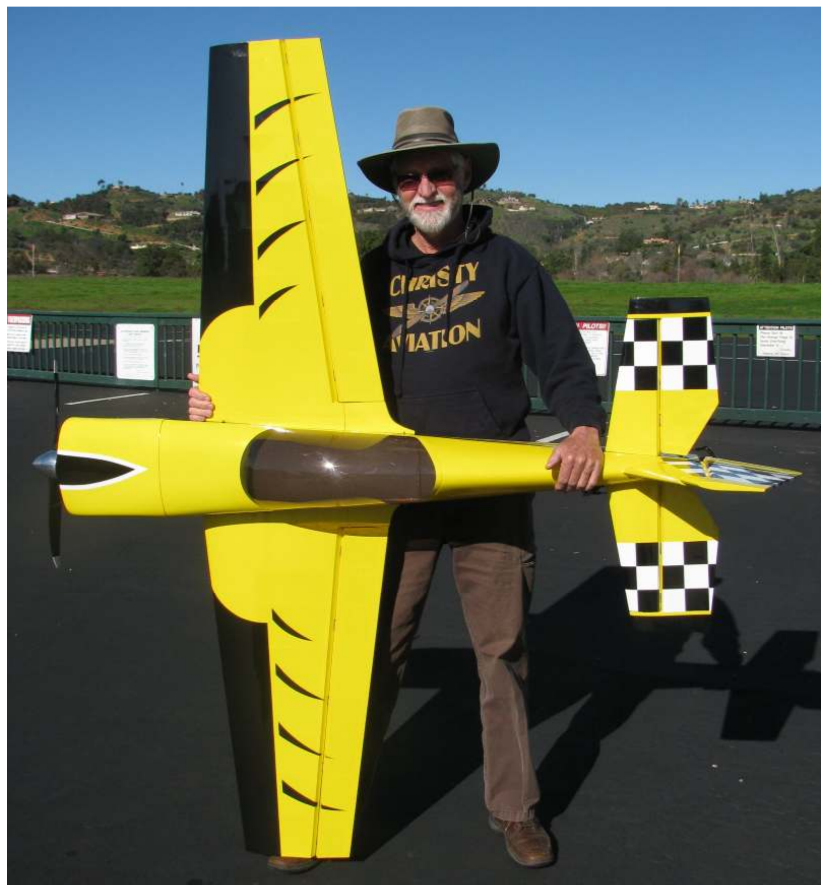
Jim Christy maidenied his new MX-2 from RC Jet World. Plane was manufactured by Fly-Model. The wing-span is 73 in. It is powered by a DLE-35 RA gas engine running a 19 x 8 prop. It has MKS 1230 servos and it weighs 11 lbs. 6 oz.
