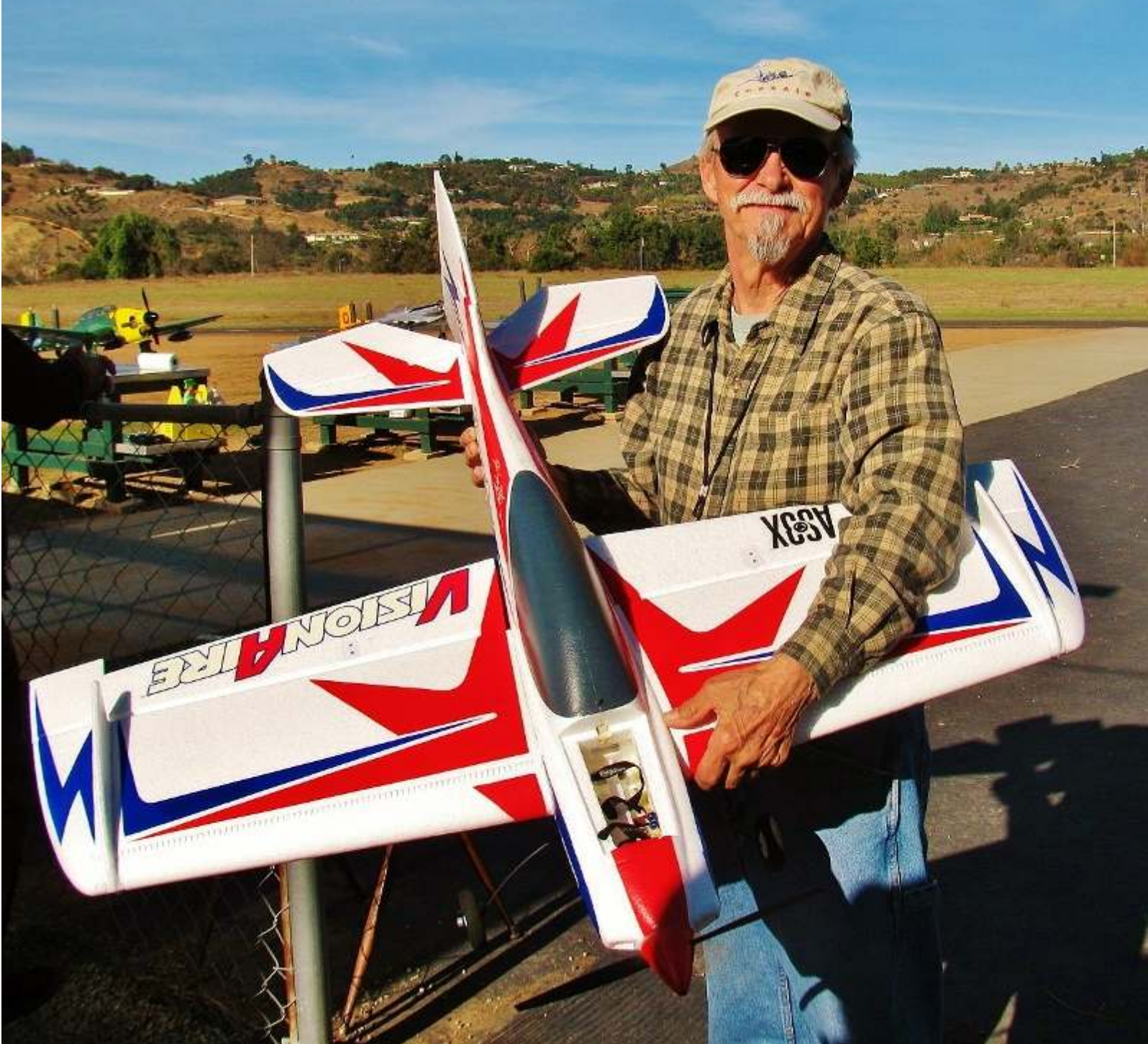
Larry Hufford is flying this new Vision Aire ARF from Park Zone. The wingspan is 45 in. and it has an AS-3X stabilizer flown with a Spektrum DX-18 radio. The electric motor is a BL-10 and is 1252v. The ESC is 40 amp and the 3S battery is 2200 mAh.
