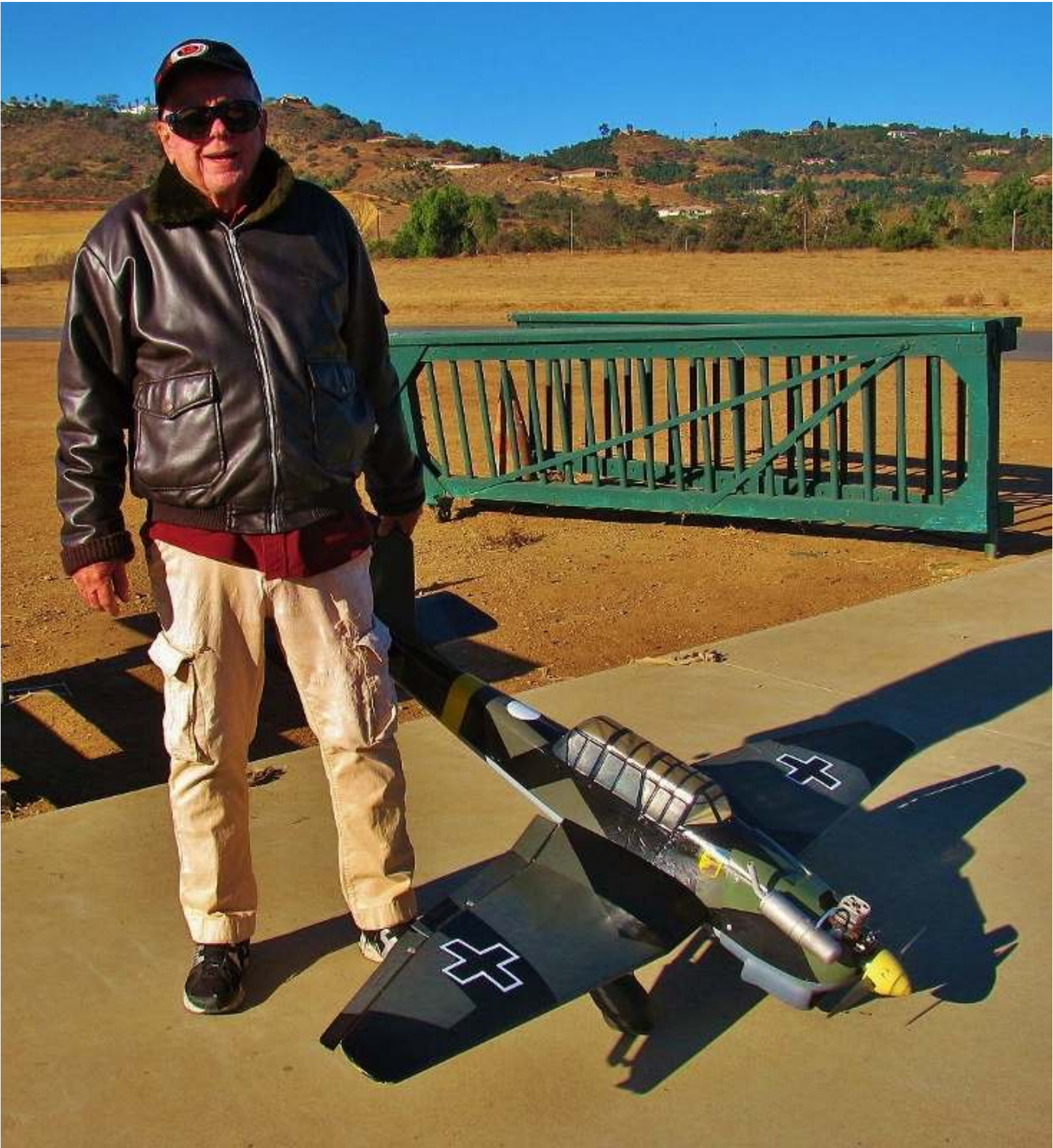
Bill DeMore has added to his warbird collection with this German Stuka divebomber. This ARF is now discontinued, but originally came from Great Planes, and he bought it from Roger Cosio. The wingspan is about 60 in. and it is powered by a 90 two-stroke glow engine.
