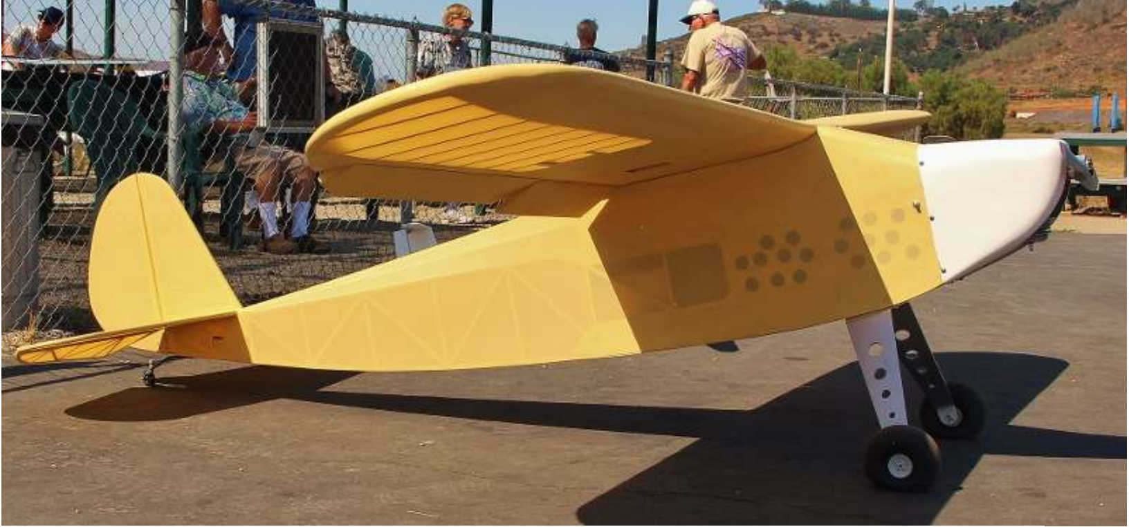
John Cutler is building this giant Cloud King for Tom Minegar for use as a tow plane. An 85cc gas engine powers it.
