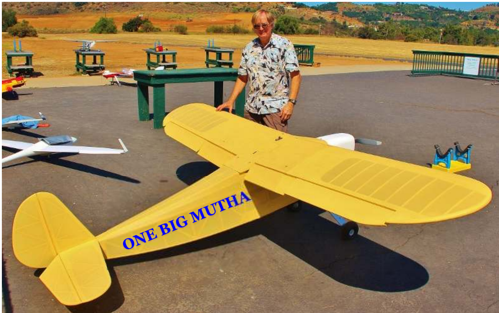
John Cutler is building this giant Cloud King for Tom Minegar for use as a tow plane. An 85cc gas engine powers it.
