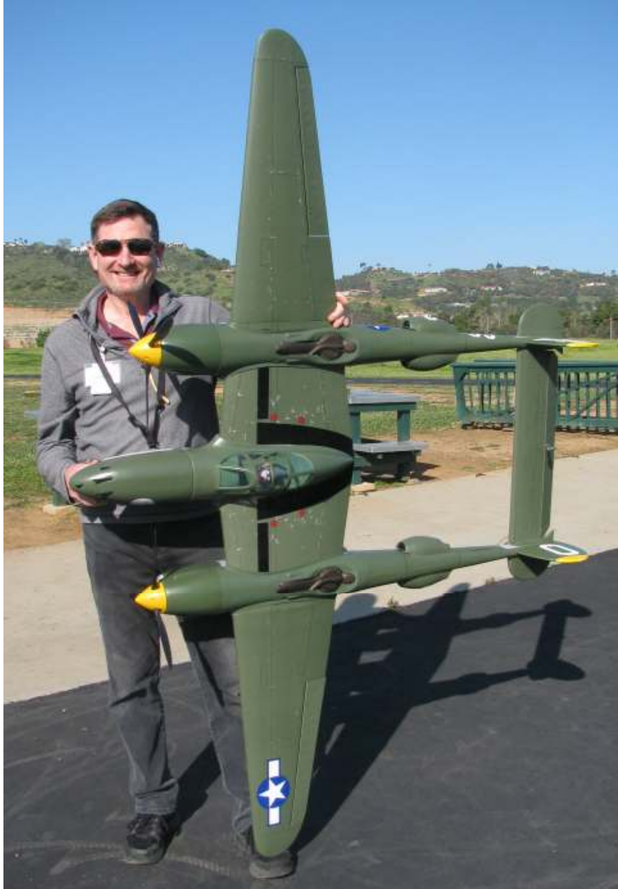
Dave Swaffer is flying his P-38 Lightning ARF from VQ. The wingspan is 83 in. and it weighs 26 lbs. The electric twin motors are Dualsky FM-5060 running both 16 Vario 3-blade props. The 2 speed controls are Castle Creations Phoenix Edge 100. Two 5S batteries are 5000 mAh. The tri-gear electric retracts are E-flite.
