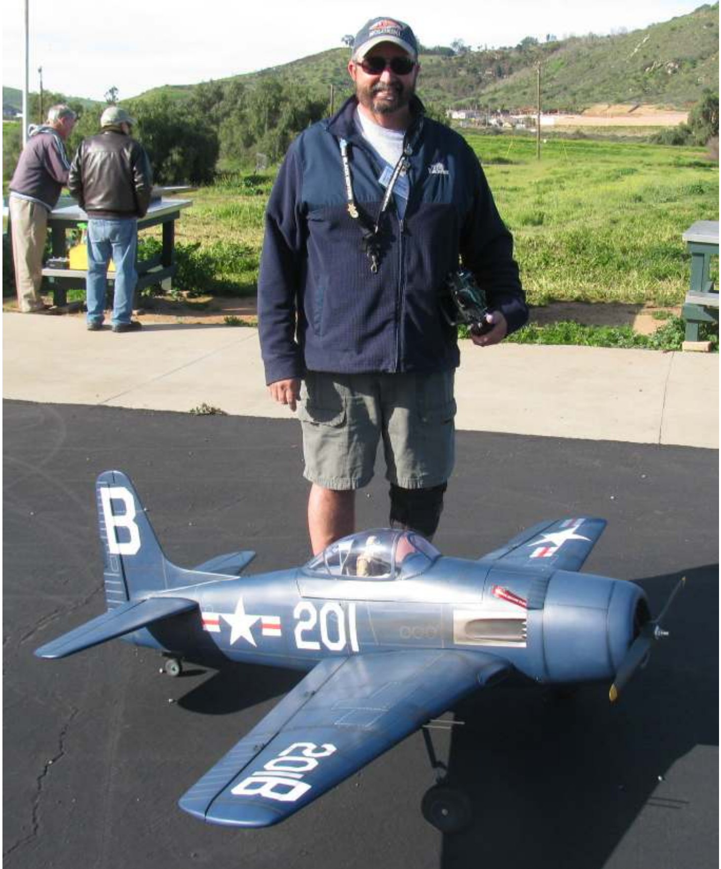
Chris Thompson has maiden and is flying this Bearcat ARF from VQ. The wingspan is 80 in. It has a Dualsky GA 6000.8 electric motor with two 6S batteries 5000 mAh. It has electric retracts, bomb release, and he has airbrushed the panel lines.
