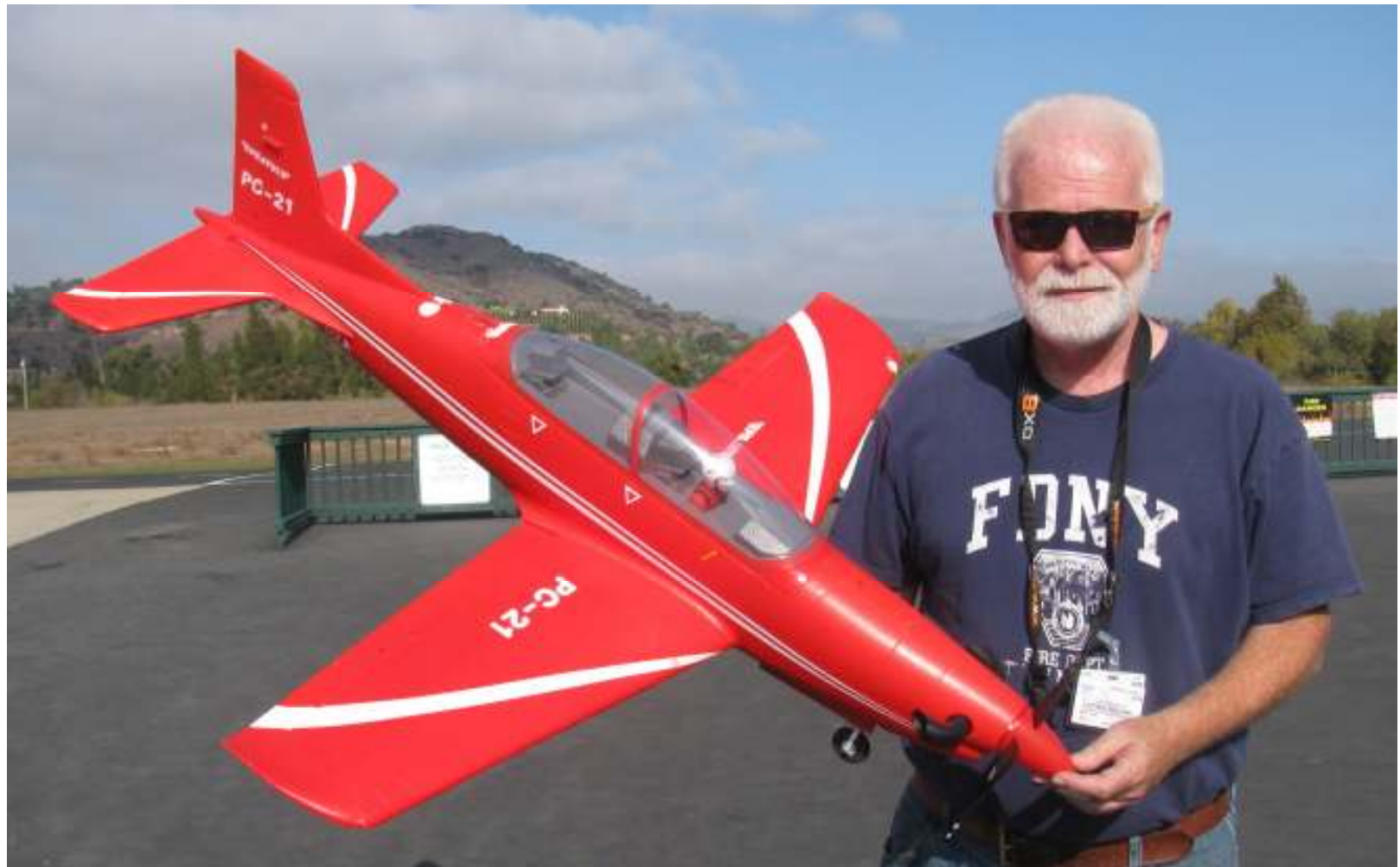
George Sullivan has a new PC-21 electric ARF from FMS. It has a 4S battery 5000 mAh.
