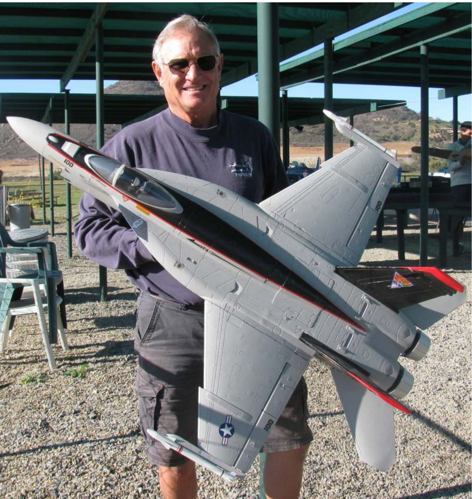
Mike Elrod is flying this FA-18 Jet from Freewing. The wingspan is 38 in. It has a 90 mm electric ducted fan with vectored thrust. The ESC is 130 amp and the 6S battery is 5000 mAh.
