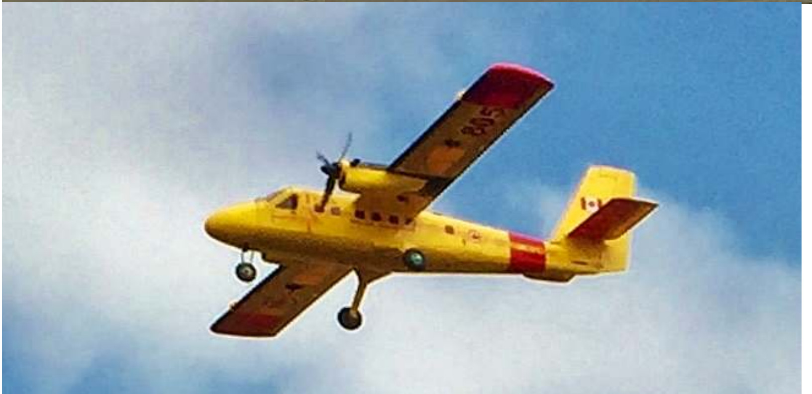
Jim Figgers VQ de Havilland Twin Otter. I've seen these flying on the Canadian Coast. They have fixed gear, STOL capabilities and carry 19 passengers.
