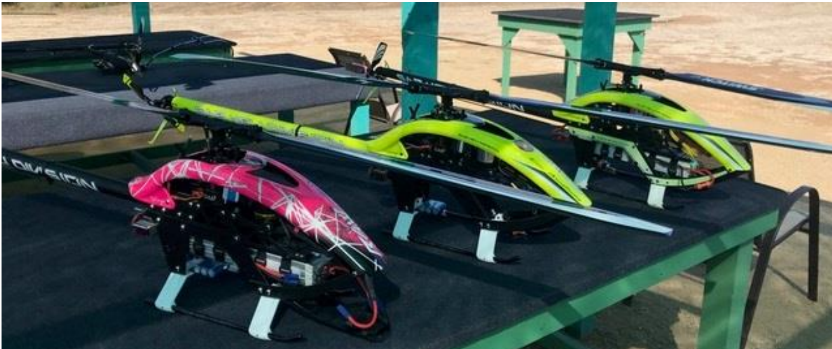
Eric Armstrong and Chris Wilson's SAB RAW Helicopters. These are the newest creations from SAB - the "Canopy" is bolted to the frame and does not need to be removed to install or remove batteries - very handy!
