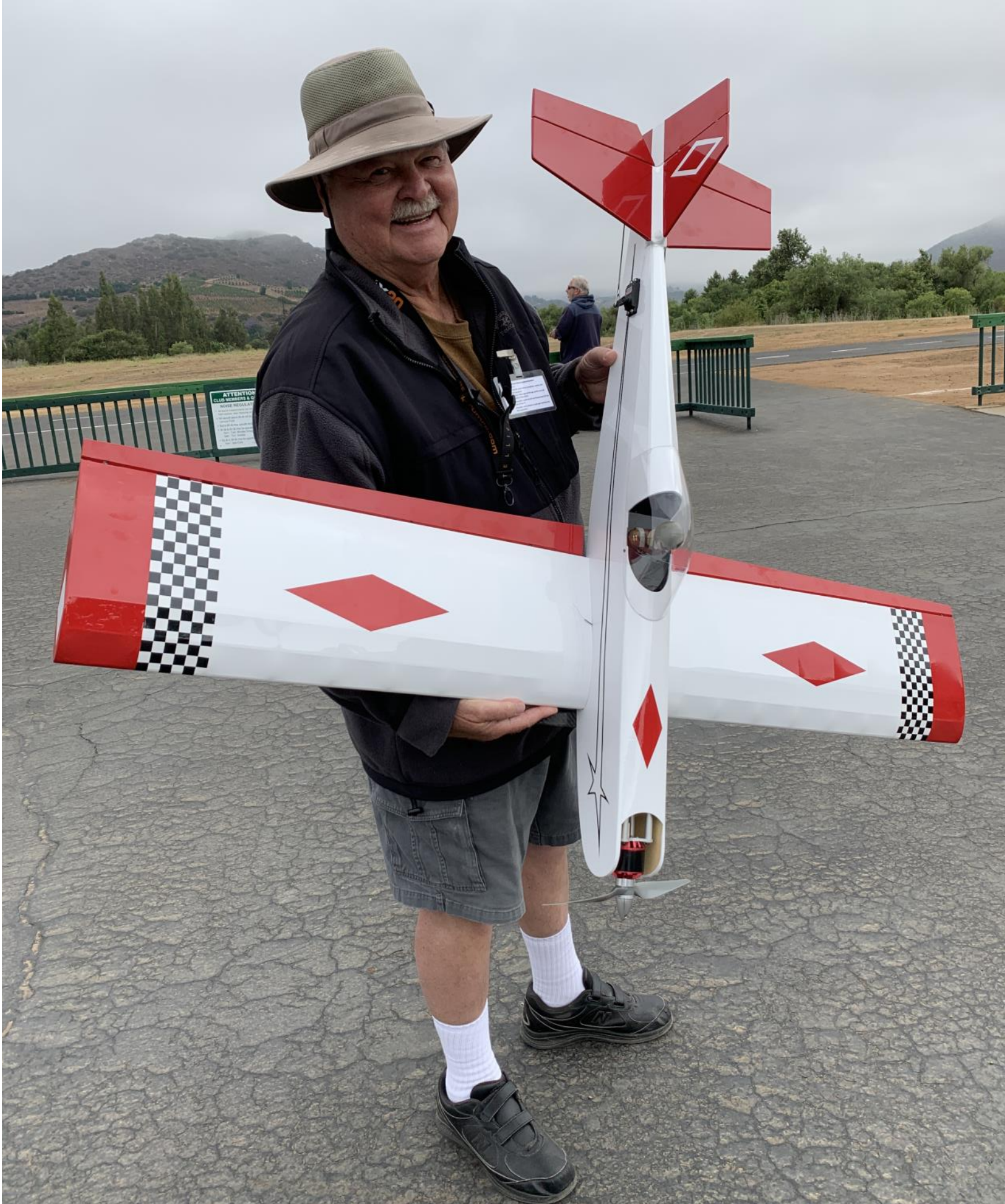
Varley Longson had successful flights with this new Sig 4-Star 40 he built from a kit. The wing is 60 in. and it is covered with Monokote. The electric motor is 46 equivalent 400 kv and the battery is 4500 6-cell. (Frank Burke photo)
