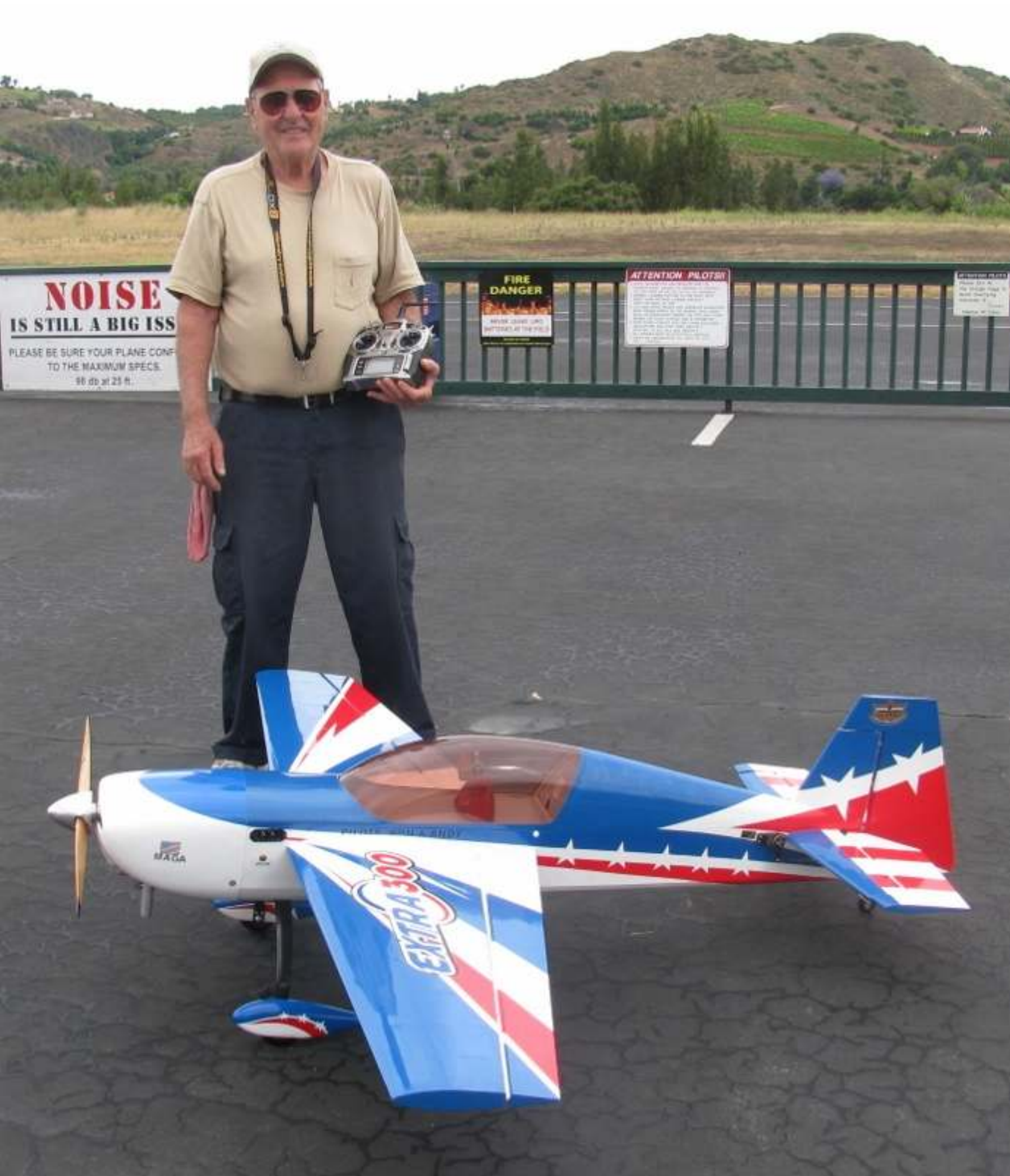
Here is Ron Schuyler and his new Extra 300 LP with a wingspan of 72 in. It is powered by an RCGF 32cc gas engine running an 18 x 10 prop. It is red/white/blue, outfitted with a smoke system, and is sporting our patriotic flag ready for 4th of July.
