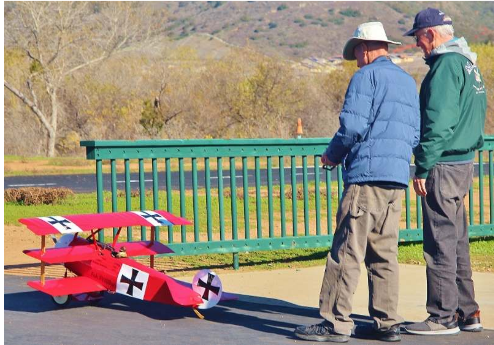
Bill Hill and Patrick Pratica with Bill's Great Plains Fokker DR-1. It needs lots of electric power. It has much inherent drag with three wings, a sub-wing and flat nose. It's fragile, flies just o.k..
