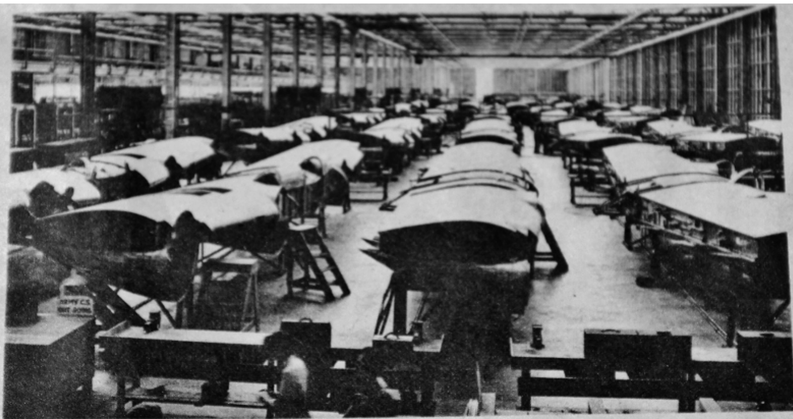
Coming right behind. Back in the plant more B-24 wing center sections are going together. Note engine nacelles under wing panels for four 1,250 h. p. P. & W. engines.
