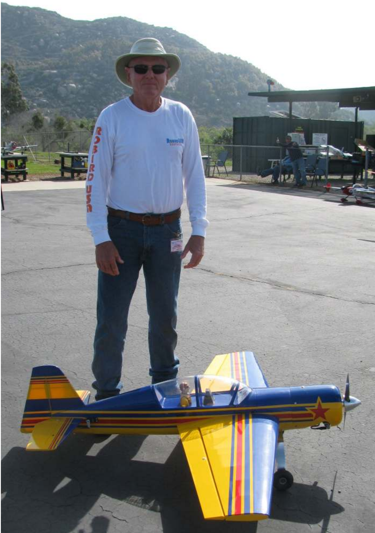
Don White maidenied this Seagull Yak 54 ARF that he put together in memory of his friend, Don Cleary, who recently passed away. The wingspan is 63 in. It is powered by a DLE-20cc gas engine running a 16 x 7 prop. The polished aluminum landing gear is from a Sig 300 Extra. He installed a Cortex gyro and a Spektrum power box receiver with built-in telemetry.
