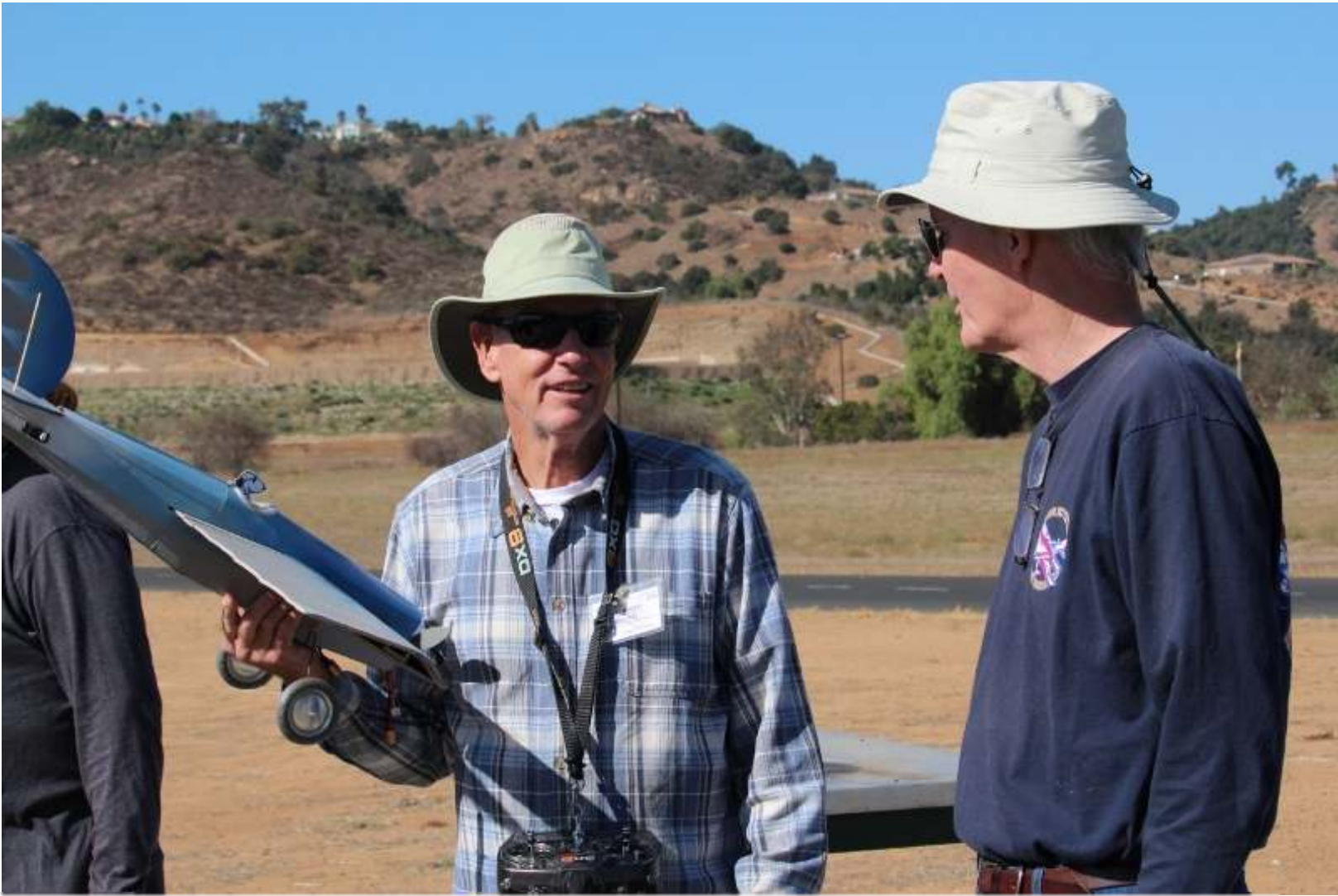
Bill Hill (center) flew his “paper” airplane for the Poker Fun Fly. Bill has about $2. of foamboard in the model and he made those wheels from the bottoms of aluminum cans. It’s a clever plane and flies great.
