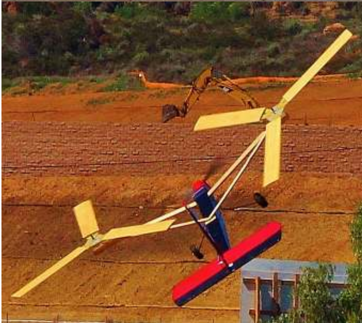
Look at the rudder turned for a right turn, but the craft continued to turn left.
