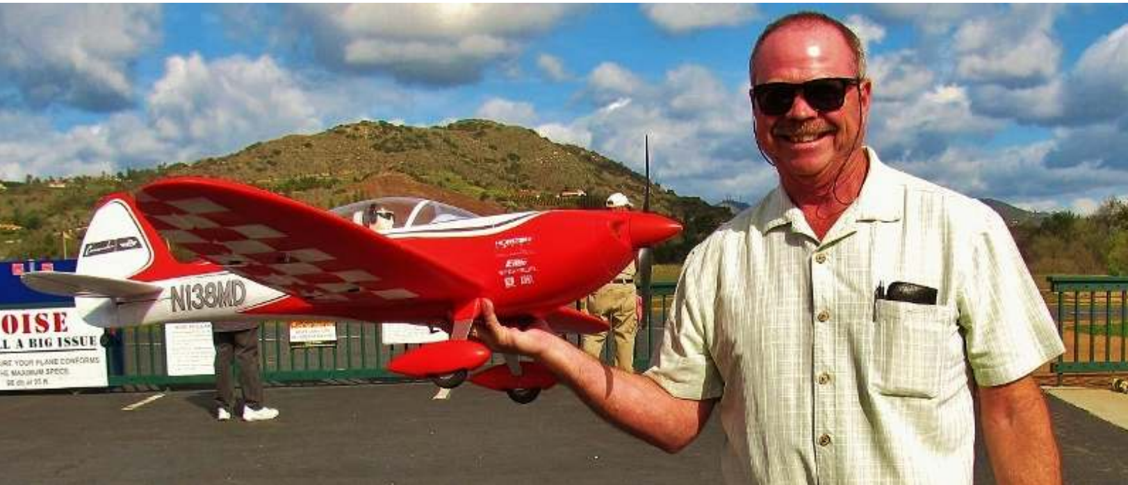
Chris Bunn also had a maiden flight with his new Commander from E-flite. It has a wingspan of 44 in. The 3S battery is 4000 mAh.
