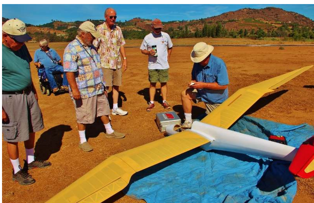
Vice President Steve Kerrin spent a few years constructing his Mini-Moa. Wingspan is 18 feet, weight is 30 pounds including 4 pounds of nose ballast. This was the first sailplane to use water ballast. 18 ounce wing loading and flies well. He maiden it on Thursday, August 30, 2018.
