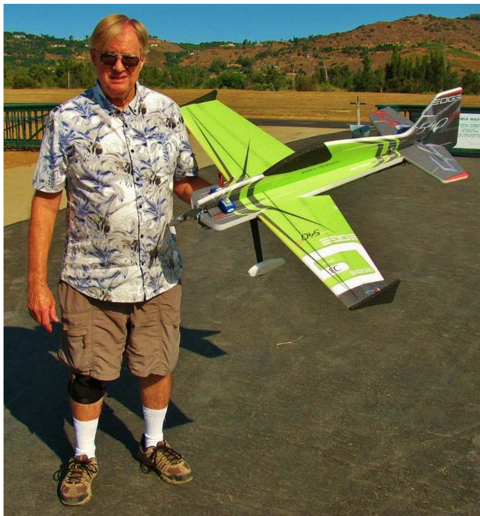
John Cutler took a maiden flight with his new electric Edge 540 from Twisted Hobbys. The wing-span is 43 in. It has an E-flite 10 motor and the 3 cell battery is 2200 mAh.
