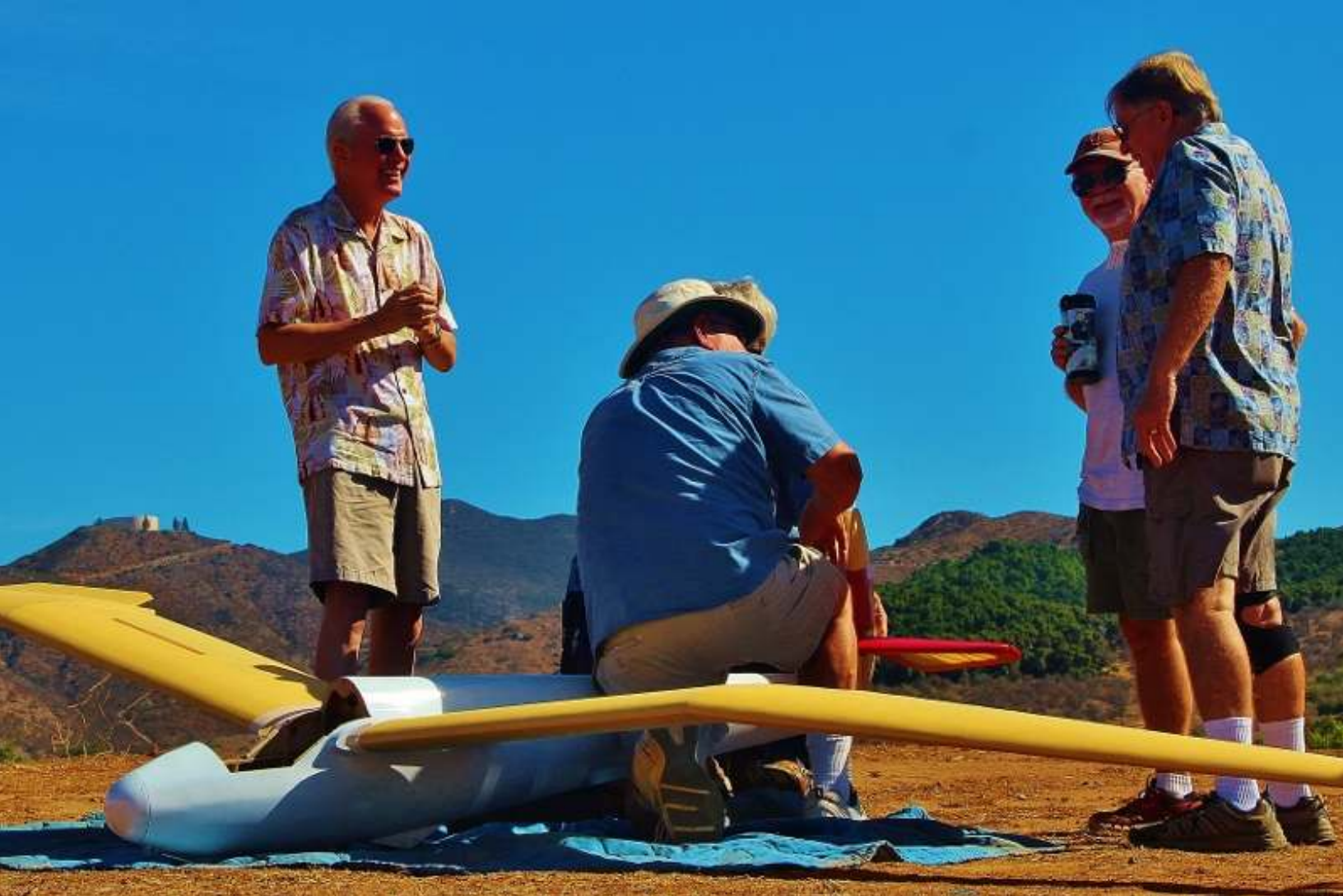
Vice President Steve Kerrin spent a few years constructing his Mini-Moa. Wingspan is 18 feet, weight is 30 pounds including 4 pounds of nose ballast. This was the first sailplane to use water ballast. 18 ounce wing loading and flies well. He maiden it on Thursday, August 30, 2018.
