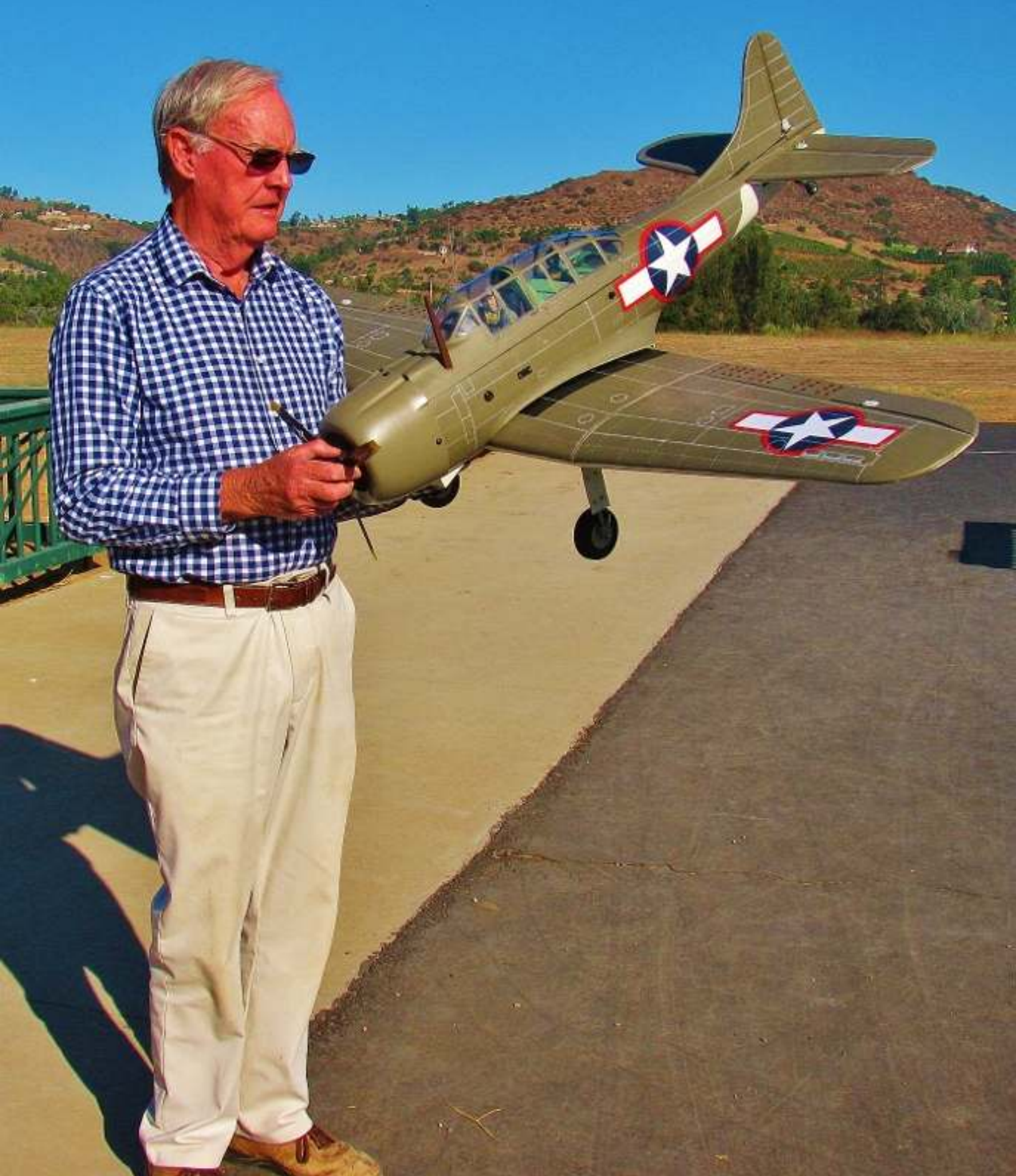
Alan Wolstenholme has a new Dauntless from VQ Models. It is powered by an OS-65-AX glow engine with a Pitts exhaust. He is running a 3-blade 12 x 6 prop. The battery is 2S and it has VQ electric retracts.
