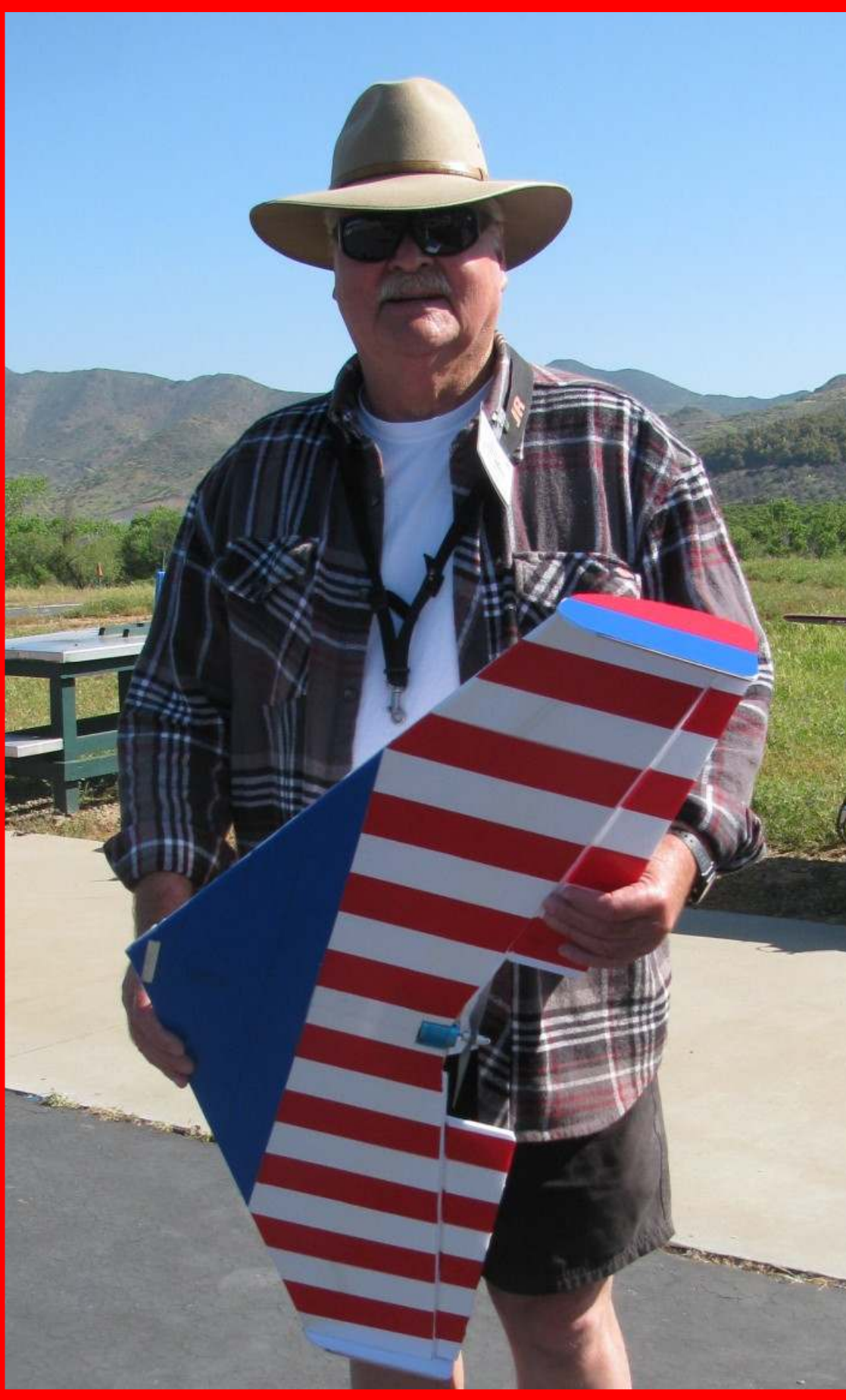
This is Varley Longson's 2nd new build from plans of an FT-Versa wing. It is made of foam board with elevons and has a 46 in. wing-span. It has a Himax 2815-2000 electric motor with a 30 amp speed controller.
