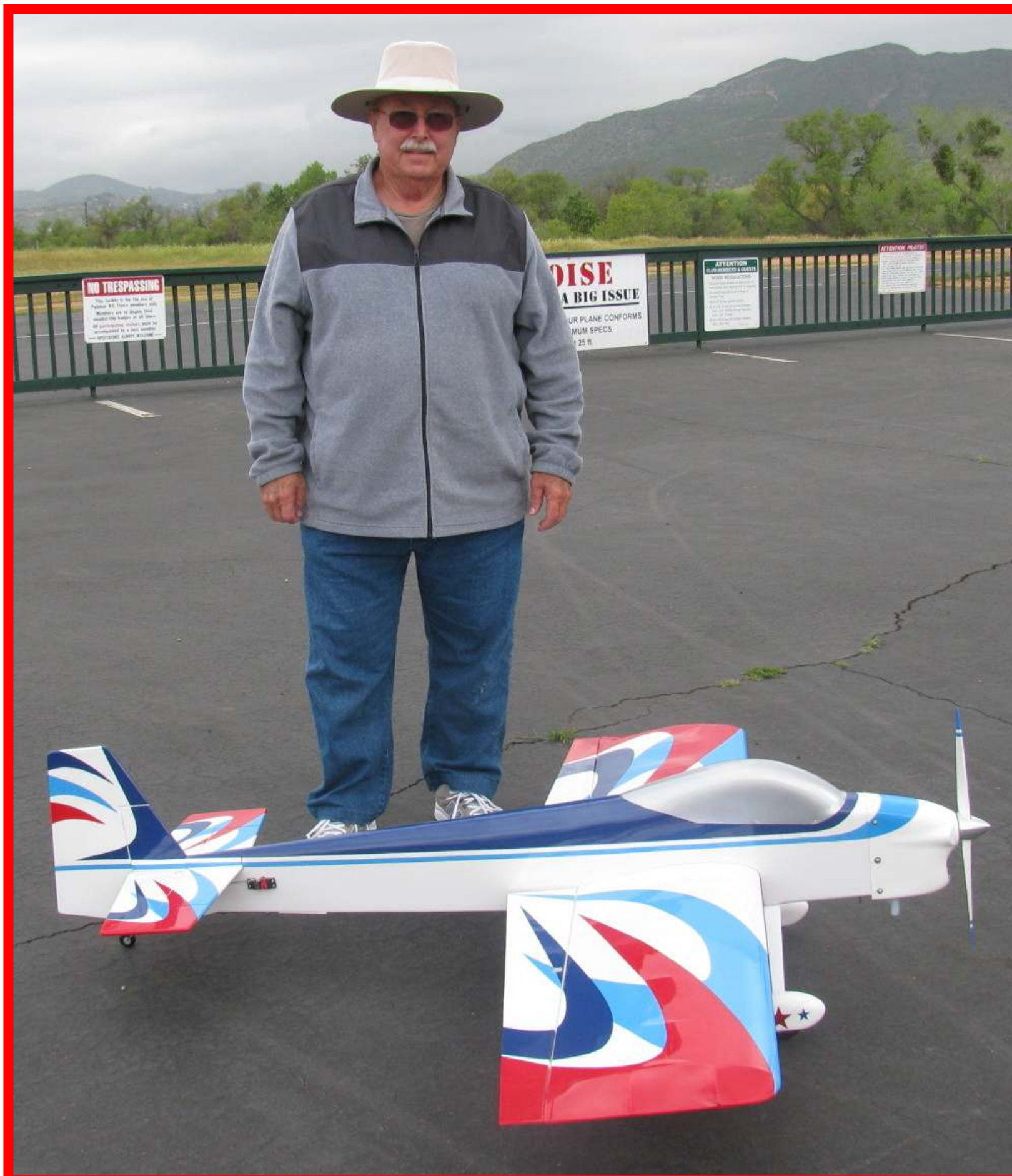
Frank Burke is flying this new U-Can-Do 60 size ARF from Tower Hobbies. It is powered by a DLE-20 gas engine with rear exhaust and uses a 17 x 6 prop.
