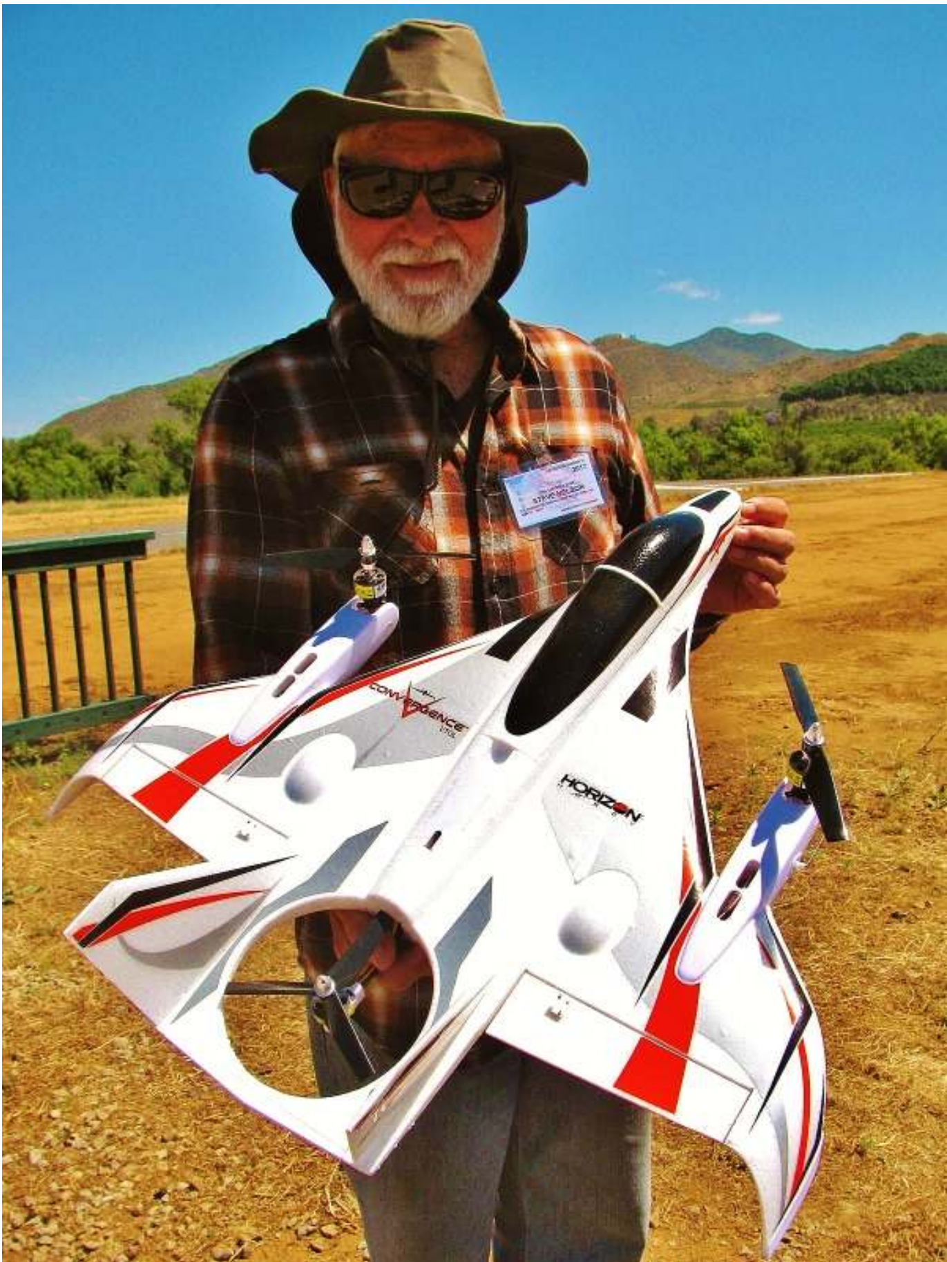
Steve Nelson is flying this new Coverage VTOL (vertical takeoff & landing) by E-flite from Horizon Hobby. It has 2 rotating electric motors on wings with 1 fixed-position motor in tail. It has a 3S battery 2200 mAh. It can be seen in flying demos on U-tube. Pilots have to work harder to transition between hovering and airplane flight and should be flown by an advanced or expert flyer. It comes with flight control software for automated transition. It is ready for set up to be used with first person view.
