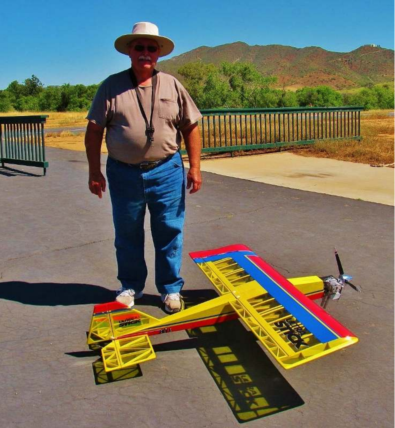
Frank Burke had maiden flight with new ARF Ultra Stick from Hangar 9. It is powered by an OS-120-AX two-stroke glow engine running a 3-blade Master Airscrew 15 x 7 prop. The wingspan is 66 in. and weight is 6 to 7 lbs.
