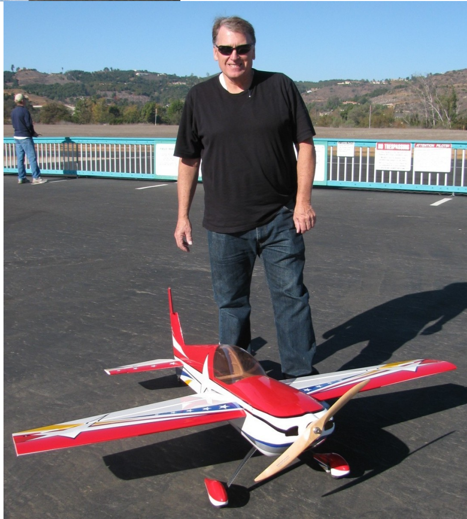
Mike Jensen also took a maiden flight with his new A. J. Slick from 3D Hobby Shop. It has a 71 in. wingspan and is equipped with a Hacker A50 16L electric motor, Hacker 70 amp ESC; two 4S--3850 mAh batteries; with a Master Air Screw 19 x 10 prop.
