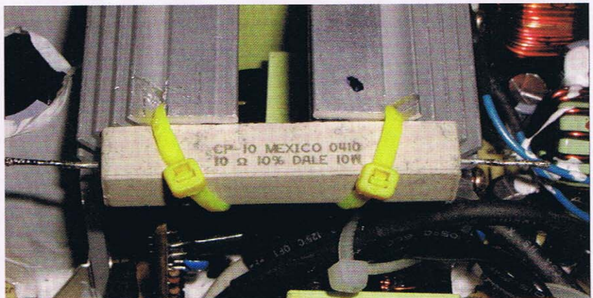
I drilled a small hole in each of these heat-sinks and secured the load resistor to them with nylon wire ties. Don't forget to use heat-sink compound between the resistor and the mounting surface. It helps to transfer the heat.
