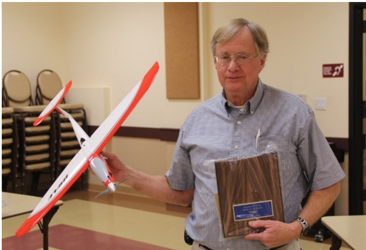
John Cutler built this electric powered fiberglass Rifle 5X5 for Gary Kaplan and won Model of the Month. It weighs 20 oz.; span 31"; length 24.5"; Prop 5X5; RPM 25-27,000. Motor E-Flite 3200KV; battery 3S @ 1800ma; speed @ 550 watts 120 mph (hopefully)
