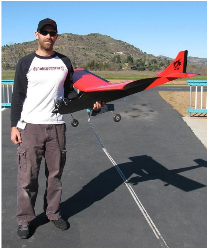
Curtis Pineau has a new A.J. Slick from 3D Hobby Shop. It has a wingspan of 89 in. and he is running a Q80 8m Hacker electric motor; Spin 200 speed controller; two 6S 5,000 MA battery packs from Nanotech.
