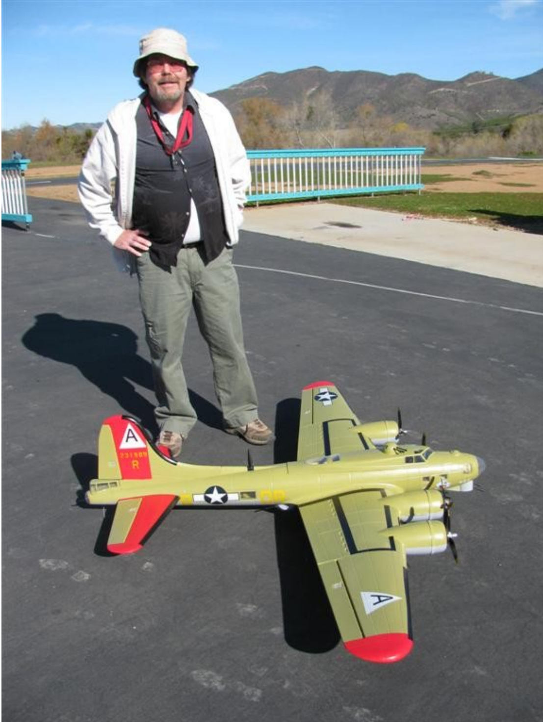
Ed Ramsey has a new electric scale B-17 Flying Fortress Bomber by Blitz RC Works from Banana Hobbies. It has a 79 in. wingspan, 3-blade props, flaps, & retracts. It has four brushless OutRunner KV750 motors, 45A brushless ESCs w/BEC, and two 14.8V 4S 2200 mah batteries.
