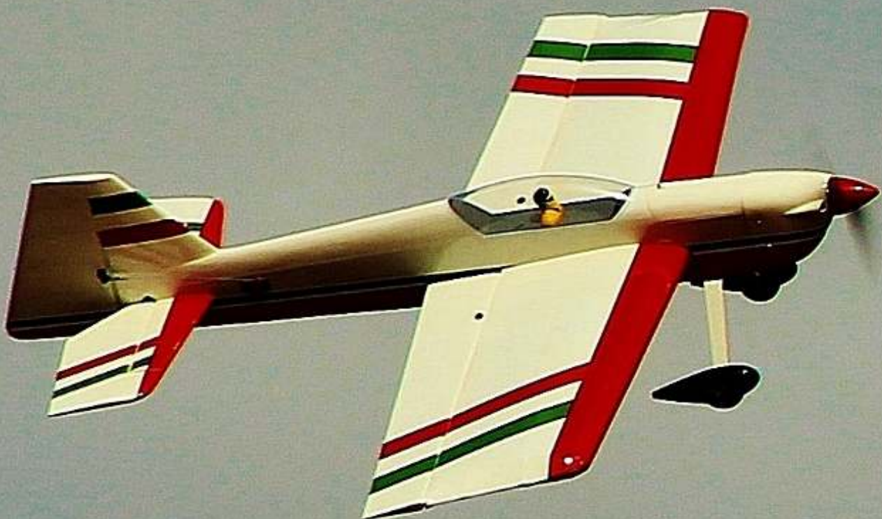
Greg Wilson's new electric Hero 3D from Phoenix is wonderfully aerobatic. It has an 18 oz. wing loading and a 63" span. These are the colors of Italy.
