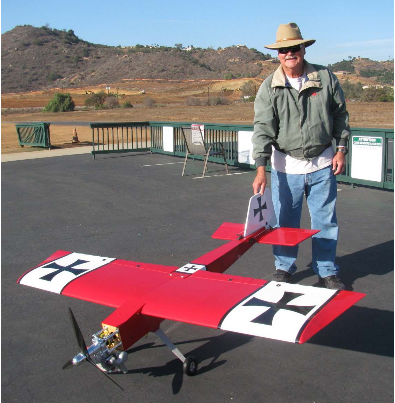
Varley Longson is flying this new Giant Big Stick ARF from Great Planes. The wingspan is 80 in. and it weighs 14 lbs. 11 oz. It is powered by a DA-50 gas engine running a 3-blade Mejzlik 20 x 10 carbon fiber prop. He modified the original tail & made a new vertical stabilizer and rudder.
