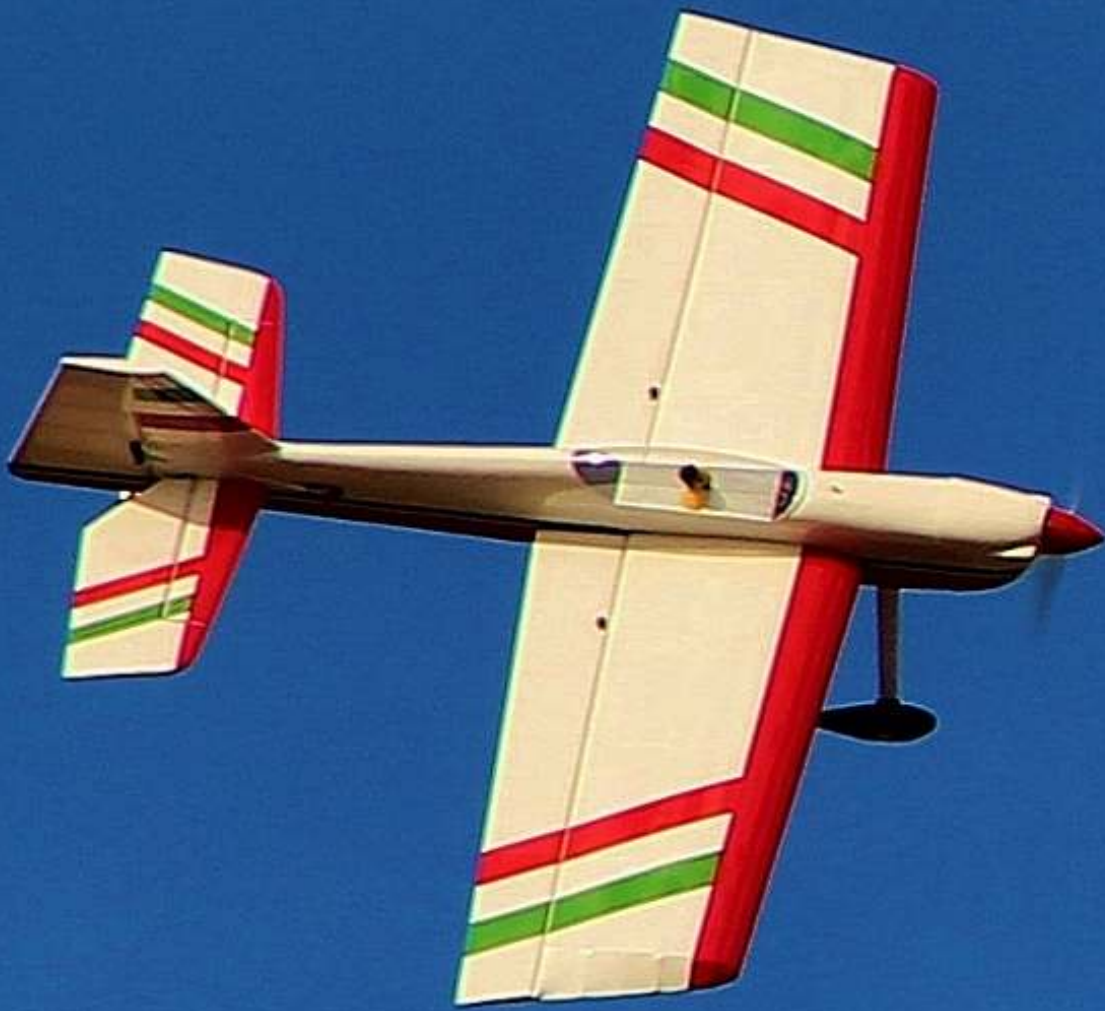
Greg Wilson's new electric Hero 3D from Phoenix is wonderfully aerobatic. It has an 18 oz. wing loading and a 63" span. These are the colors of Italy.
