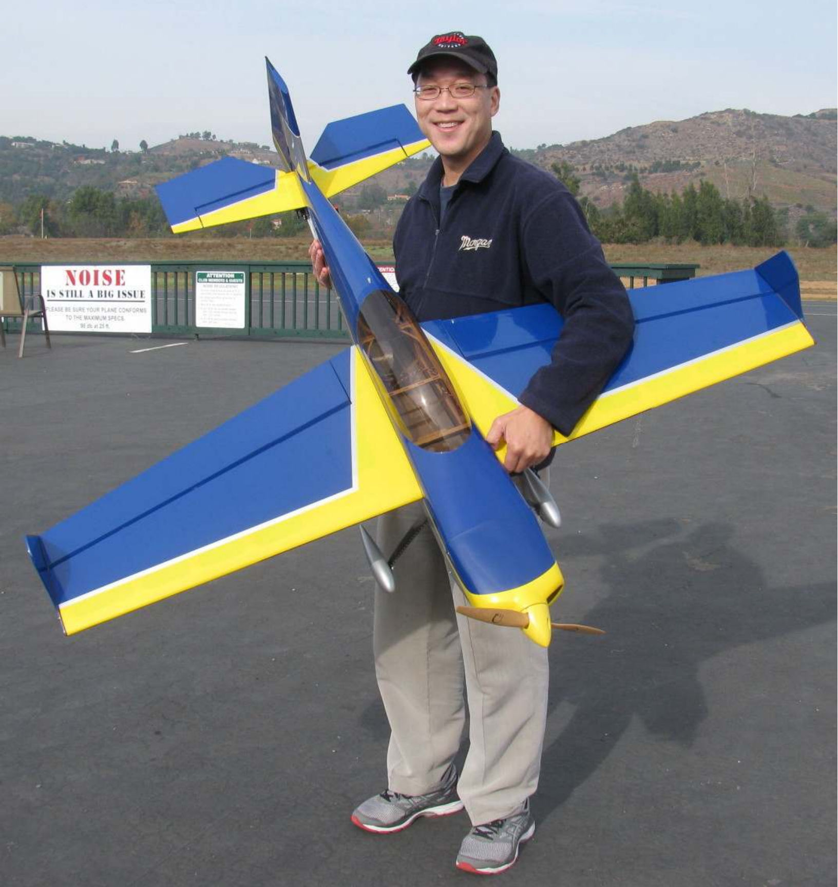
Kelvin Phoon is flying this new Edge 540T from Extreme Flight. The wingspan is 60 in. It has a Torque 4016 electric motor with a 16 x 7 prop; Castle Talon 90 ESC; and a 6S Thunder Power 55c battery 3300 mAh.
