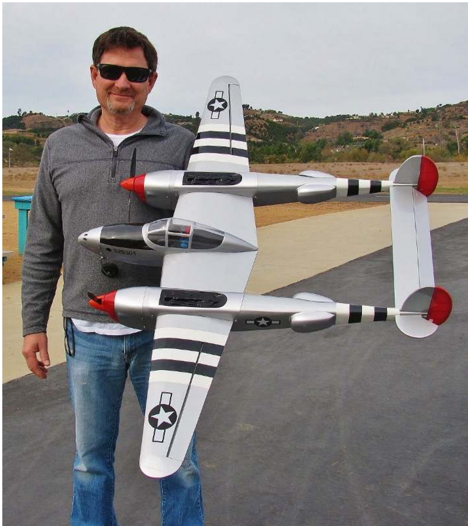
Here is Dave Swaffer after having a successful maiden flight with his new P-38 Lightning ARF. It has a 40 in. wingspan, and it is flown with twin E-max 2820 electric motors. It has two E-max 30 amp ESC's and two 1500 mAh 3S batteries. He is using a Spektrum 4 channel receiver.
