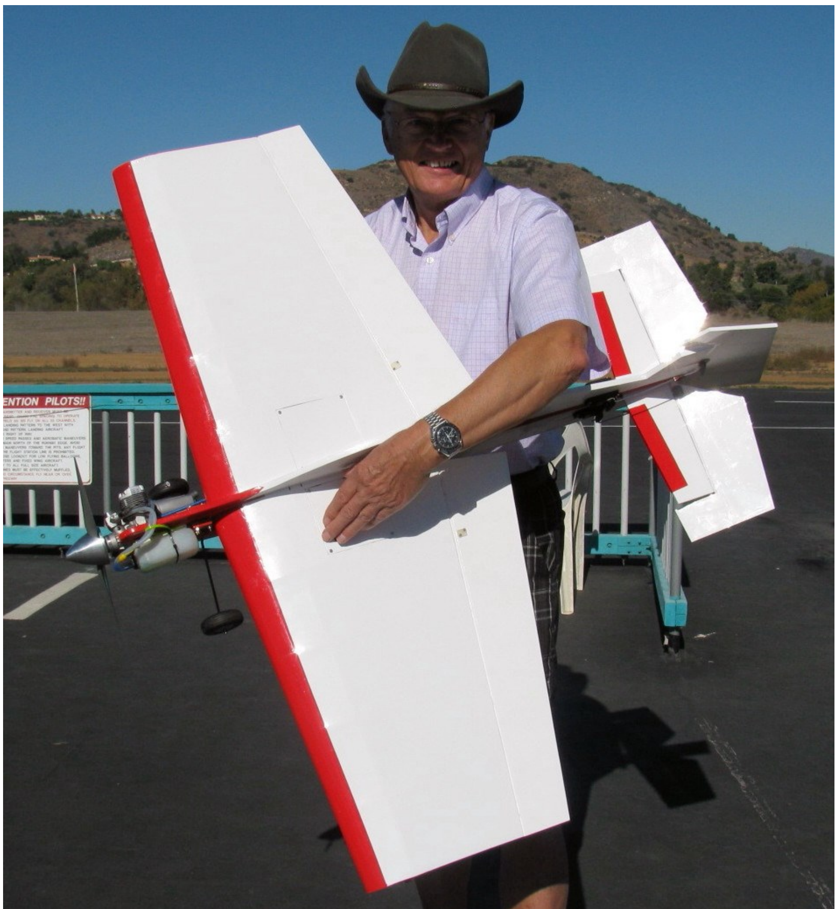
Graham Lloyd has built this new balsa 3D Profile Mojo from Paul Swanson plans and CNC parts. It has a 52 in. wingspan and weighs 5 ½ lbs. It is powered by an OS-46-AX glow engine with a 12 x 4 prop. It has a carbon fiber rod running through the center front-to-back and has a ½ in. plywood mount for the engine. This is an American made kit, but Graham is the only one here in our club that has built one, and this is his 5th build of same. There are 8 of these flying in his club back home in the U.K.
