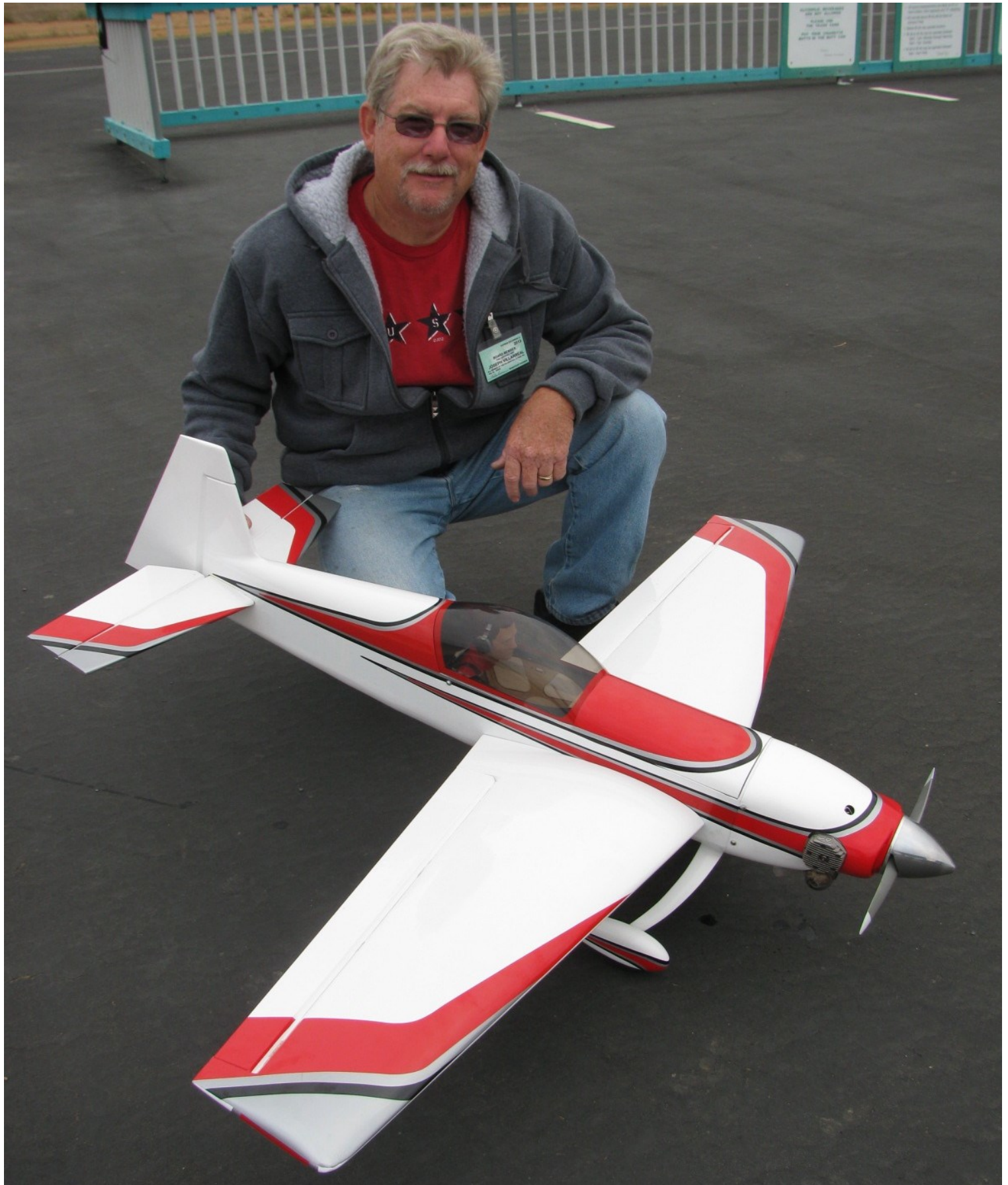
Joe Villarreal had a successful maiden flight with his new Revolver ARF from Great Planes. It has a wingspan of 59 in. and weighs 7 lbs. 2 oz. It is powered with an OS-75 AX two-stroke glow engine running a 12 x 8 APC prop.
