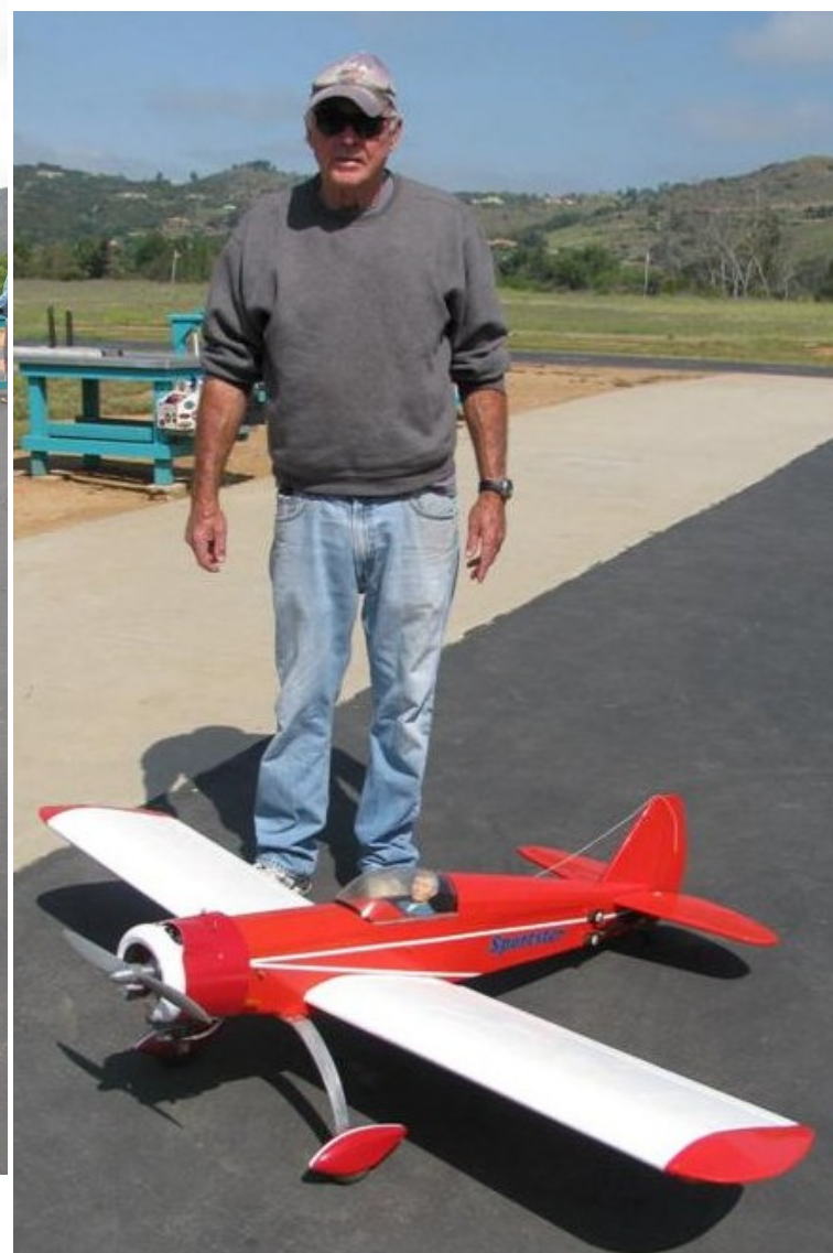
Bob Matthiessen is flying this Sportster 60. It is powered by an Echo chain saw motor with a 16 x 8 prop
