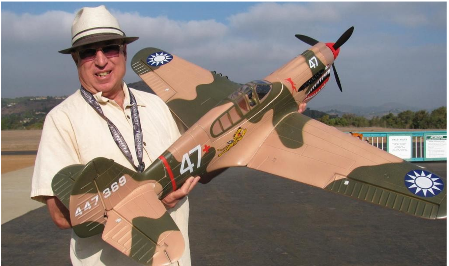
Roy DeMille has a new P-40 Warhawk from Airfield with a wingspan of 43 in. It has a brushless electric motor with a 2200 mAh battery.
