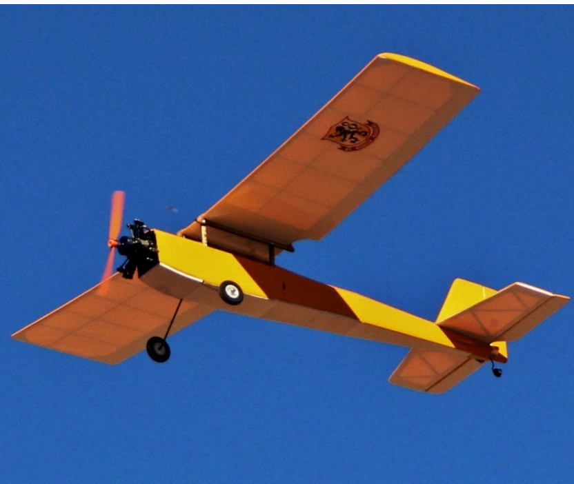
Nov. 13, 2012 John Grimm built and flew this 1970's design of the Q-Tee. It originally flew with an .049 but he converted it to electric. That's a 3 cylinder dummy engine. Joe Buko photos
