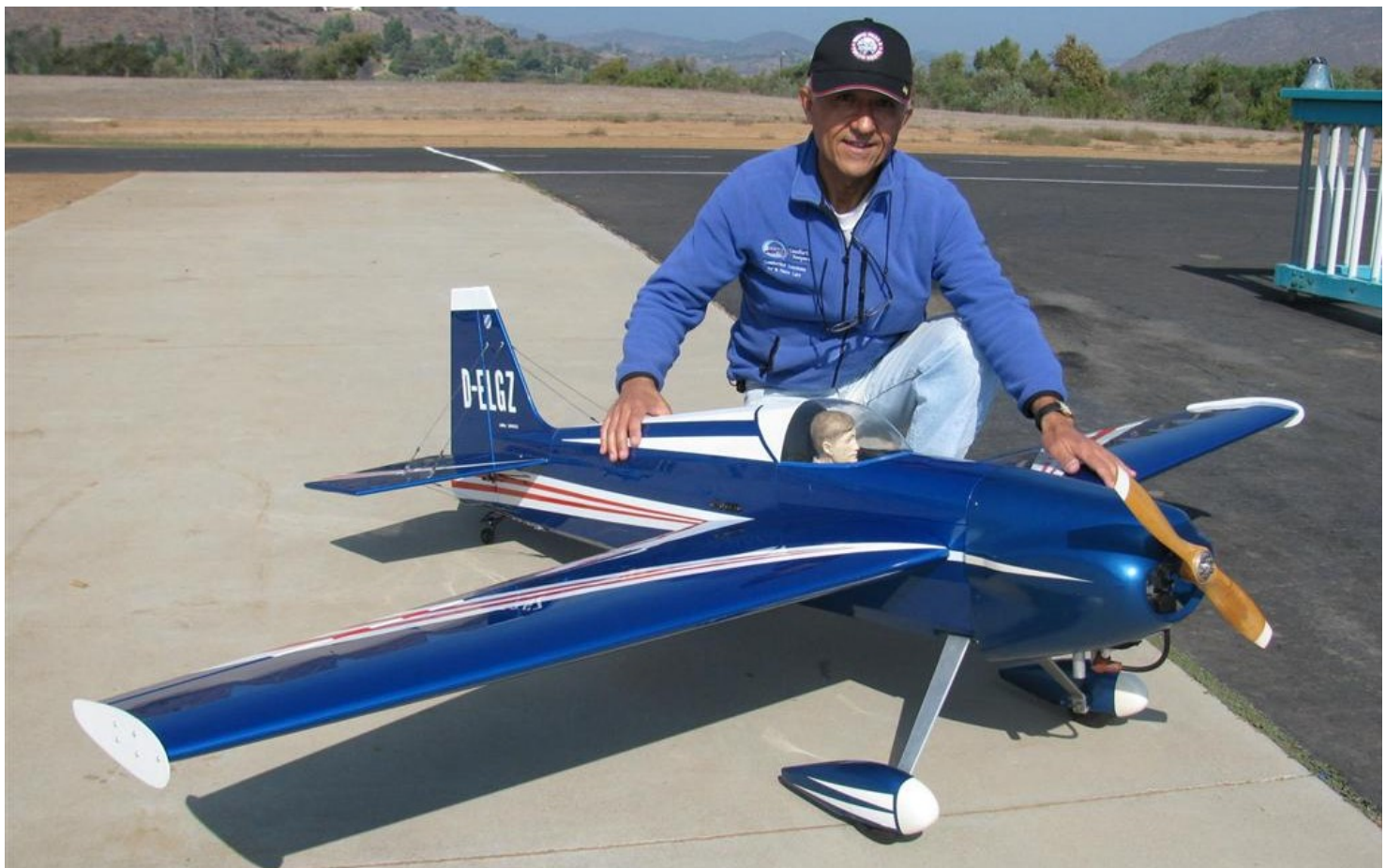
"Welcome" to new member, Cesar Fernandez-Mansilla. He had this Laser refurbished that was built from a kit some time ago. It has a wingspan of 87 in., and it is powered by a Zenoah G-38cc gas engine with an 18 x 8 prop. It weighs 17 lbs. Ethel Burke photos
