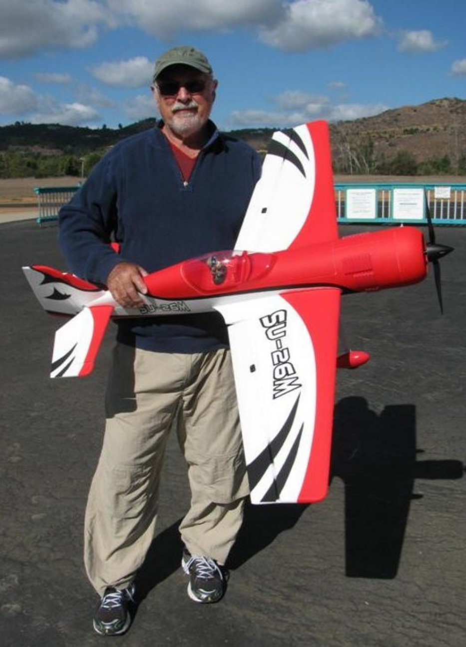
Roger Cosio has a new Buzzard Bombshell and made a successful maiden flight with it. It was partially built by Gary Sheldon and was stored in his attic for several years until he donated it to Roger. It was completed and covered in Monokote. It has a 70 in. wingspan with an Axi 2826/12 electric motor, 36 amp ESC, and an 11.1 3-cell battery.
