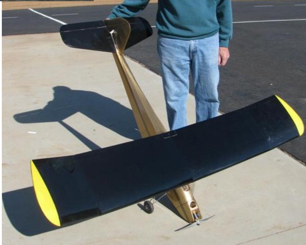
Roger Cosio has a new Buzzard Bombshell and made a successful maiden flight with it. It was partially built by Gary Sheldon and was stored in his attic for several years until he donated it to Roger. It was completed and covered in Monokote. It has a 70 in. wingspan with an Axi 2826/12 electric motor, 36 amp ESC, and an 11.1 3-cell battery.
