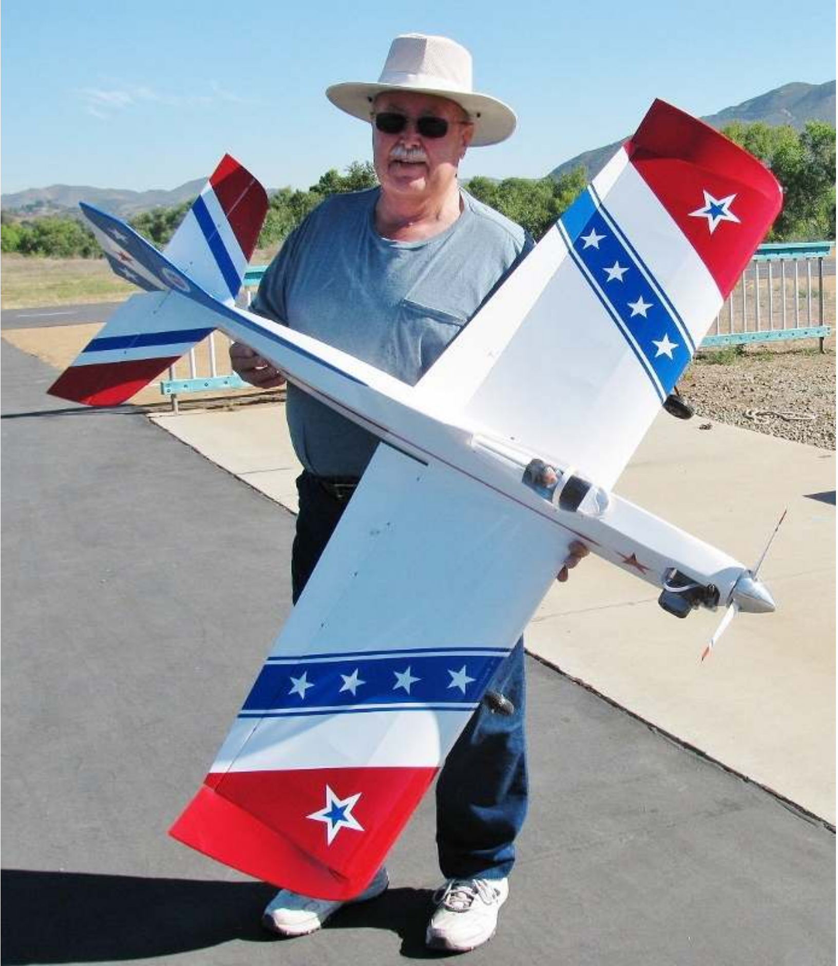
Frank Burke has built this new Contender from a Top Flite kit (still available). The wingspan is 61 ½ in. and it weighs 7 lbs. 10 oz. It is powered by a 75 Super Tigre 2-stroke glow engine with a Bisson exhaust. It has a 3-blade Master Airscrew prop 12 x 6. It has electric retracts from Hobby King.
