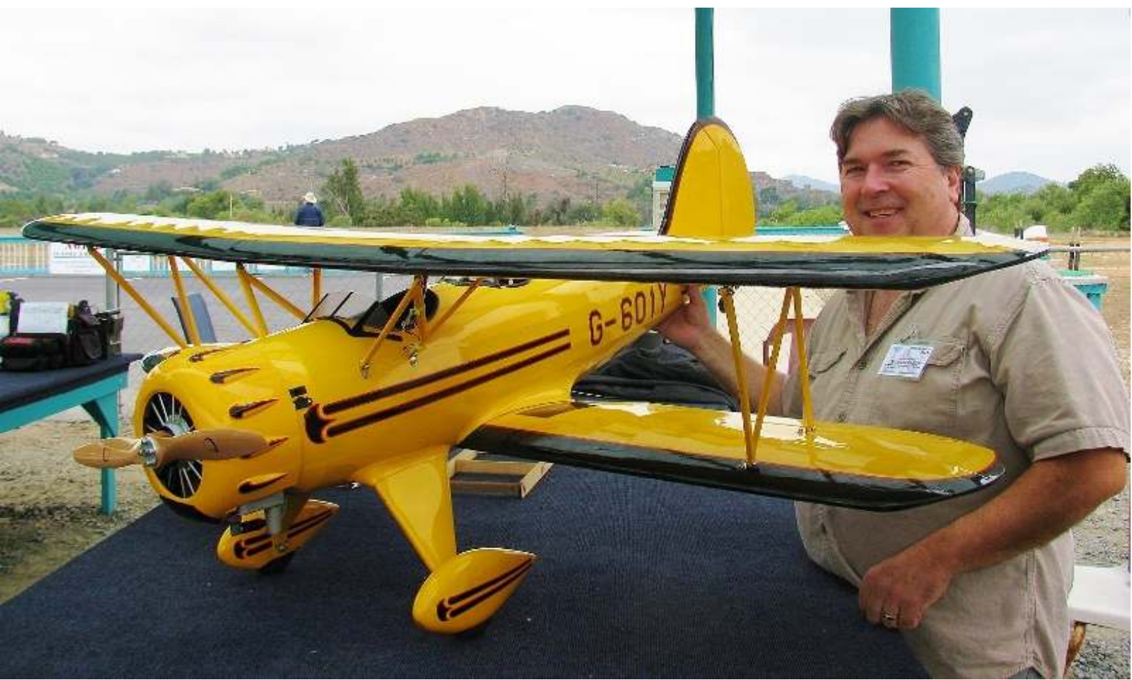
Richard Martin is flying this classic Waco YMF-5D biplane ARF from Great Planes. The wingspan is 72 in. with a wing area of 1384 sq. in. It is powered by a DLE-30cc gas engine running an 18 x 8 Xoar prop. It has 2 Lipo batteries and weighs about 13 lbs. (Note that this Waco has a double cockpit.)
