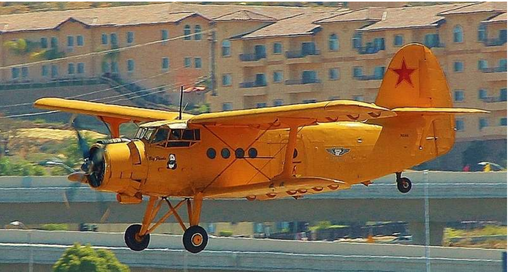
This Antonov AN-2 is the world's largest bi-plane, first manufactured in Russia where 5,000 were built. Poland delivered 11,950 of these since 1960. The proto-type first flew in 1947. It has a 1,000 hp engine, a 60'9" span and flies 8 to 10 passengers. It is a reliable freight hauler, especially in the back country. The Commemorative Air Force owns this one. It's ugly, but there was another plane even more ugly that appears on page 61 of this issue.
