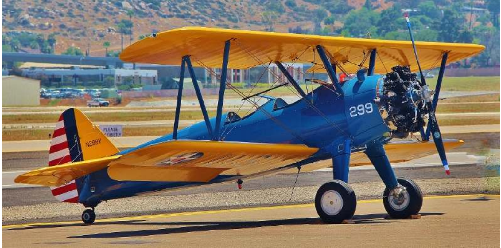
Stearman Aircraft/Boeing made PT-17's with a 225 hp engine. Made in 1934 during the Golden Age of Flight.
