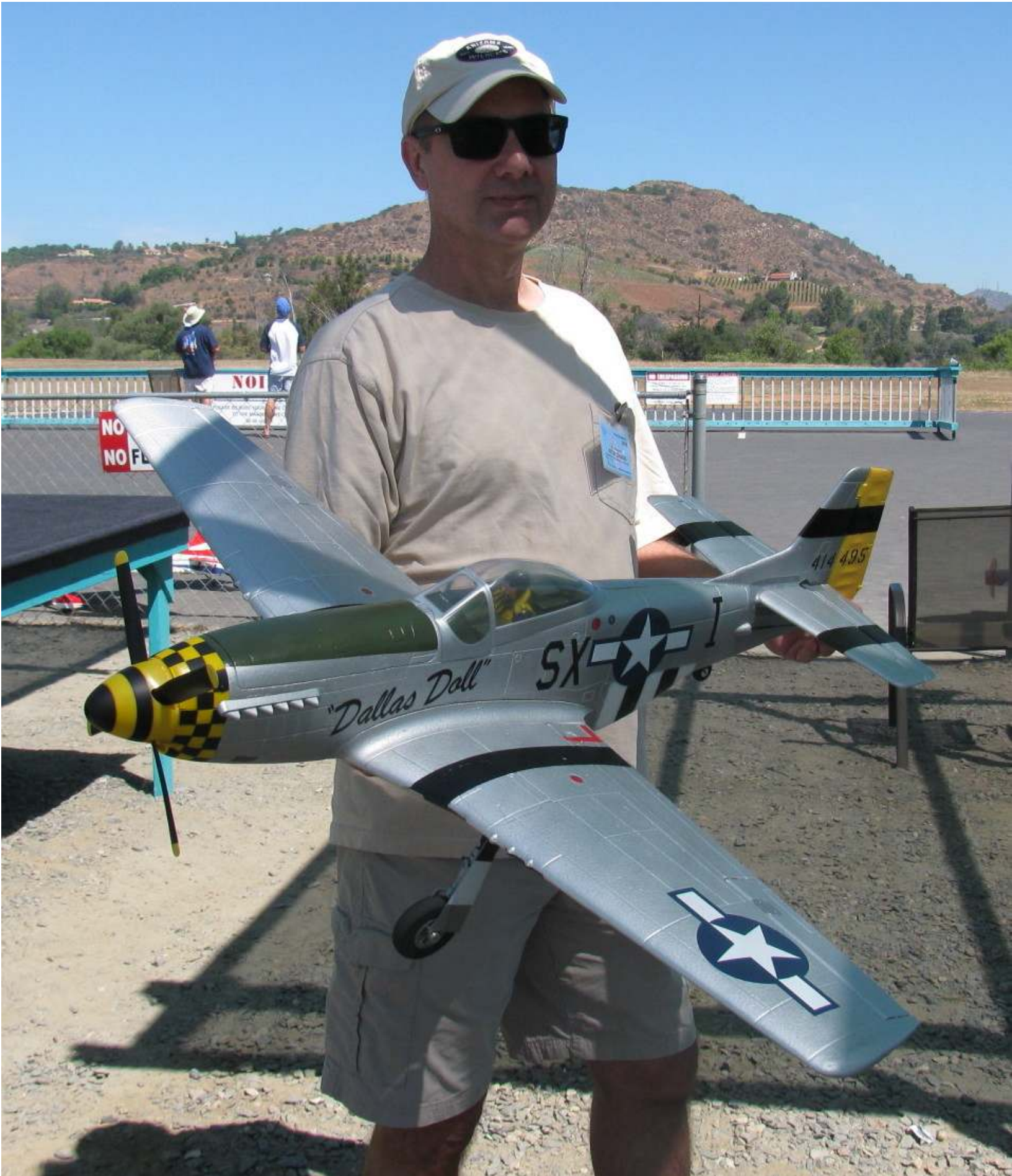
Pete Uscinski is flying this new P-51 Mustang from E-flite. It has a 44 in. wing-span with electric retracts, and a 4-blade prop. It has an E-flite electric motor, 40 amp ESC, and a 3S battery 2200 mAh.
