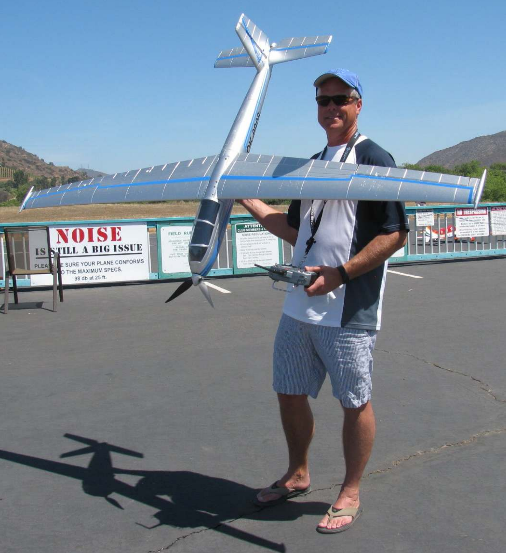
Greg Farrell has a new 8 ft. wing Blanik glider from Hobby King. It has an electric motor with folding prop, 40 amp ESC, and a 3S battery 3300 mAh.
