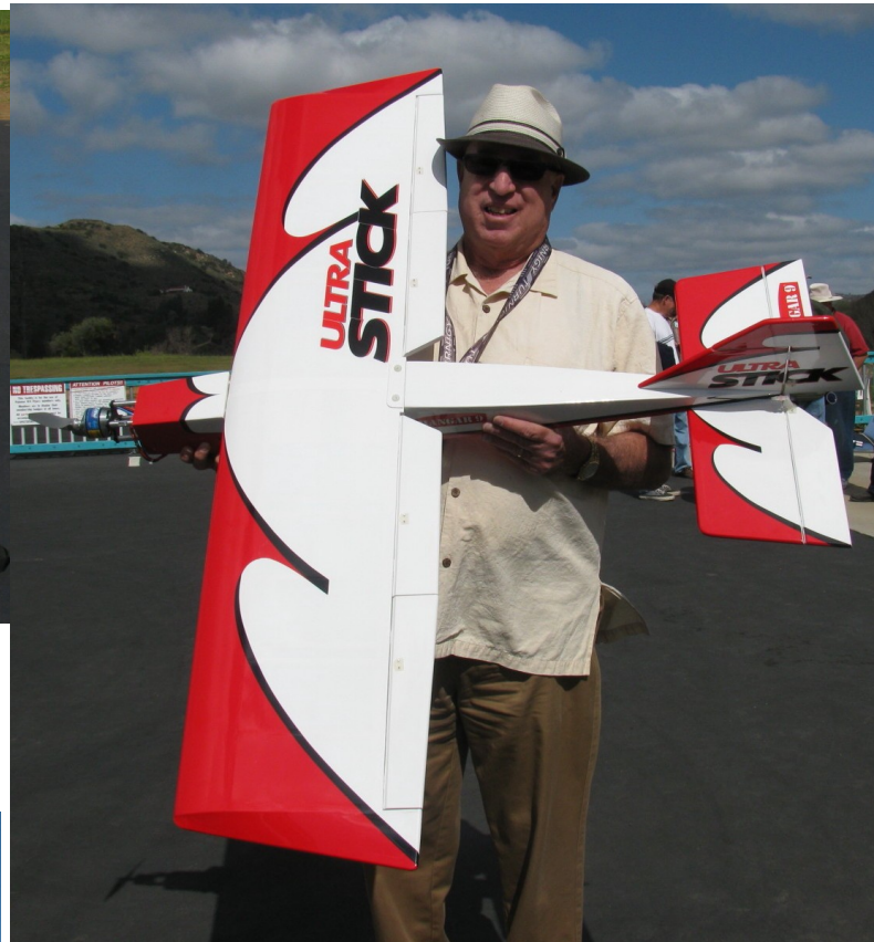
Roy DeMille has a new Ultra Stick 40 ARF from Hangar 9. It has a wingspan of 57.5 in. and the length is 51 in. It has an E-flite power 46 motor; 60 amp ESC; and a 4000 mAh 4 cell battery with a 6 channel receiver. Roy searched 5 states looking for this plane and finally found the last one which he had shipped in from Texas.
