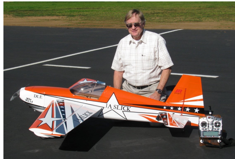
John Cutler has a new A. J. Slick from 3D Hobby Shop. It has a 71 in. wingspan. It is powered by a DLE-30cc gas engine. He made the graphics from Ultracote using his wife's craft cutting machine.
