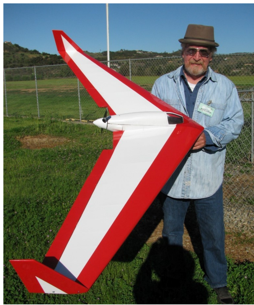
Marv Clemens has scratch-built this new "Winglet" with tri-gear from plans in Model Aviation News. It has a wing-span of 74 in. and is built with balsa and covered in Monokote. Note the good viewing on bottom of wing. He is running a "pusher" 40 size Outrunner electric motor with a 12 x 6 prop and 6 cell 4000 mAh battery.
