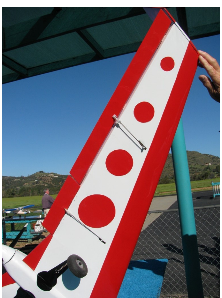
Marv Clemens has scratch-built this new "Winglet" with tri-gear from plans in Model Aviation News. It has a wing-span of 74 in. and is built with balsa and covered in Monokote. Note the good viewing on bottom of wing. He is running a "pusher" 40 size Outrunner electric motor with a 12 x 6 prop and 6 cell 4000 mAh battery.
