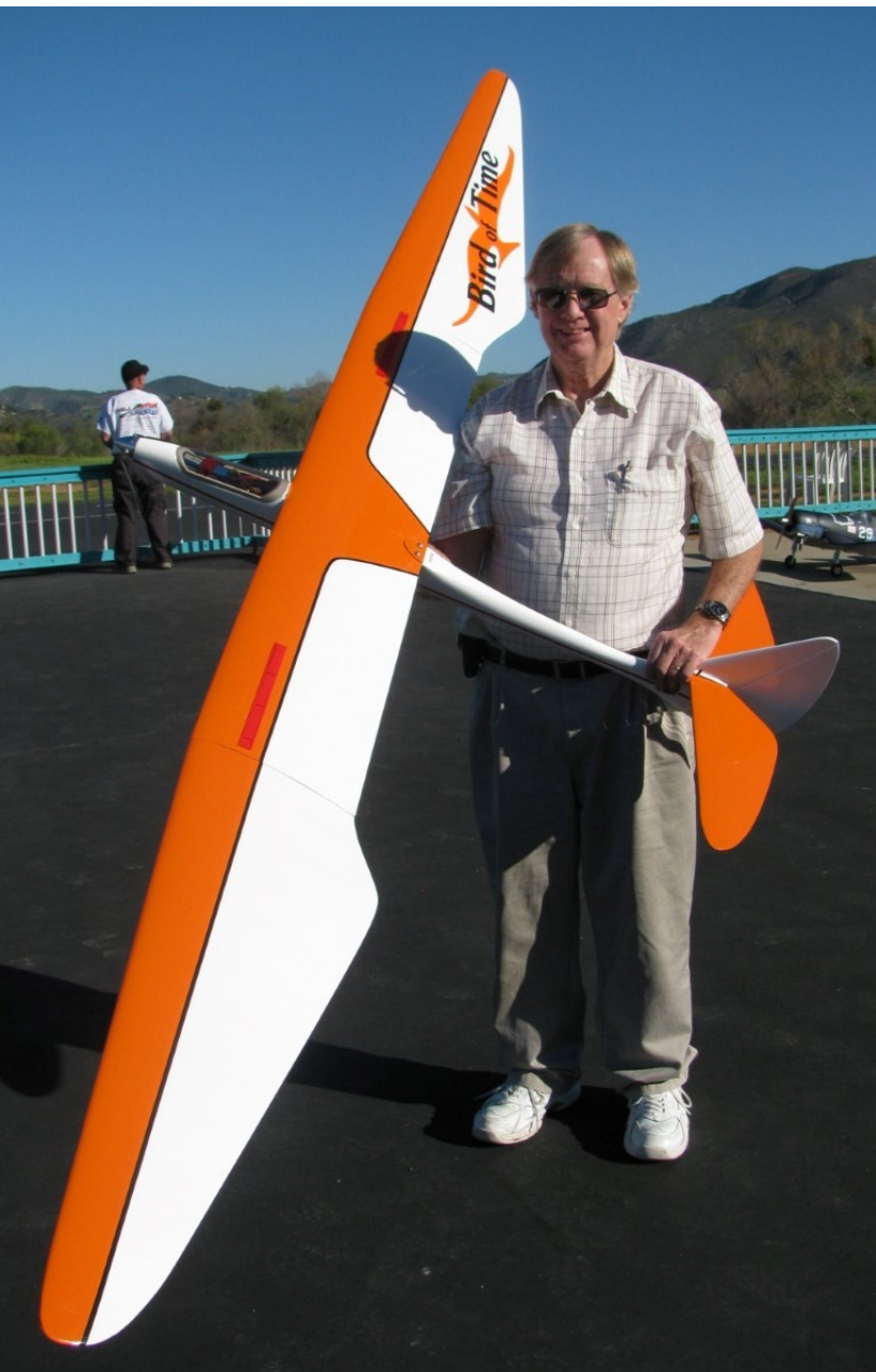
John Cutler has a new A. J. Slick from 3D Hobby Shop. It has a 71 in. wingspan. It is powered by a DLE-30cc gas engine. He made the graphics from Ultracote using his wife's craft cutting machine.
