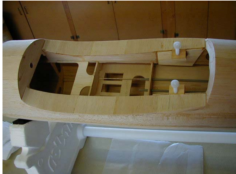
Wing cradle sheeting, wing mounting blocks & control rods installed
