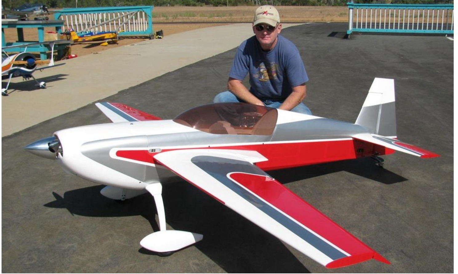
Dave Litaker and his very quiet DA 120cc twin with MTW RE-2 tuned pipes, Mejzlik 28/12 carbon fiber prop. Hangar 9 Extra 300. Ethel Burke photo
