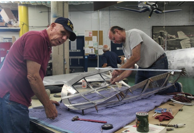
Volunteer builders Chris Sundahl and Bob Parker work the Bell X-1 canopy.
