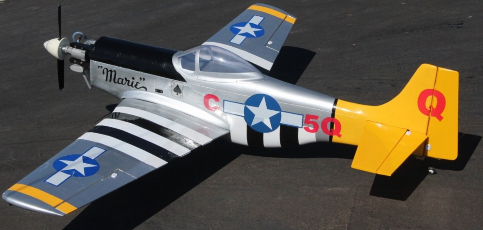
Bill Demore's Mustang is repaired after a retract stuck in flight and drained the battery. Now the retracts have their own energy source. It's a Nitro model which weighs 9 lbs, is powered with a Thunder Tiger .61, 65.5" wingspan and flies well. Joe Buko photos
