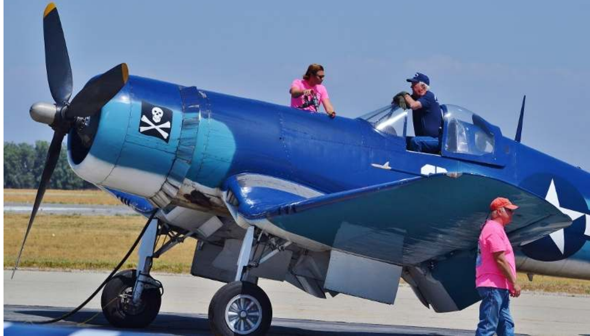
Chance-Vought F4U Corsair made its first flight in May 1940 with a top speed of about 385 mph though in a dive it flew over 400 mph.
