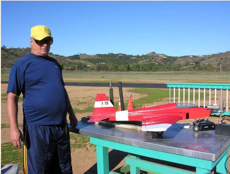
Here is Claude Sirgant with his new F-20 Tiger Shark fighter jet. It is powered by an OS-46 glow engine.
