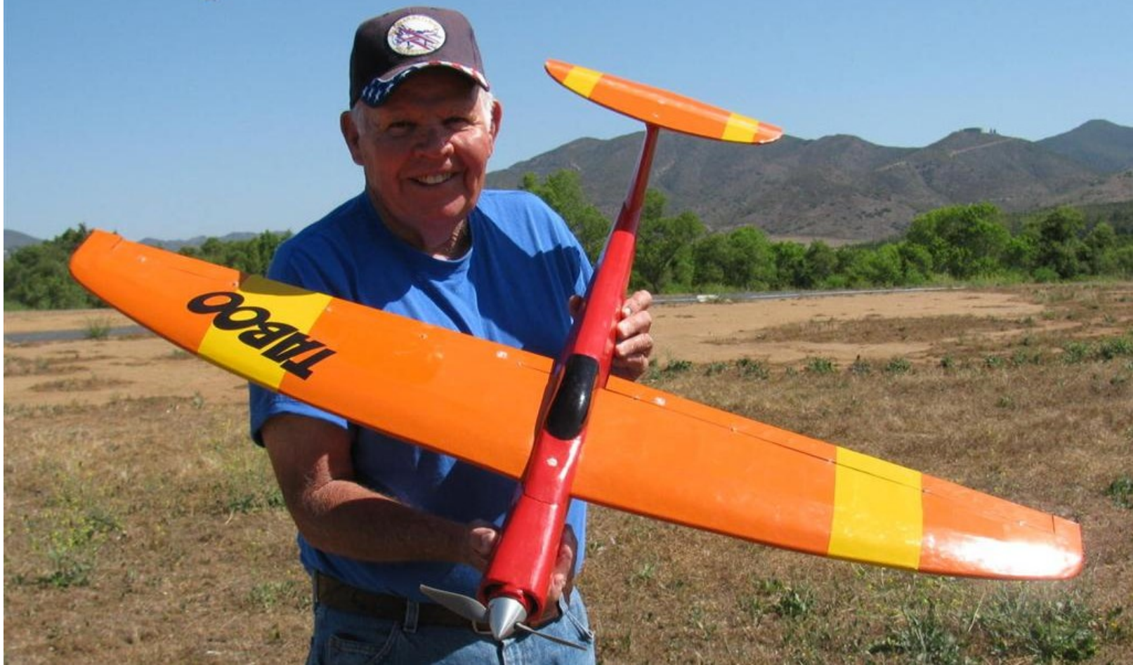
John Hartsell, Sr. built this new Taboo from scratch in 4 months. He found the plans in an English model airplane magazine. It weighs 2 lbs. 1 oz. John, Jr. put all electric in it using a Cobra KV-1390 motor, 45 amp speed control, 4 cell battery, and Hitec servos. He made a successful maiden flight with the Taboo on Memorial Day.
