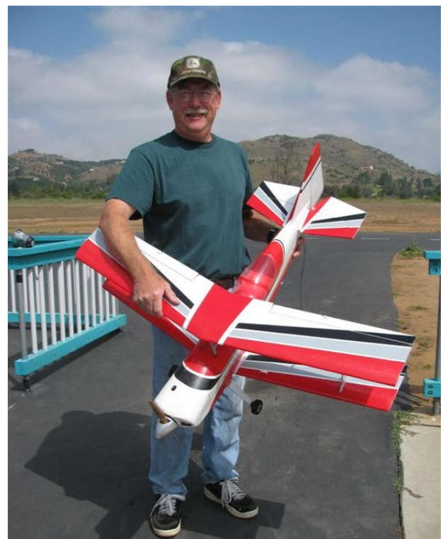
Also " Welcome " to Joe Villarreal who is another new member joining our Club from the "Bonsall Boys" group. Joe is flying this Ultimate Biplane from CMP. It is powered by an OS-46 two-stroke glow engine with an 11 x 7 prop. The wingspan is 41 in. Joe also flies an Extra 260 from Hangar 9 on page 12. It has a wingspan of 78 in. and is powered by an OS-1.60 cu.in. two-stroke glow engine with a 16 x 6 prop. It weighs 12.5 lbs. Variety is good, and so Joe flies this P-40 Warhawk ARF from VQ Models. It has a wingspan of 62 in. and is powered by a Saito 100 four-stroke glow engine. It weighs 8 lbs.
