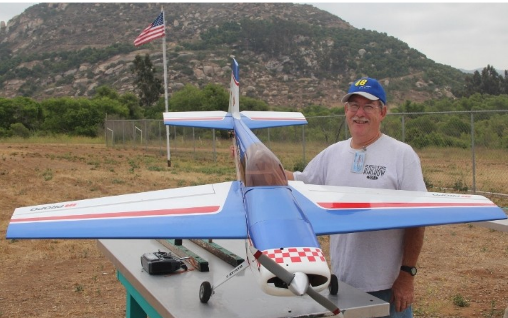
Joe Villarreal with his Hangar 9 X260. O.S 160 FX 2 stroke with a 78" span on June 9, 2012
