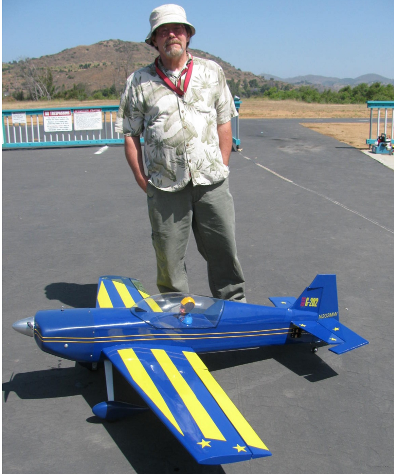
Ed Ramsey has built a Giles 202 from a Midwest kit that is now discontinued. It is covered in Ultracote. It has a 72 in. wingspan and is powered by a Saito 180 four-stroke glow engine with a 16 x 8 APC prop. It weighs 12 lbs. Ed also had a successful maiden flight with this new F4U Corsair ARF just out from Top Flite. It has a wingspan of 62 in. and weighs 9.5 lbs. It is powered by a Saito 100 with a 3-blade 13 x 8 prop and has Century Jet retracts.
