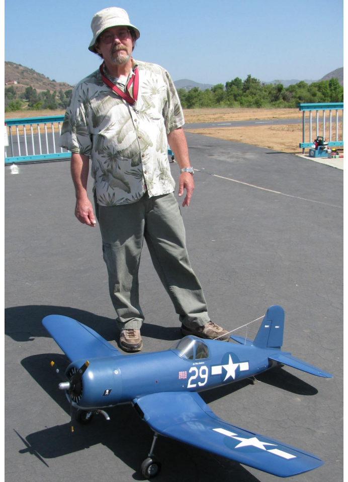
Ed Ramsey has built a Giles 202 from a Midwest kit that is now discontinued. It is covered in Ultracote. It has a 72 in. wingspan and is powered by a Saito 180 four-stroke glow engine with a 16 x 8 APC prop. It weighs 12 lbs. Ed also had a successful maiden flight with this new F4U Corsair ARF just out from Top Flite. It has a wingspan of 62 in. and weighs 9.5 lbs. It is powered by a Saito 100 with a 3-blade 13 x 8 prop and has Century Jet retracts.
