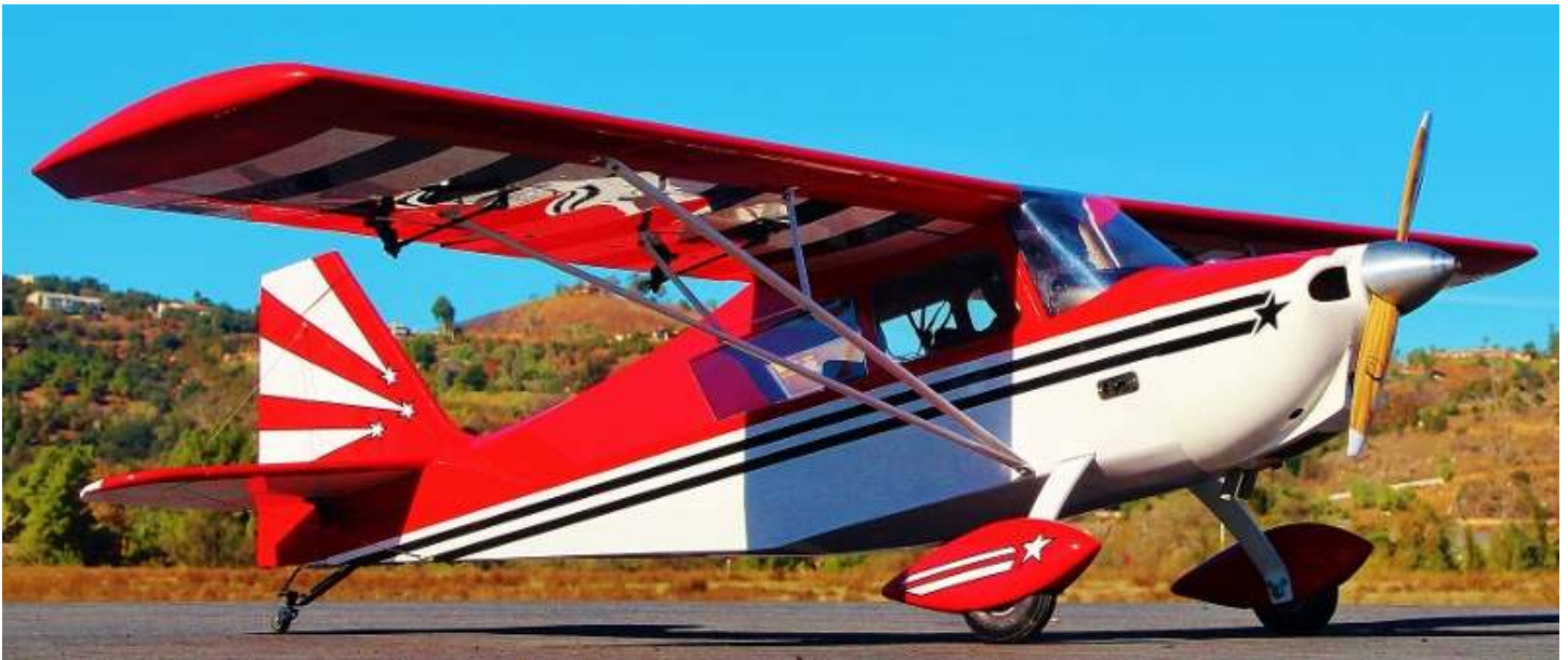
Doesn't Don's plane look full-scale? It has an 85" wingspan, is an ARF, and has a 180 Saito 4 stroke gasoline ignition engine which hauls this 15 pound beauty quickly.
