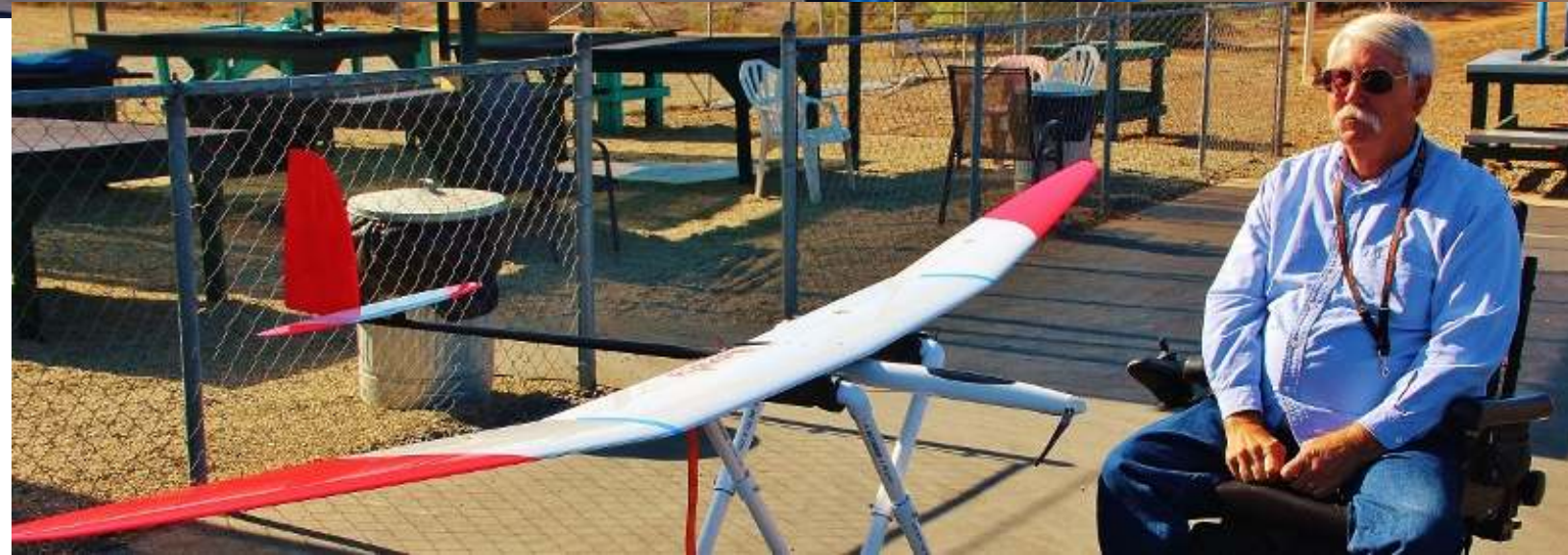
Mike Lonnecker with his plane imported by Soaring USA, perhaps from Ukraine. 150" wingspan, just over 7 oz wing loading with a NUE 1102 inrunner with 6.7 to 1 gear box swinging a 16X8 folding carbon fiber prop.
