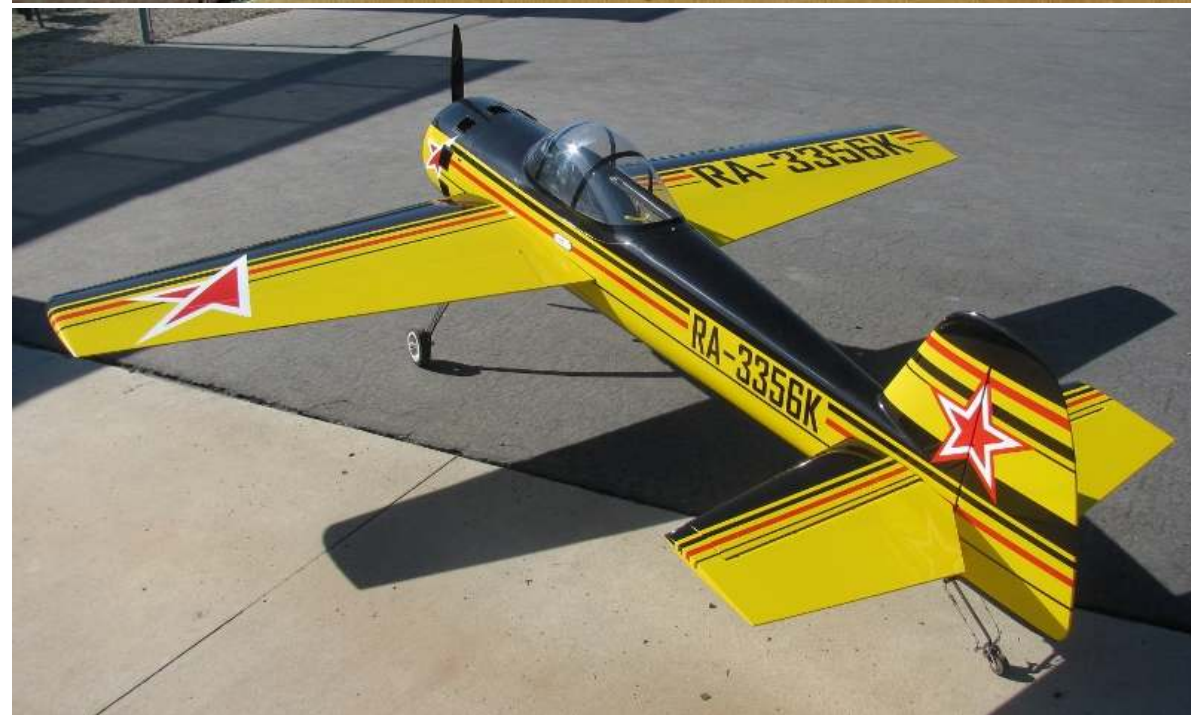
Dave Litaker has a new Yak 55M from Krill. It is composite & fiberglass construction and is painted in the mold. The wingspan is 102 in. and it weighs 26 lbs. It is powered by a DA-120 gas engine running a 28 x 12 Mejzlik carbon fiber prop and spinner. The landing gear is carbon fiber with White Rose wheels. It has Savox high voltage servos and JR--DMSS radio system 11 channels.
