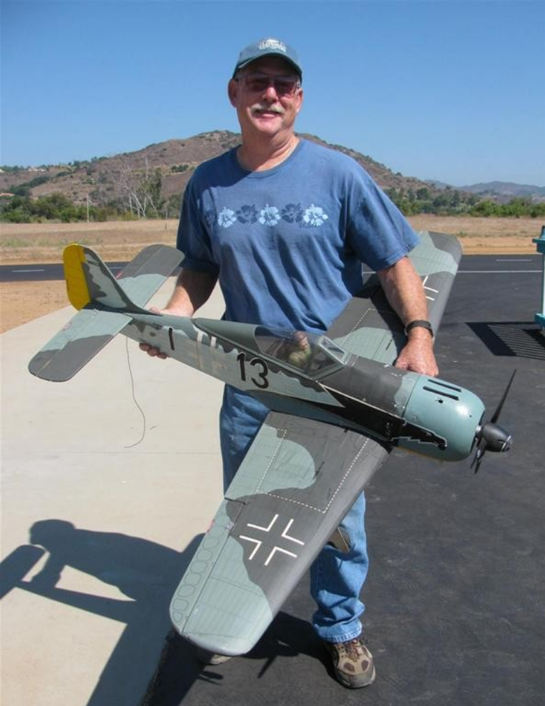
Joe Villarreal is flying this Focke Wulf FW-190 from Kyosho. It has a 57 in. wingspan and weighs 7.5 lbs. It is powered by an OS-75 two-stroke glow engine running a 13 x 8 prop.
