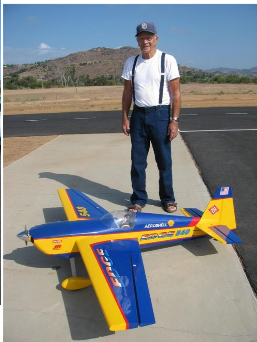
Lou Governale purchased this Edge 540 ARF from Bob Warner at the swap meet. It is powered by a Saito 180 four-stroke glow engine. The wingspan is 78 in. and it weighs 11.5 lbs.
