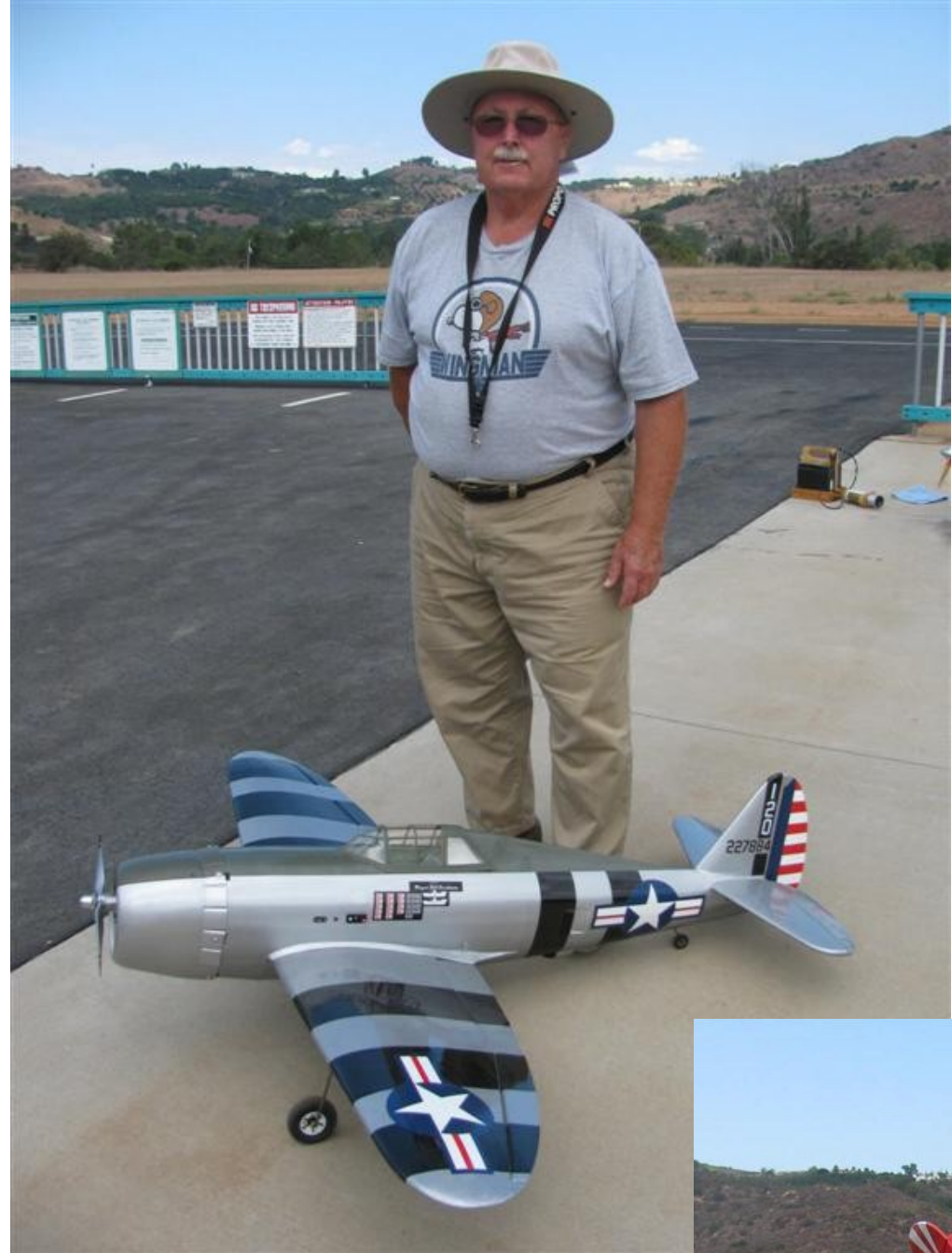
Frank Burke is flying a P-47 Thunderbolt that was built by Ed Ramsey from a TopFlite kit. It is powered by a Super Tiger 75 two-stroke glow engine with in cowl muffler system and on-board glow. It has a wingspan of 63 in. weighing 10 lbs. 12 oz. with a 35.5 oz. wing load and has Robart air retracts.
