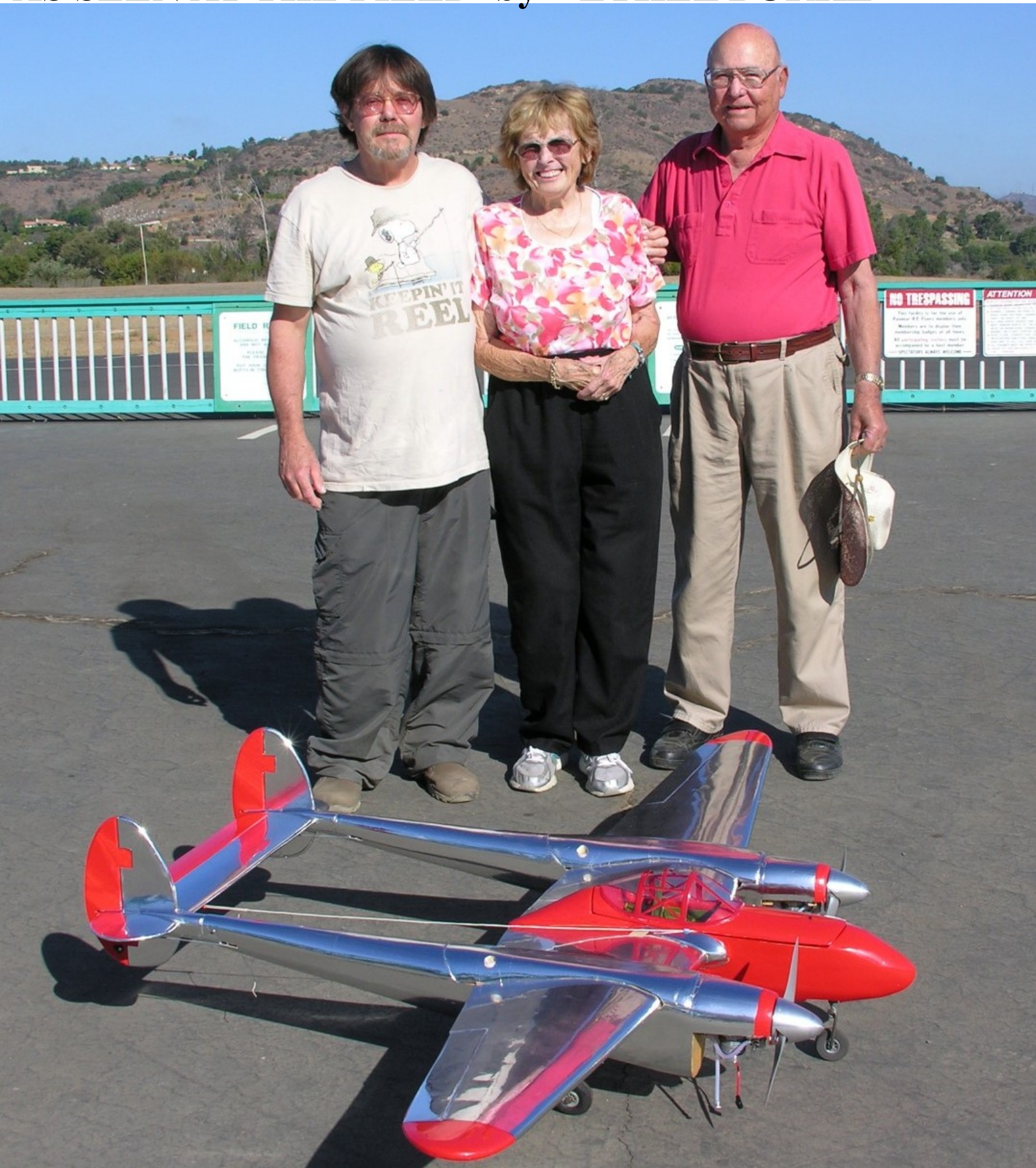
This is Charlie Wajdak (and wife, Kay) with new P-38 Lightning built by Ed Ramsey (on left) from a Royal kit. It is powered by twin OS-SF 46 two-stroke reverse rotation engines running 11 x 6 props. The wingspan is 74 ¼ in. and it weighs 10 ¾ lbs. It has on-board glow with Spring Air retracts and is covered with chrome and red UltraCote. (Ethel Burke photos on this and the next three pages)
