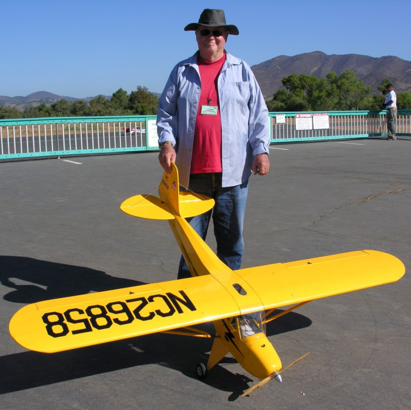
Denver Bates has a new Piper Cub J-3 ARF from World Models. It is powered by a 1 cu. in. Saito 100 glow engine running a 14 x 4 prop. The wingspan is 84 in. and it weighs 7 ½ lbs.
