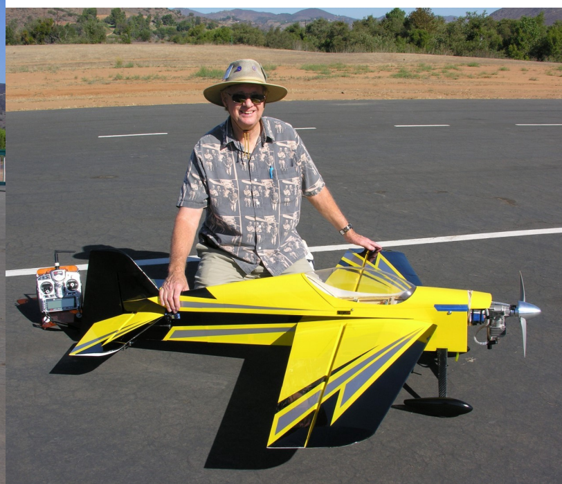
John Cutler is flying this Vyper ARF from 3D Hobby Shop. Special "Thank You" goes out to Ron Madison for the wreckage and to John Hartsell, Sr. for the loan of a DLE-20cc gas engine to try out this rebuilt frame. A new fuselage was rebuilt, wing repaired, and new canopy replaced. The wingspan is 65 in. He is running a 16 x 8 prop and it weighed in at 9 lbs. The maiden flight was successful, and this repaired Vyper is back to flying well again.
