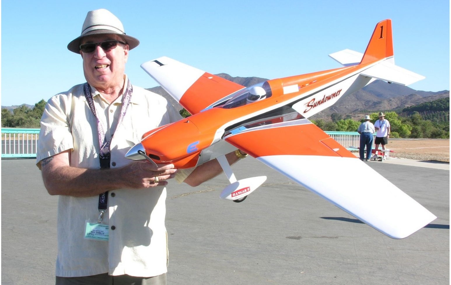
Roy DeMille is flying this new Sundowner with a 64 in. wingspan from Hangar 9. It has an E-flite Power 60 motor; an E-flite 60 amp ESC; and a 4000 mAh 14.8 volt battery.
