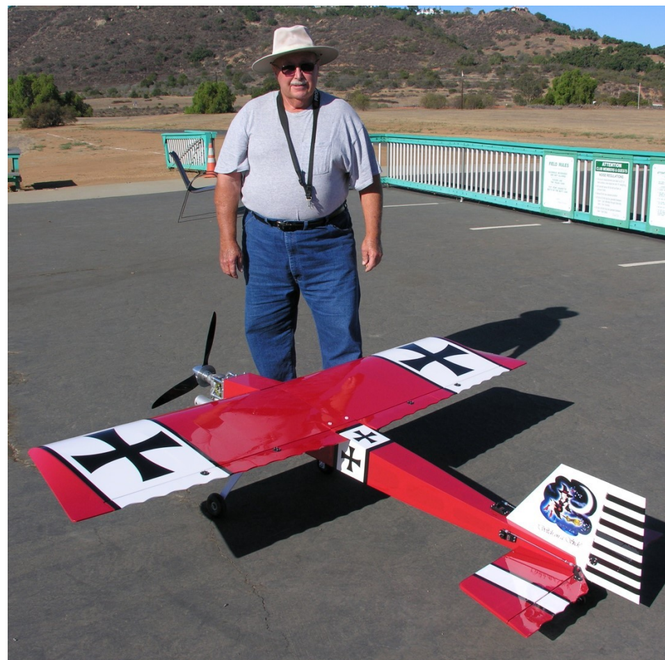
Frank Burke has a new Big Stick ARF from Great Planes. It is powered by a DLE-55cc gas engine running a 3-blade carbon fiber Biela 20 x 10 prop. It has a wingspan of 81 in. with a 22 oz. wing load, and it weighs 14 lbs. 11 oz. The tail was modified with a new straight vertical stab and rudder.
