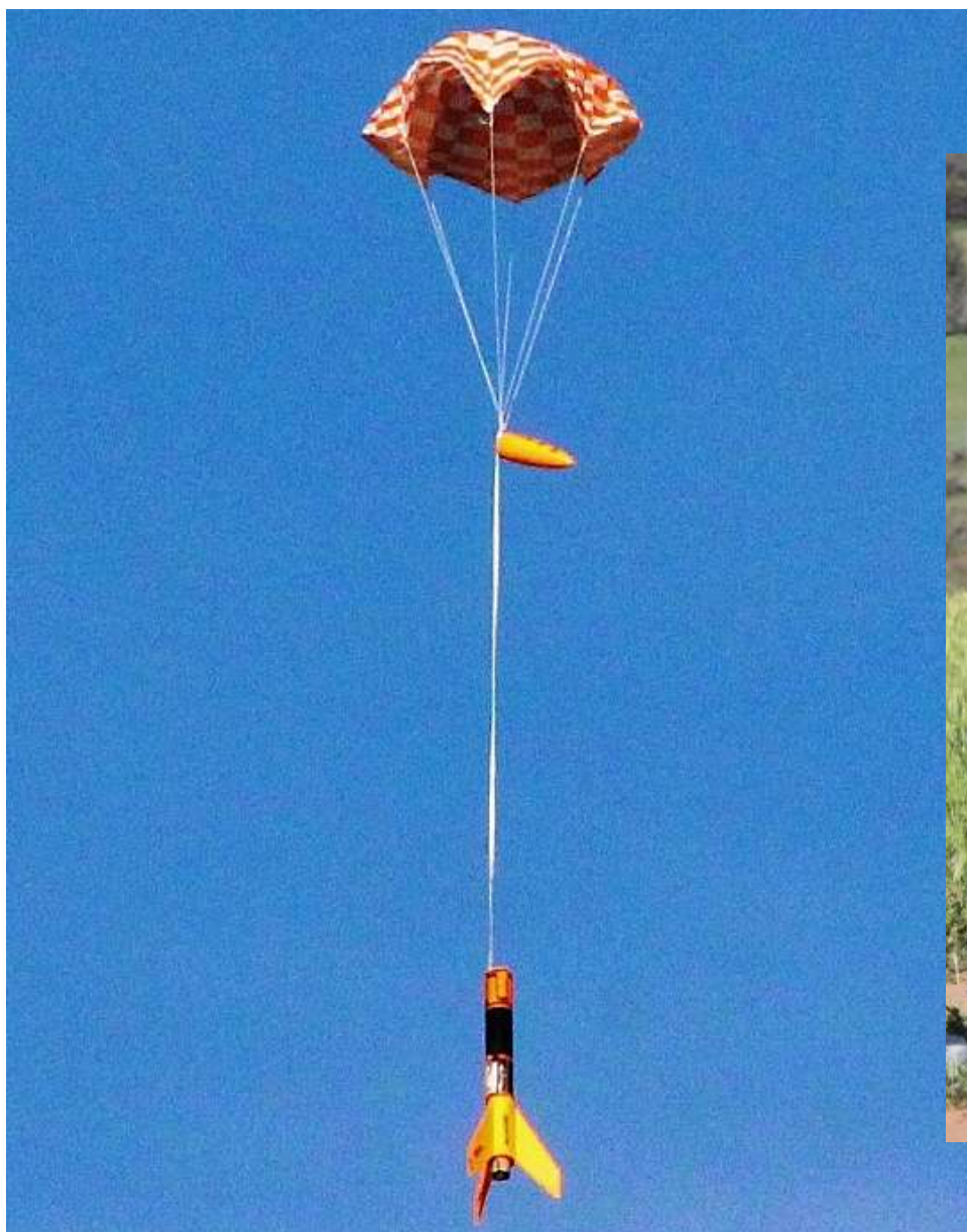
The rockets deploy a chute for a soft landing. Each launch costs about $4. for the rocket motor which can be used but once.
