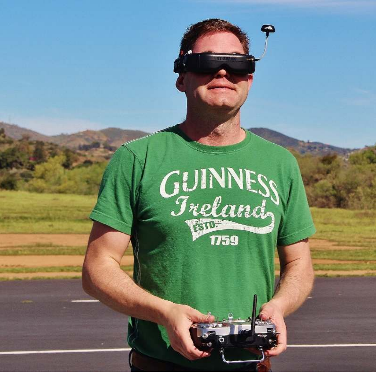
Former member Tim Wesselman has his FPV (first person view) glasses on with which he can fly his plane. The photo below shows the FPV setup.
