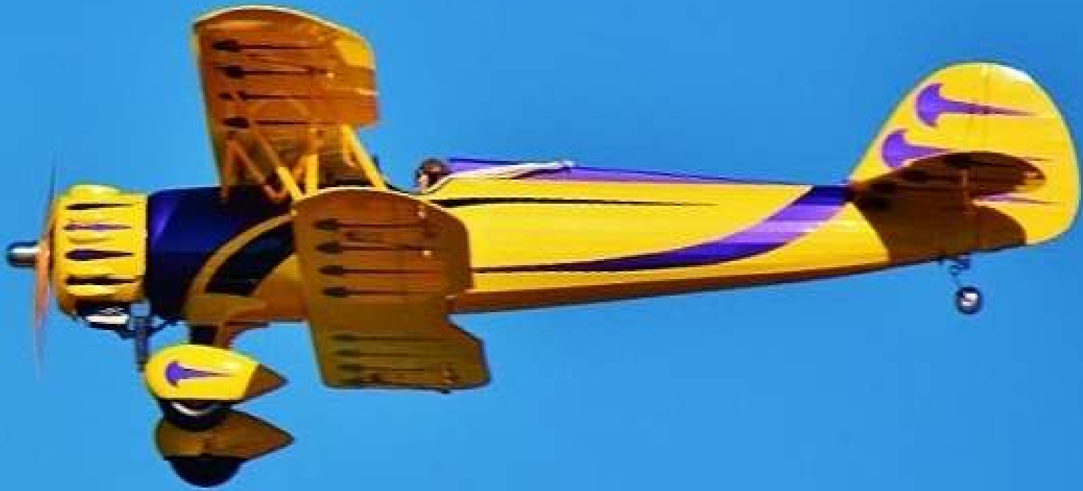
Frank Burke has built and flown this new Waco 1/5 scale biplane from a Pica kit. Got the kit from John Hartsell, Sr., and much thanks to him for the opportunity to build it. The wingspan is 72 in. and it has a 27 oz. wing loading. It is powered by a DLE-55cc rear exhaust gas engine running a 23 x 8 Xoar prop. It weighs 18 ½ lbs. (Photos courtesy of Clay Hoag)
