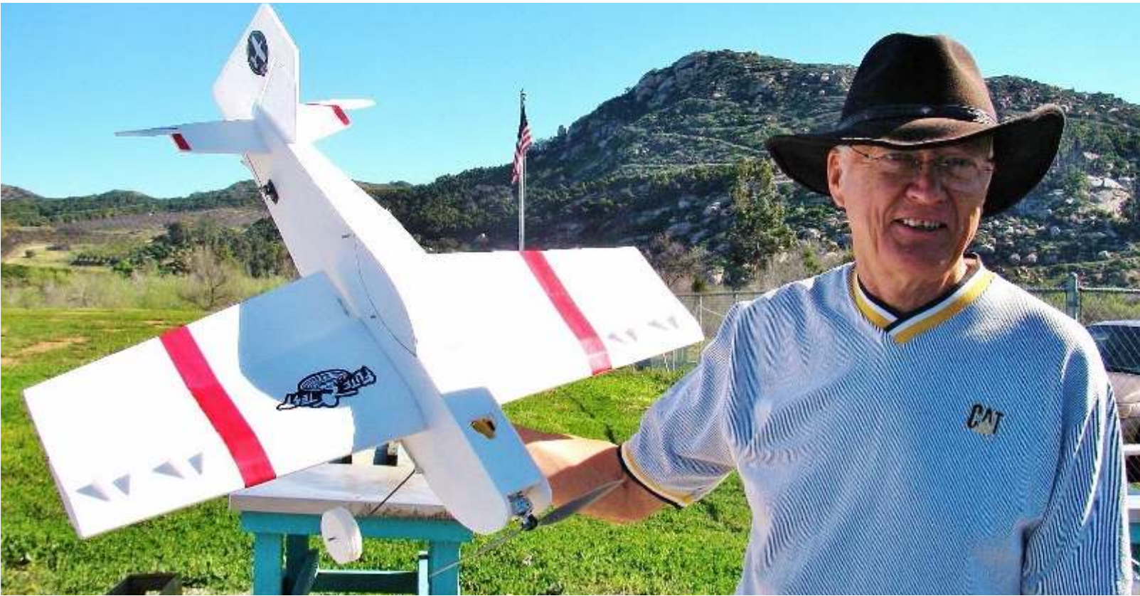
Graham Lloyd flew a new FT-3D plane from FliteTest that he found on-line @ You Tube. The air frame costs $36.00 and it is made of foam board covered with paper. He made it in an afternoon. It has an electric motor 130 watts with a 10 x 4.7 prop. The ESC is 18 amps and he is using a battery with 11.1 volts 1300 mAh.
