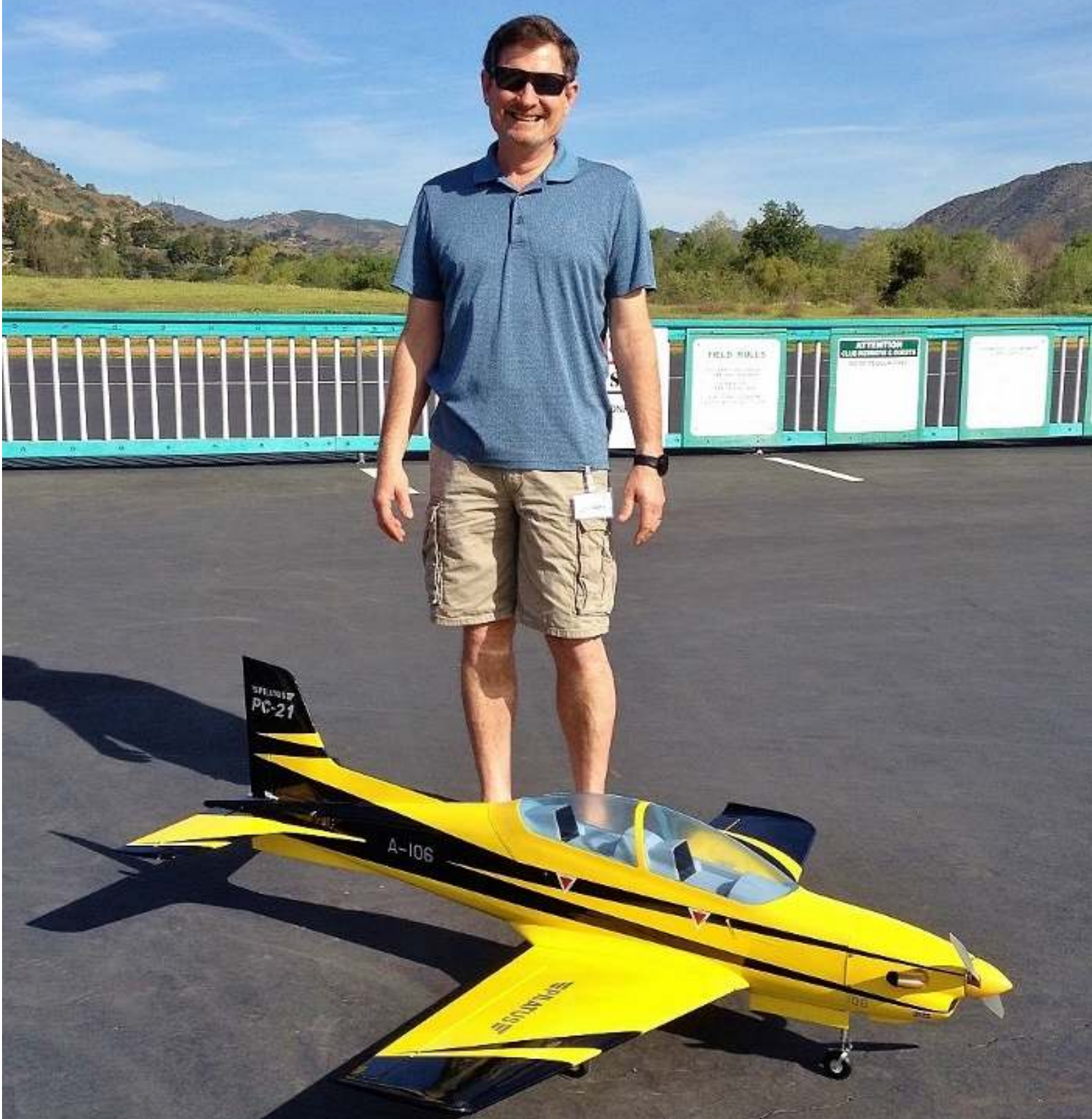
Dave Swaffer made a successful maiden flight with his new Swiss Pilatus PC-21 tri-gear ARF plane from SebArt. It has a 60 in. wingspan with a Hacker A-50 electric motor and a Hacker SB-70 ESC. It has 5S battery and all Savox servos. It is a good flying plane and is available through Chief Aircraft.
