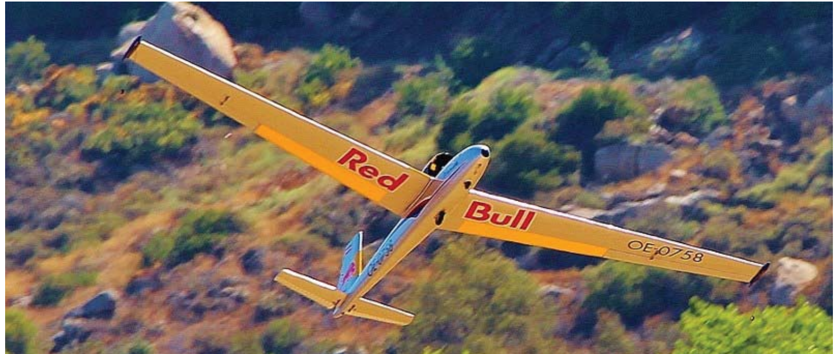
June 12, 2014 Victor Lanz prepares his Czech Blanik turbo-fan powered sailplane which weighs 28 lbs. It flies awesomely and has a 14 foot wingspan! The turbine spins at 30,000rpm!
