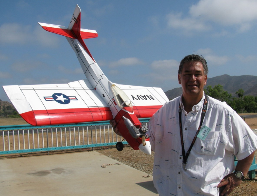
Jim Jenkins, our Club Safety Officer, is flying this Contender. It is powered by a Magnum XL-61 glow engine running a 12 x 5 prop. It has a wingspan of 48 in. and it weighs 10 lbs. Jim also flies this Sportster with a wingspan of 48 in. It is powered by a Magnum 52 two-stroke glow engine. It has retracts and weighs 10 lbs.
