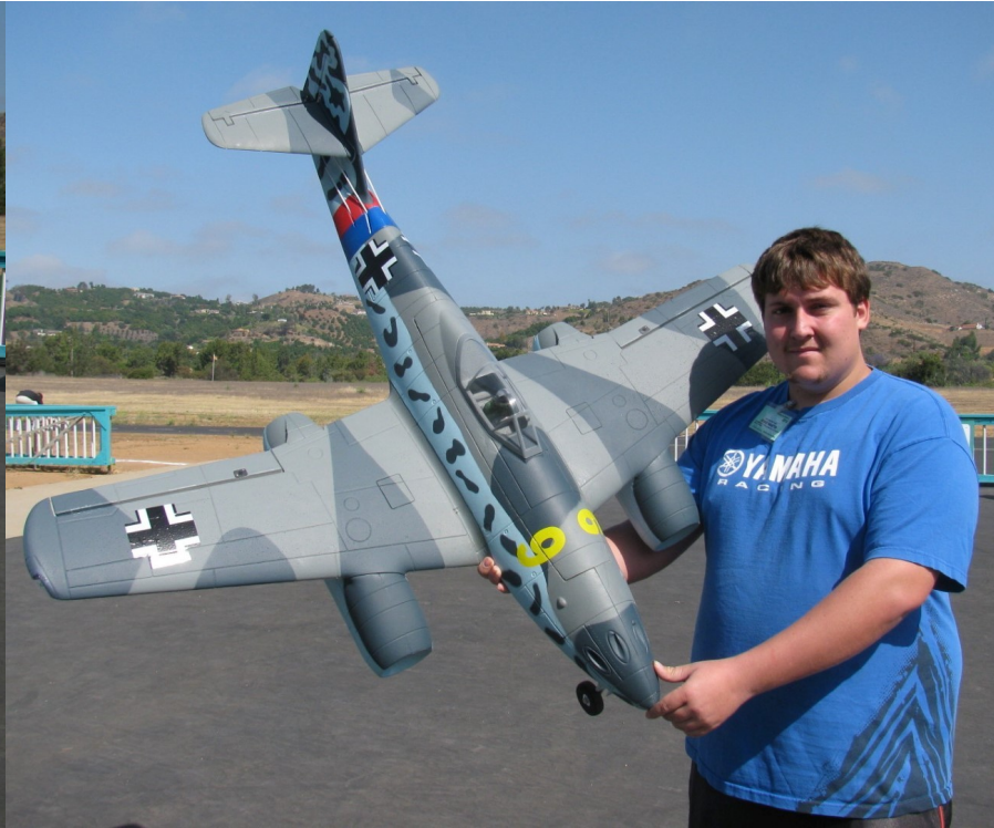
Another father & son team, Richard and Jesse Martin were out to fly. Rich has this Great Planes Reactor Biplane with a Saito 100 Golden Knight 4-stroke glow engine. Jesse is flying this ME-262 jet by Dynam. It has 2 ducted fans 70 mm electric motors with a 4000 mAh battery.
