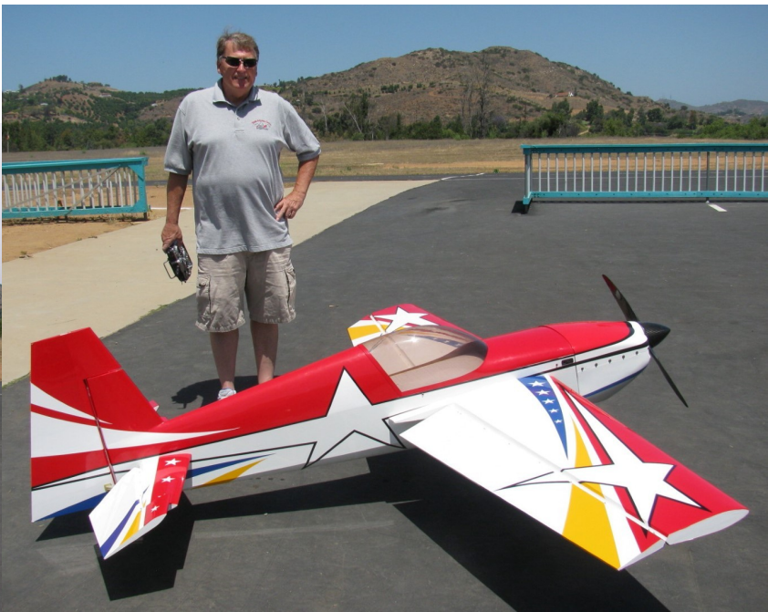
Mike Jensen is flying this A. J. Slick from 3D Hobby Shop. The wingspan is 104 in. and it weighs 27 lbs. It is powered by a DA-120cc gas engine with a 32 oz. fuel tank. It has a carbon fiber landing gear & spinner with Mejzlik 29 x 10S prop. The exhaust system is a K. & S. German canister. It has a pair of 3800 2S lipo batteries with an R922X receiver. (This plane quit flying once and fell into the jungle, was found, luckily in this great condition. We don't lose all of them folks.)
