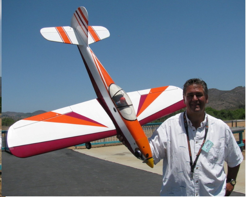
Jim Jenkins, our Club Safety Officer, is flying this Contender. It is powered by a Magnum XL-61 glow engine running a 12 x 5 prop. It has a wingspan of 48 in. and it weighs 10 lbs. Jim also flies this Sportster with a wingspan of 48 in. It is powered by a Magnum 52 two-stroke glow engine. It has retracts and weighs 10 lbs.
