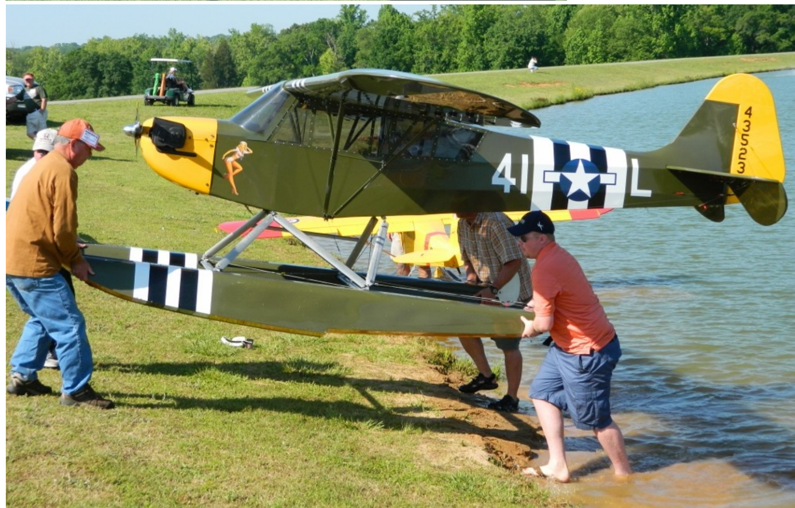
This is a 60% size Cub built from a Bill Hempel kit. Price 13 of kit is $3,200 and Bill's website is: Billhempel.com This model weighs 120 pounds and has 16 to 20 servos. For example, one aileron alone has four servos, each @ 400 inch ounces of throw. When this plane flies, most other activity stops to watch this most scale-like plane perform. The rudder stands 50" above ground.
