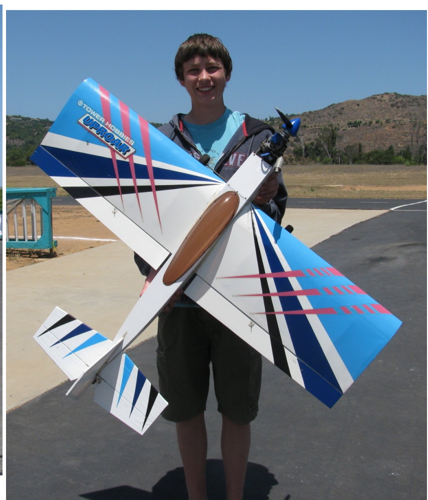
" Welcome " to new member, John Buckley. John is a student pilot close to earning his flight certificate. He is flying this Uproar 40 from Tower Hobbies. The wingspan is 48 in. and it weighs about 4 lbs. It is powered by a Magnum XL-52 four-stroke glow engine running a Master Aircrew 12 x 6 prop.
