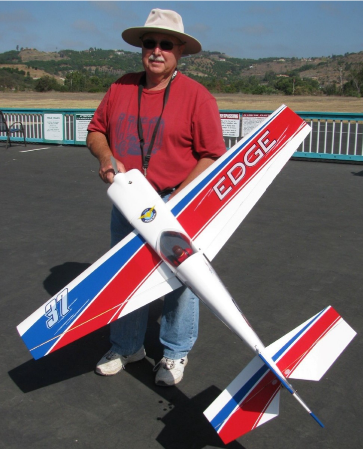
Frank Burke has a new Edge 540 from Phoenix Models with a 56 in. wingspan. It has a Tower Hobbies 46 two-stroke glow engine with an 11 x 6 prop, and weighs 6 lb. 1 oz.
