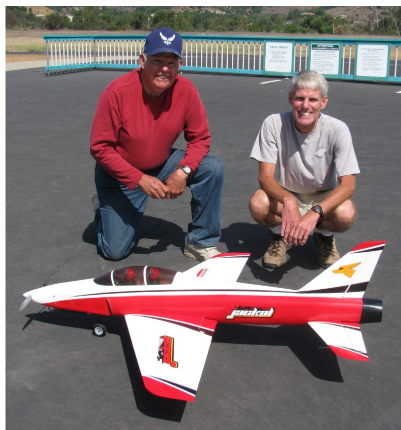
Here we have John Hartsell, Sr., builder and John, Jr., pilot with their new Jackal 50 prop jet from Hangar 9. It has a wingspan of 54 in. with flaps. It is powered by an Evolution 10cc gas engine running a 10 x 7 prop. It has Robart tricycle landing gear and weighs 8 lbs. 8 oz.
