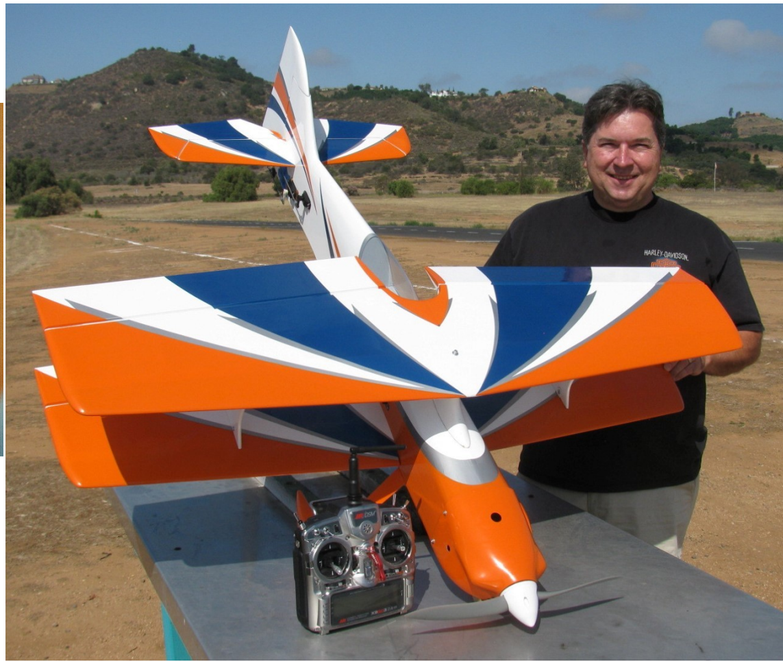
Frank Burke has a new Edge 540 from Phoenix Models with a 56 in. wingspan. It has a Tower Hobbies 46 two-stroke glow engine with an 11 x 6 prop, and weighs 6 lb. 1 oz.
