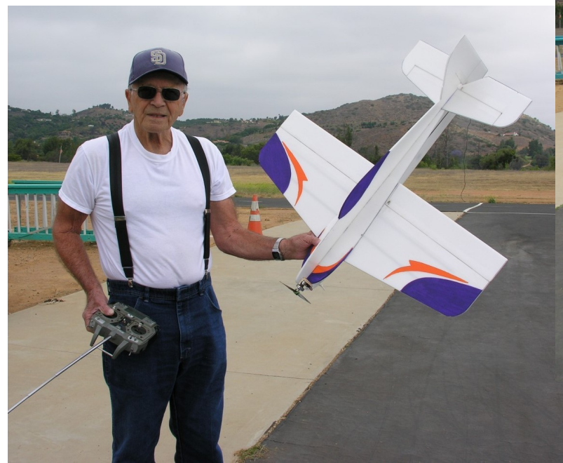
Lou Governale has created his own Depron foam 3-D plane. It has an electric motor; 15 amp ESC; E-flite 1000 mAh 20c battery; with 6 in. prop and Hitec 5-channel receiver & Hitec servos. Carbon fiber spars are used for reinforcement, and he used water base craft shop paint for color design. It flies well.
