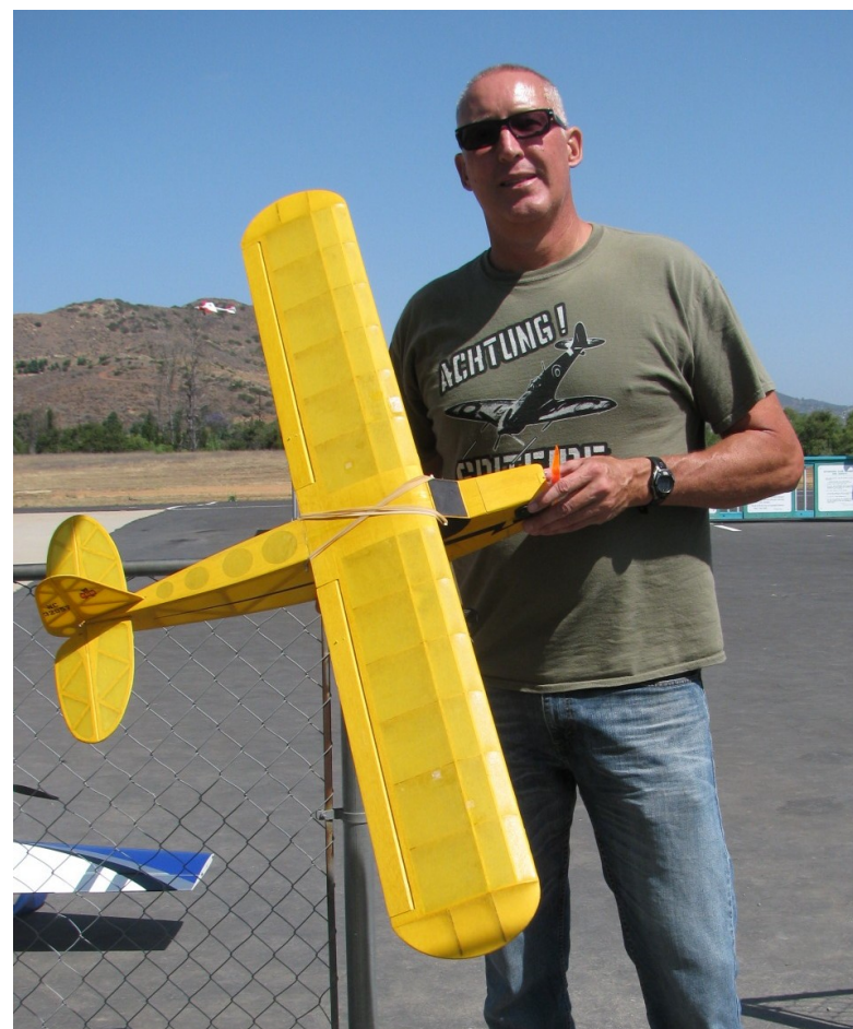
John Grimm has built a bunch of unique electric planes packed in the back of his SUV. This one is a Piper Cub from House of Balsa. It has a wingspan of 42 in. and is covered with tissue. He is running an electric 400 size motor with an 8 x 4 prop. His wife, Ann, came along to watch--riding in on her Harley-Davidson Sportster. John rides a Harley-Davidson Blackline soft tail.
