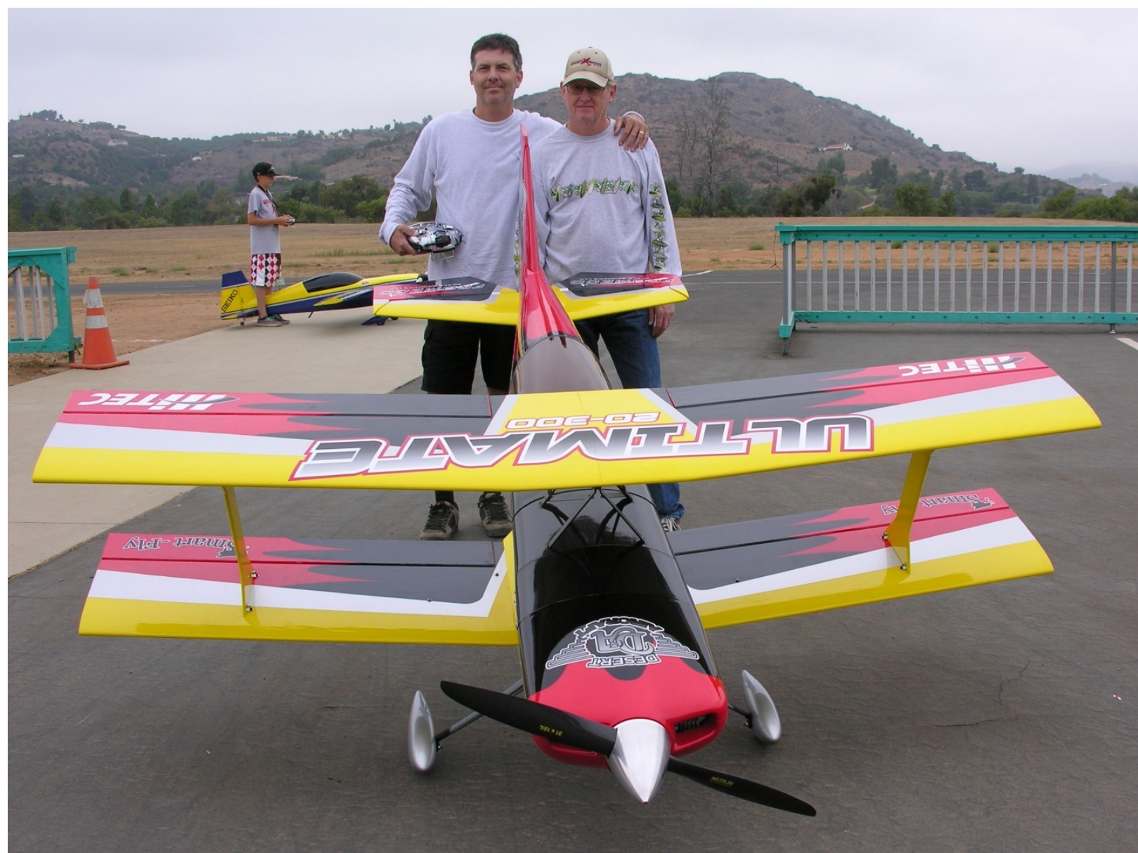
This is a 42% Ultimate Bipe 20-300 from Aeroworks. It is powered by a DA-170cc twin cylinder gas engine with a Mejzlik 31 x 12 EVO L carbon fiber prop. It is fitted with MTW RE3 tune pipes, all Hitec digital servos, Fromeco switches and batteries, carbon fiber landing gear with White Rose main wheels and tail wheel, SMJ custom ultra spinner and B & E Graphix. It was assembled by Dave Litaker and is flown by both he and James D'Eliseo. You can compare the size next to Clay Hoag's Ultimate.
