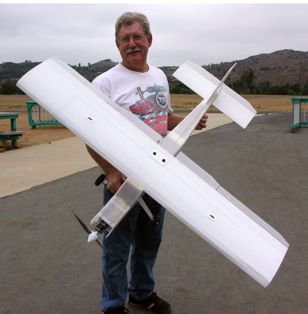
Joe Villarreal prepares for night flying event with a maiden flight on his coroplast trainer. He is using a Turnigy G-32 electric motor with a 14 x 10E prop; 4S 2200 mAh battery; 55 amp Turnigy ESC. He has a total of 300 LED lights inside the wing and fuselage.
