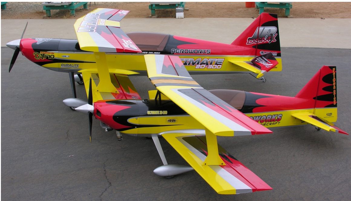
This is a 42% Ultimate Bipe 20-300 from Aeroworks. It is powered by a DA-170cc twin cylinder gas engine with a Mejzlik 31 x 12 EVO L carbon fiber prop. It is fitted with MTW RE3 tune pipes, all Hitec digital servos, Fromeco switches and batteries, carbon fiber landing gear with White Rose main wheels and tail wheel, SMJ custom ultra spinner and B & E Graphix. It was assembled by Dave Litaker and is flown by both he and James D'Eliseo. You can compare the size next to Clay Hoag's Ultimate.
