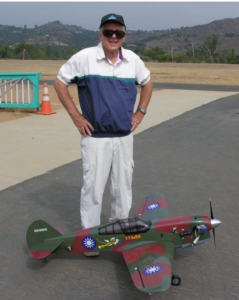
Bill Demore has a new P-40E Warhawk ARF from CMP. It is powered by a Magnum 91 four-stroke glow engine. The wingspan is 65 in. and it has Robart air retracts. Bill also is flying this new 60 size Ultra Stick. It is powered by a Thunder Tiger 61 two-stroke glow engine. The wingspan is 60 in.
