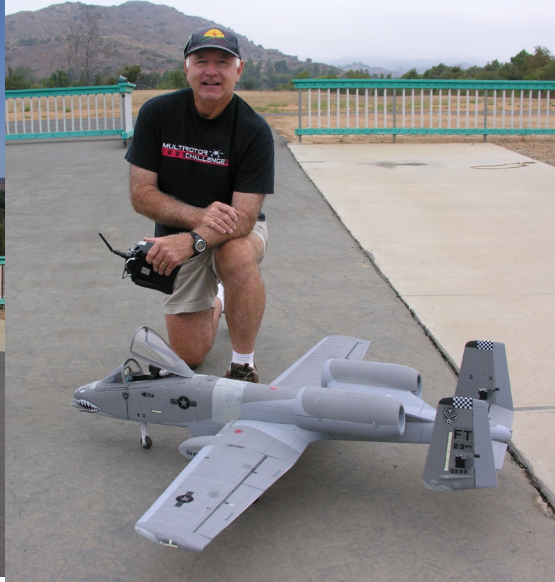
Butch Weiser, guest flyer visiting from the Weedwackers Club, flew his A-10 Warthog from Toysonics Hobby Shop. It has a 59 in. wingspan with 70mm twin ducted fan electric motors. It has two 60 amp ESC's and 6S--45C battery 3300 mAh (needs more power). It has an operational canopy and exterior running lights.
