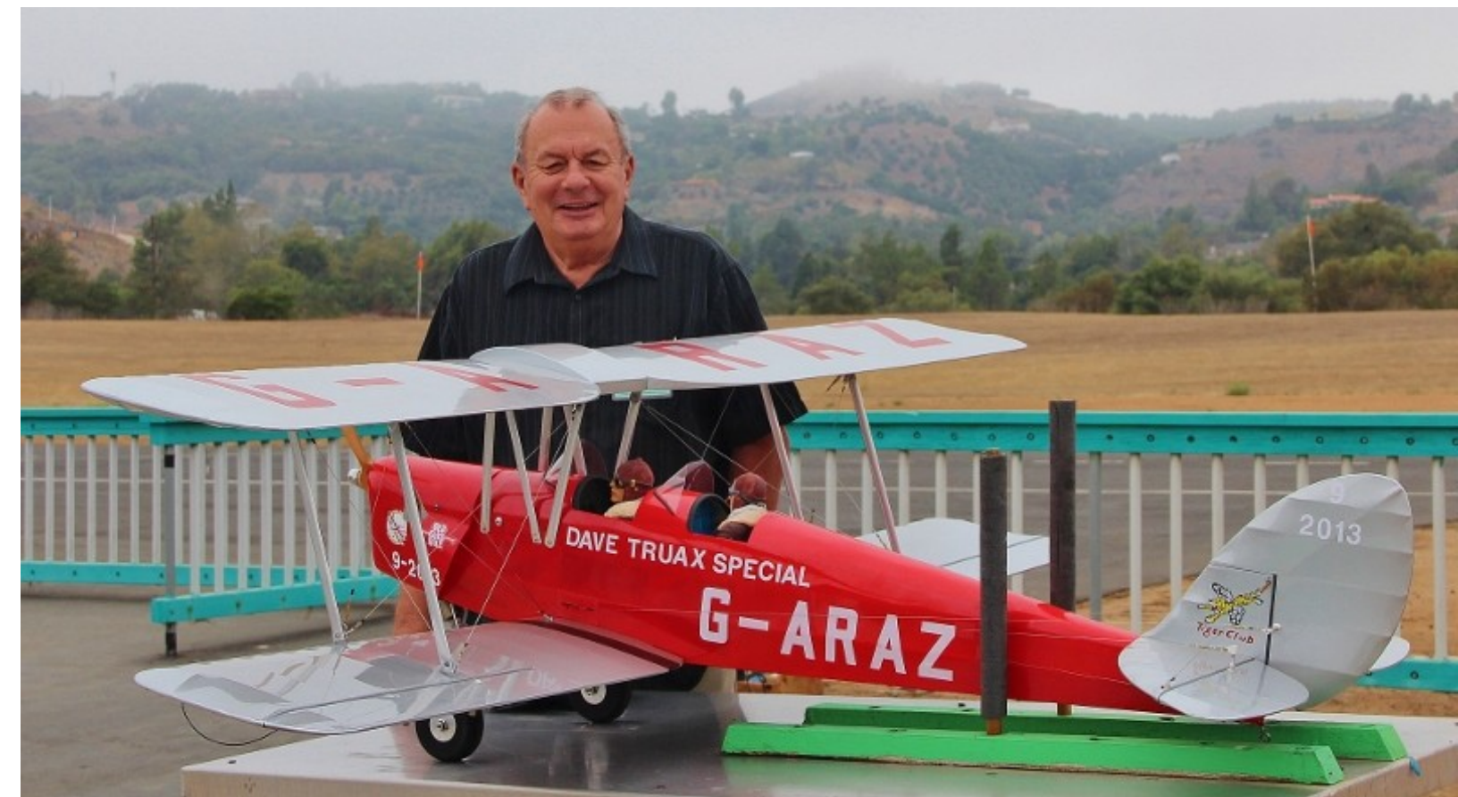
Dave Truax came to the field on Sept. 17th to watch the maiden flight which went beautifully. It flew well because James D'Eliseo was the pilot. This won Model-of-the Month for September. The front student pilot is a woman. The Vane airspeed indicator on the left strut adds a nice touch. Removable wingtip skids, a shock-absorbing landing gear, tail-bracing, turnbuckles, lettering etc. are my additions. It weighs 11.8 lbs. and has 13 sq. feet of wing area giving it a 14.5 ounce per sq. ft. It floats and is a delight to fly. 14 This plane belongs to Joe Buko, your editor.
