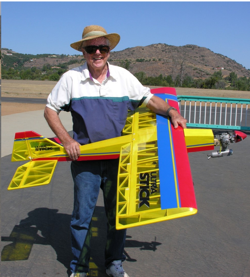
Bill Demore has a new P-40E Warhawk ARF from CMP. It is powered by a Magnum 91 four-stroke glow engine. The wingspan is 65 in. and it has Robart air retracts. Bill also is flying this new 60 size Ultra Stick. It is powered by a Thunder Tiger 61 two-stroke glow engine. The wingspan is 60 in.
