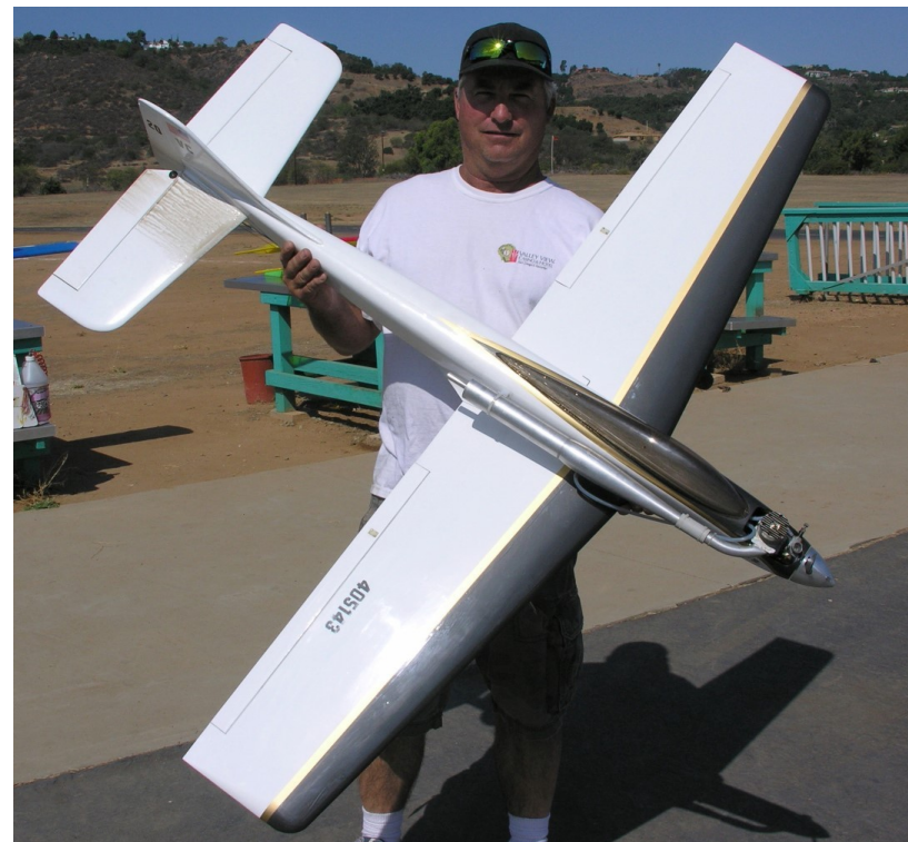
Scott Holmes has built this "Dirty Birdie" from a Blue Jay kit. It is powered by an OS-61-FSR two-stroke engine with a tune pipe. It has a 64 in. wingspan and mechanical retracts.
