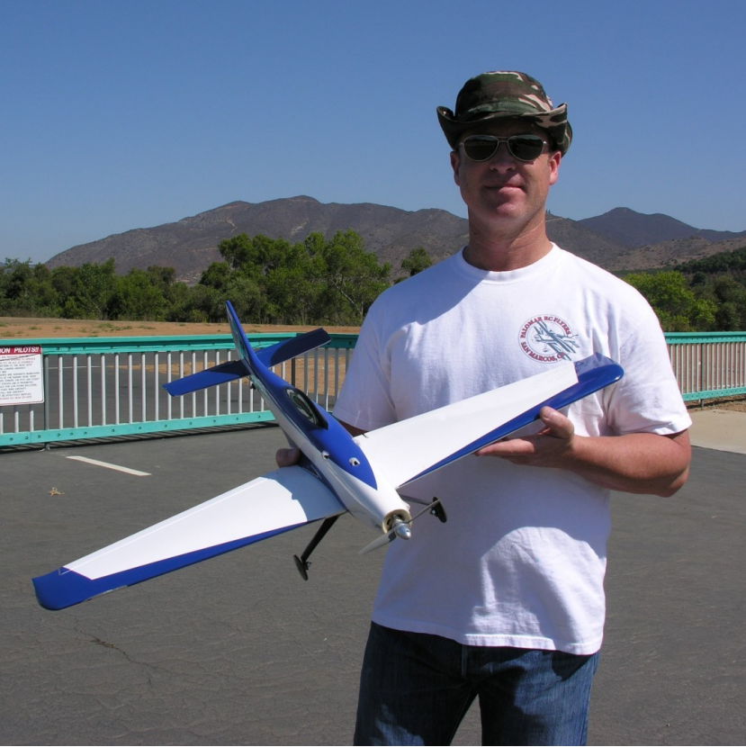
Gary Kaplan has a new Pylon Racer from Hobby King. It has a 3300 kv Typhoon inrunner electric motor-140 amps-2400 watts-22,000 RPM. It has a Castle Creations Phoenix Edge 150 ESC, 4S battery, and a 475 x 5.5 APC prop. (Speed may be 180+). Modified landing gear and tail wheel are also used. He has added several air scoops to cool motor.
